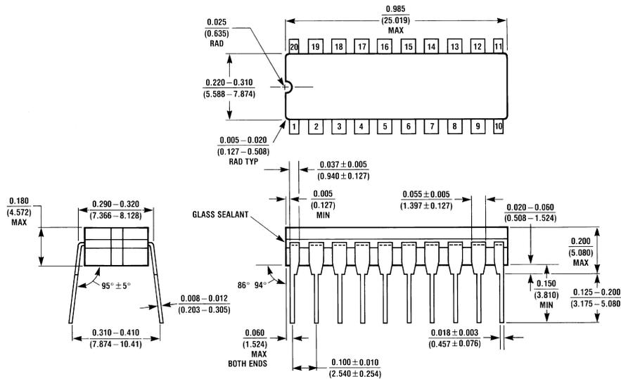
**Cavity Dual-In-Line Package (J) (Side Brazed)**
