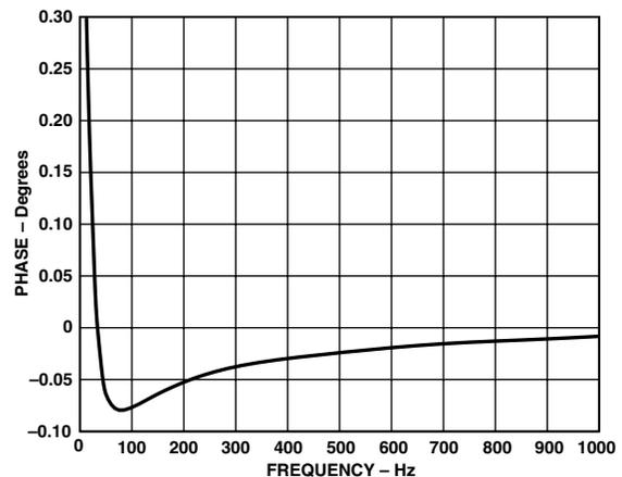
Figure 10. Phase Error Between Channels (0 Hz to 1 kHz)
