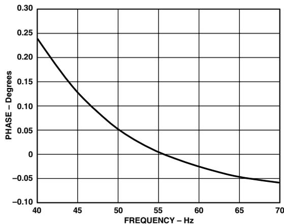
Figure 11. Phase Error Between Channels (40 Hz to 70 Hz)
