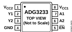
Figure 6. 8-Lead MSOP Package (RM-8)
