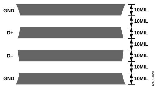
Figure 20. Arrangement of Signal Tracks
