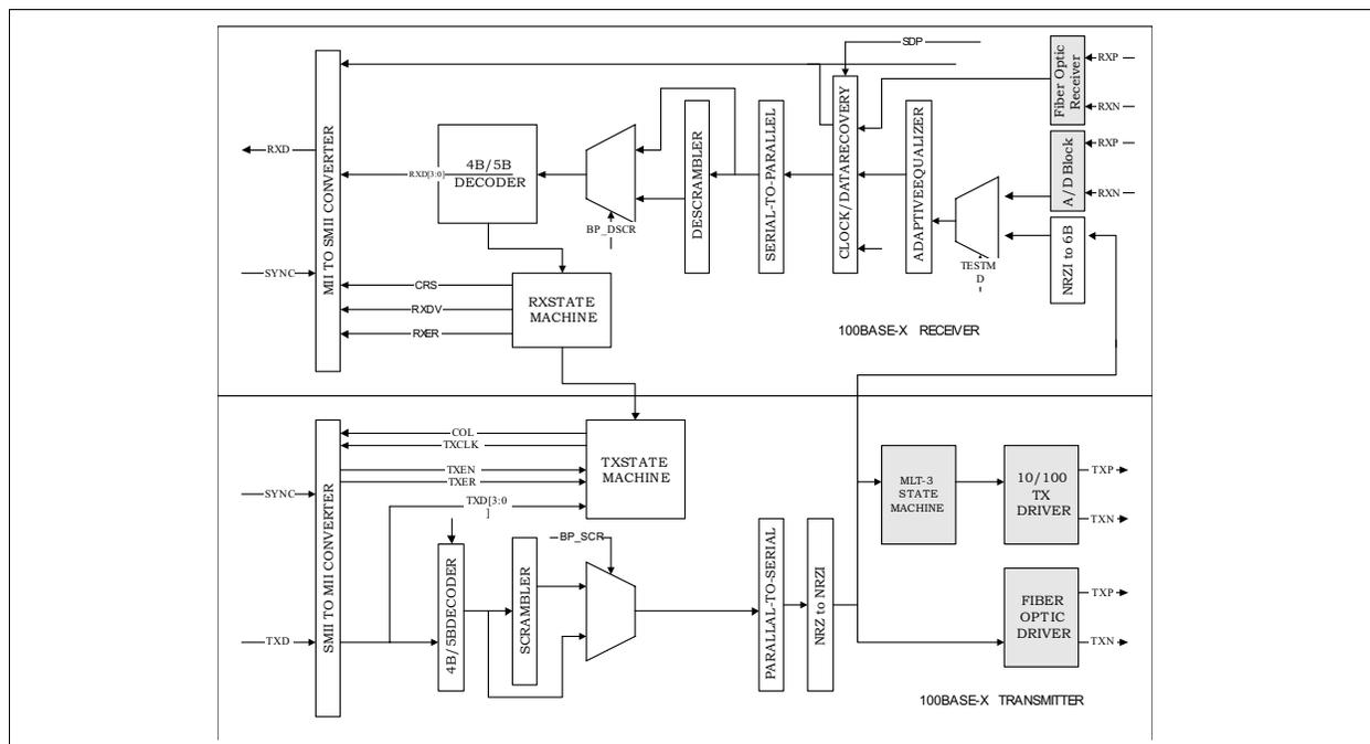
**Figure 3 100Base-X Block Diagram and Data Path**
