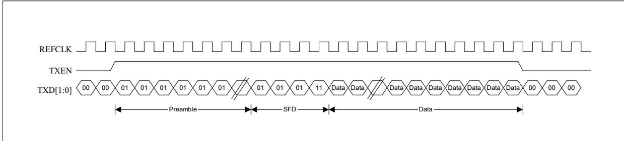
**Figure 10 100M RMIIT Transmit Diagram**
