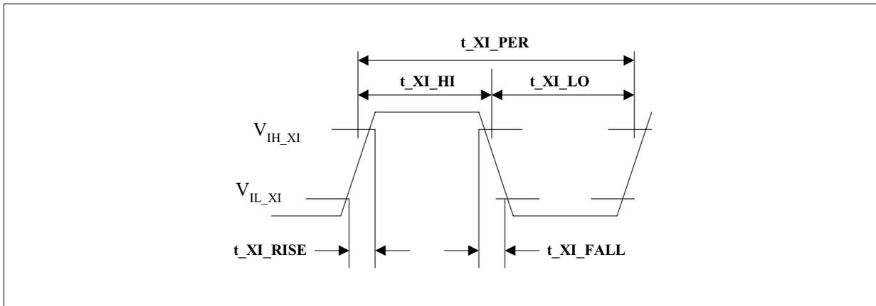
Figure 25 Crystal/Oscillator Timing
