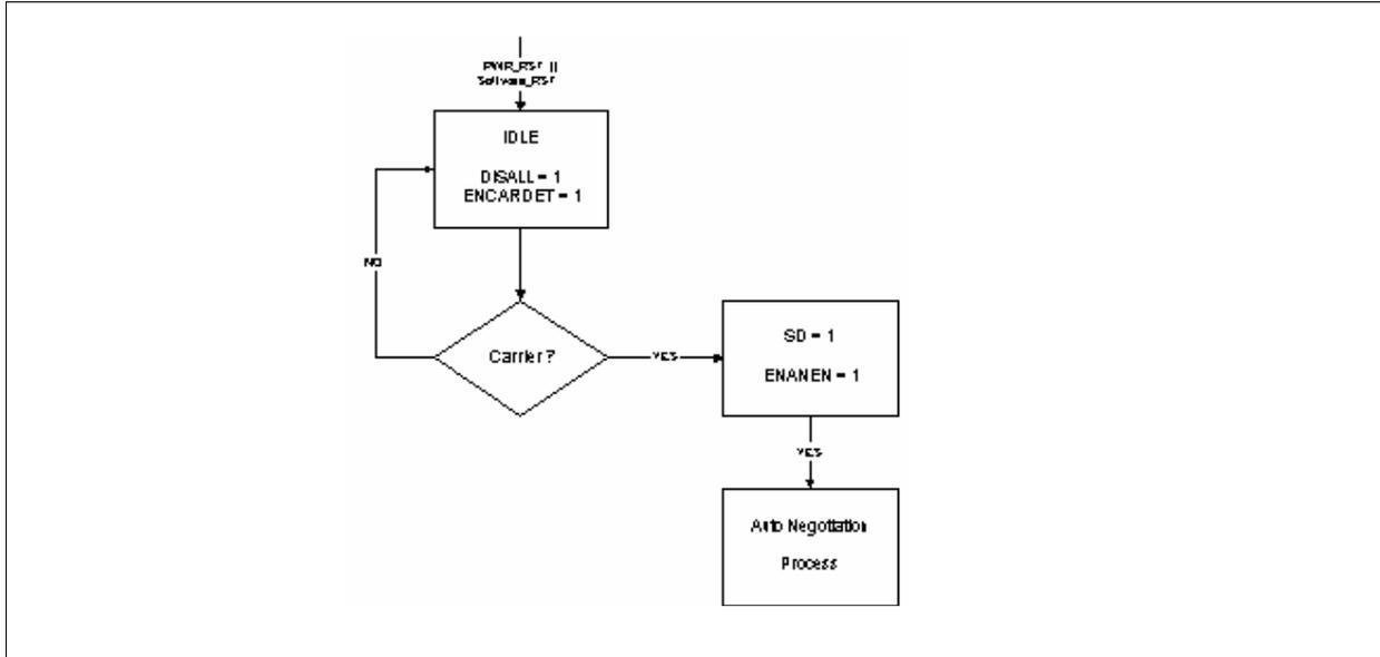
**Figure 23 Medium Detect Power Management Flow Chart**
