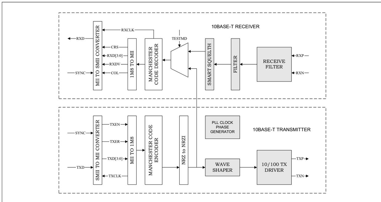
**Figure 4 10Base-T Block Diagram and Data Path**
