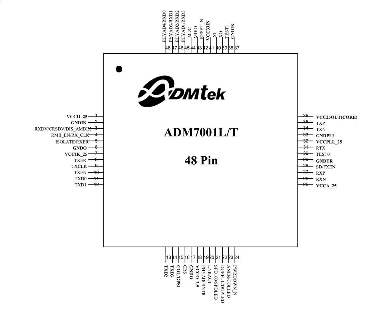
**Figure 2 Pin Diagram**
