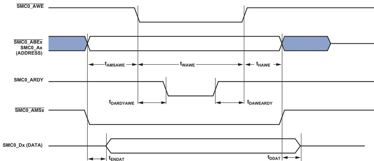
Figure 15. Asynchronous Write
