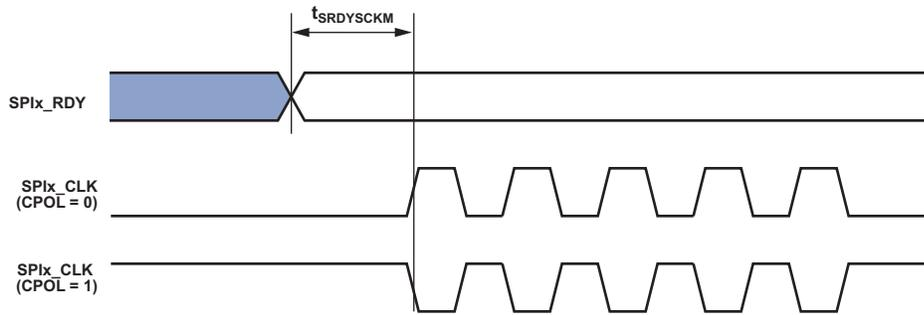
Figure 51. SPIx\_CLK Switching Diagram after SPIx\_RDY Assertion, CPHA = x
