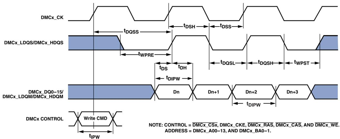
Figure 22. Mobile DDR SDRAM Controller Output AC Timing
