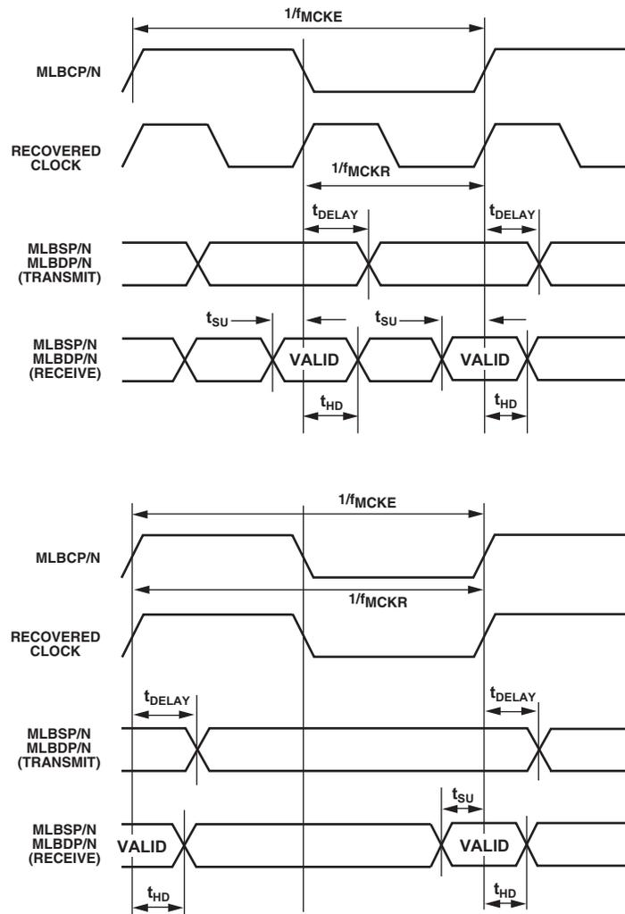
Figure 74. Media Local Bus 6-Pin Delay, Setup, and Hold Times
