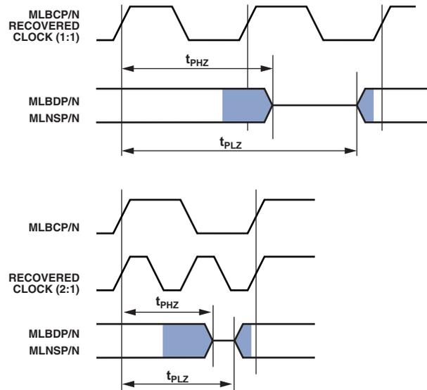
Figure 75. Media Local Bus 6-Pin Disable and Enable Turnaround Times
