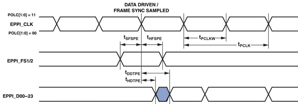
Figure 34. PPI External Clock GP Transmit Mode with External Frame Sync Timing
