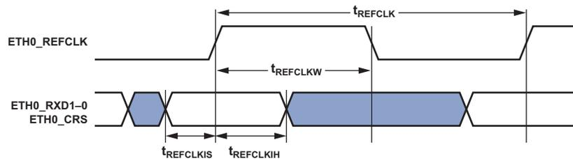
Figure 61. 10/100 Ethernet MAC Controller Timing: RMII Receive Signal
