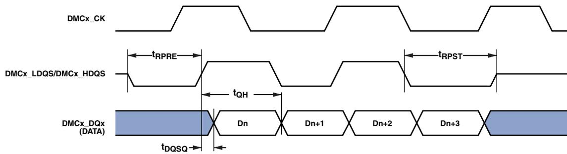
Figure 21. Mobile DDR SDRAM Controller Input AC Timing
