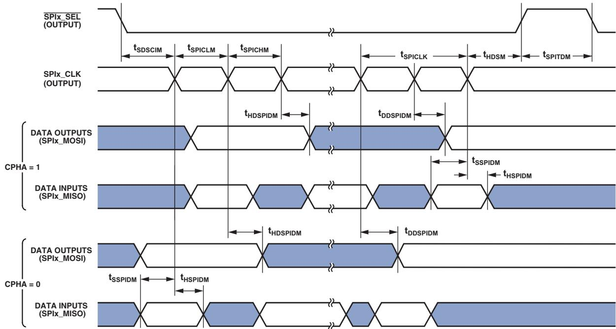
Figure 43. Serial Peripheral Interface (SPI) Port—Master Timing
