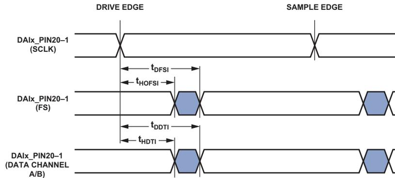
Figure 70. S/PDIF Receiver Internal Digital PLL Mode Timing
