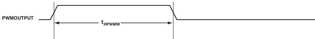
Figure 58. PWM Heightened-Precision Mode Timing, Output Pulse
