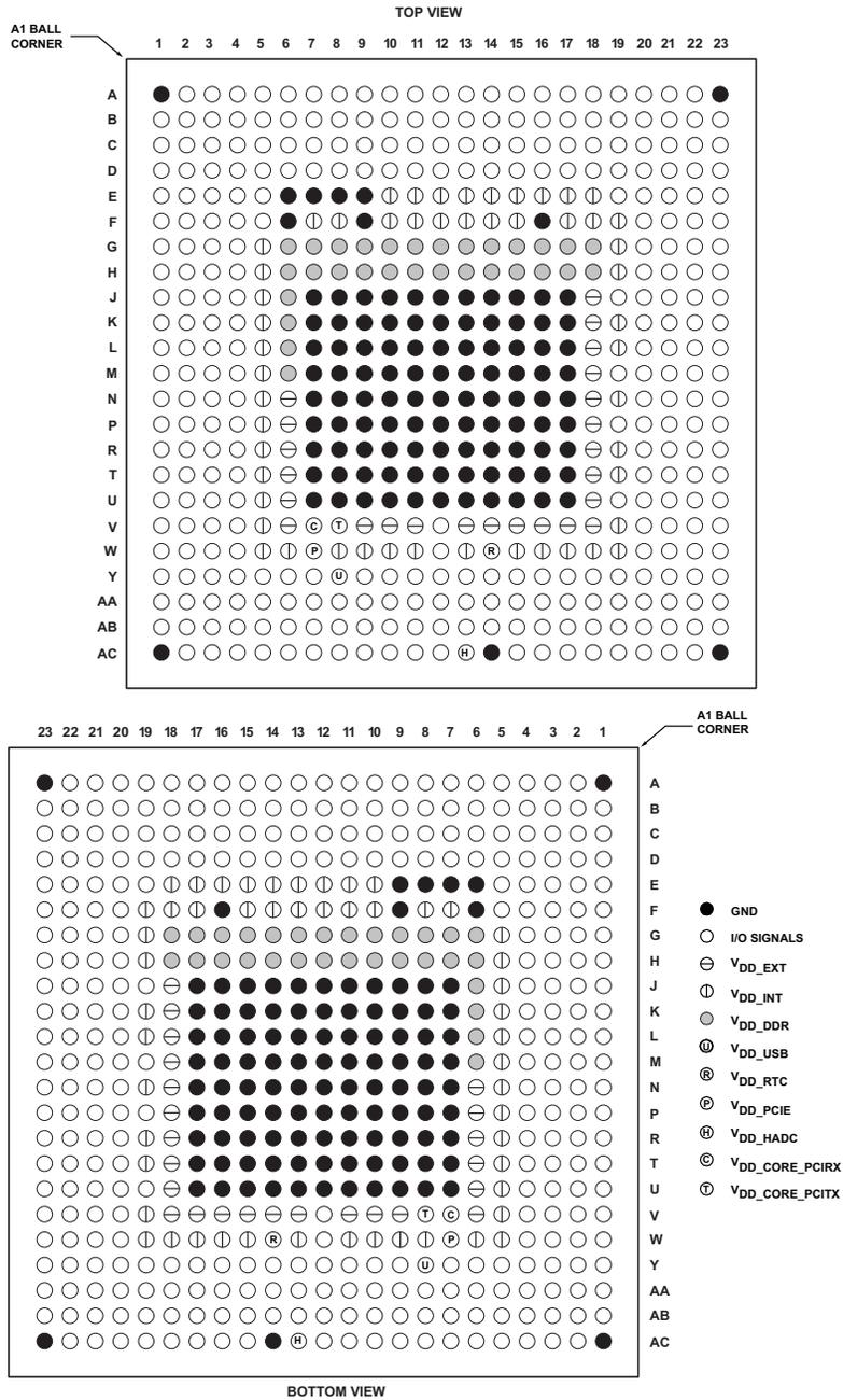
Figure 80. 529-Ball CSP\_BGA Configuration
