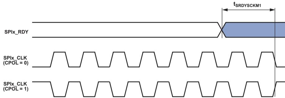
Figure 50. SPIx\_RDY Setup Before SPIx\_CLK with CPHA = 1
