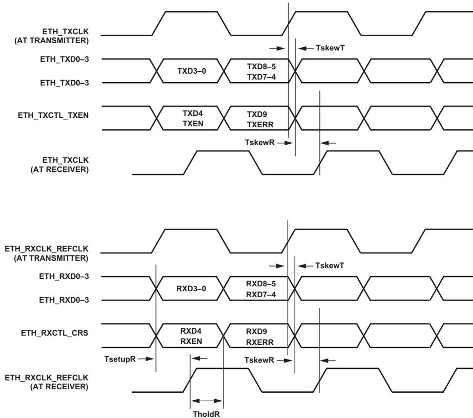
Figure 64. Gigabit Ethernet MAC Controller Timing: RGMII
