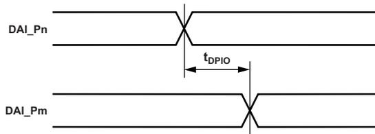
Figure 55. DAI Pin to Pin Direct Routing
