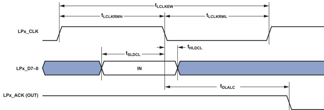
Figure 35. Link Ports—Receive
