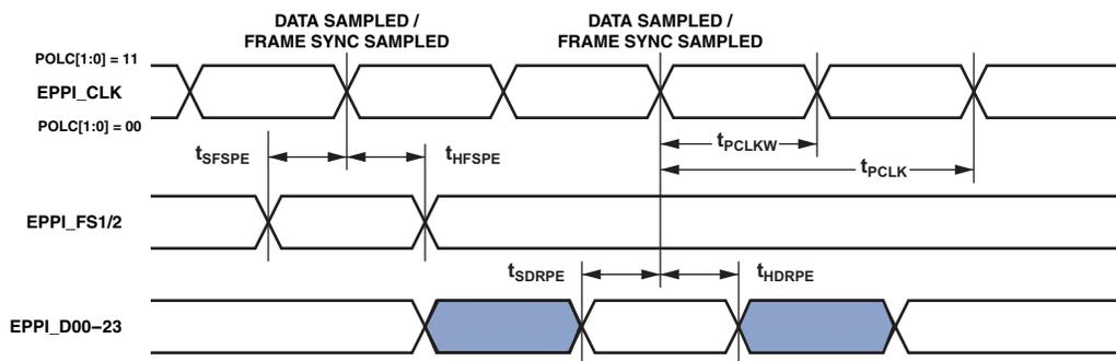
Figure 33. PPI External Clock GP Receive Mode with External Frame Sync Timing
