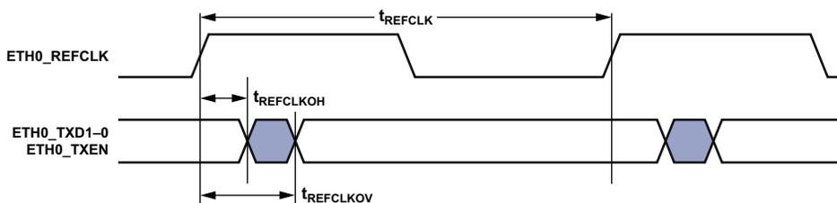
Figure 62. 10/100 Ethernet MAC Controller Timing: RMII Transmit Signal
