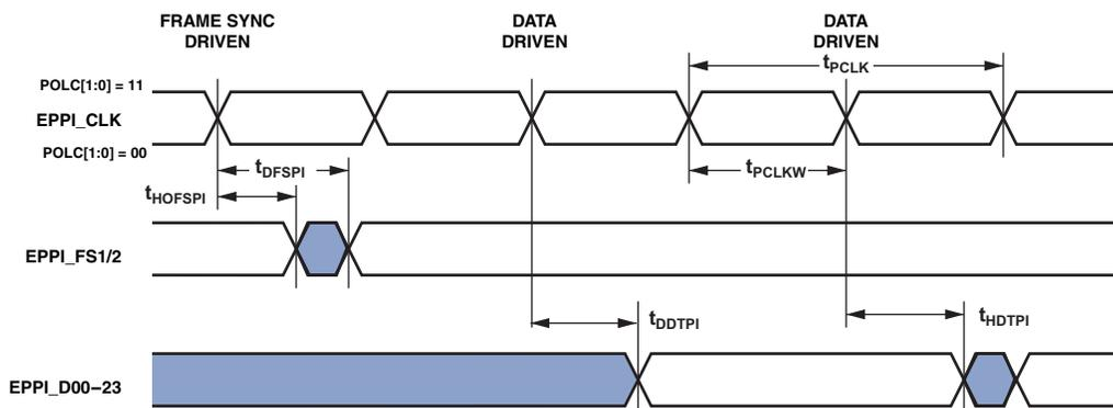
Figure 27. PPI Internal Clock GP Transmit Mode with Internal Frame Sync Timing
