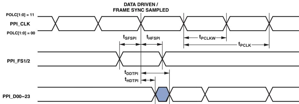
Figure 29. PPI Internal Clock GP Transmit Mode with External Frame Sync Timing
