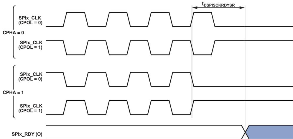
Figure 45. SPIx\_RDY Deassertion from Valid Input SPIx\_CLK Edge in Slave Mode Receive (FCCH = 0)
