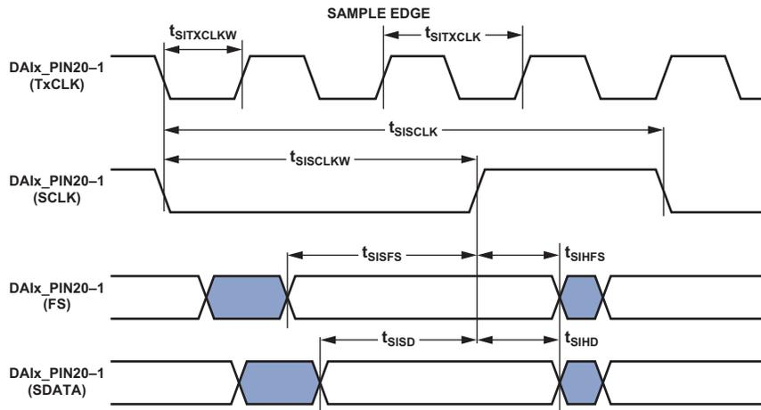
Figure 69. S/PDIF Transmitter Input Timing
