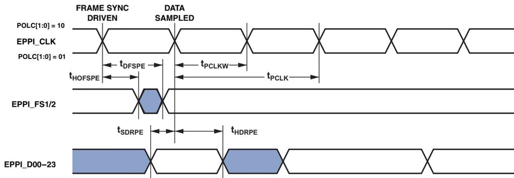
Figure 31. PPI External Clock GP Receive Mode with Internal Frame Sync Timing
