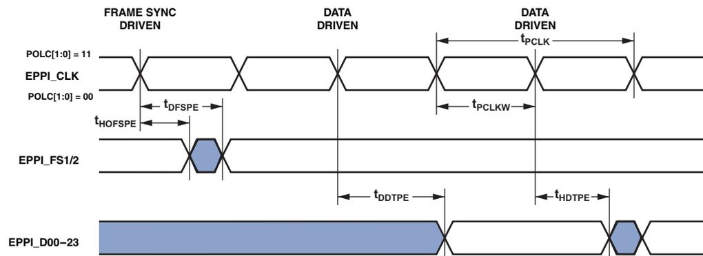
Figure 32. PPI External Clock GP Transmit Mode with Internal Frame Sync Timing
