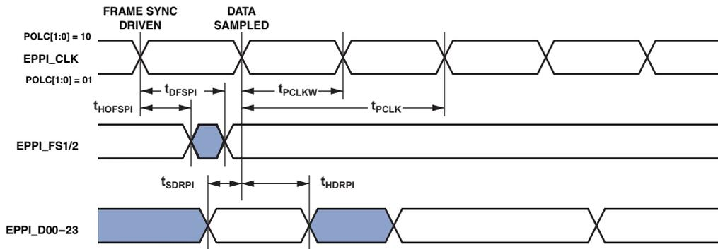
Figure 26. PPI Internal Clock GP Receive Mode with Internal Frame Sync Timing
