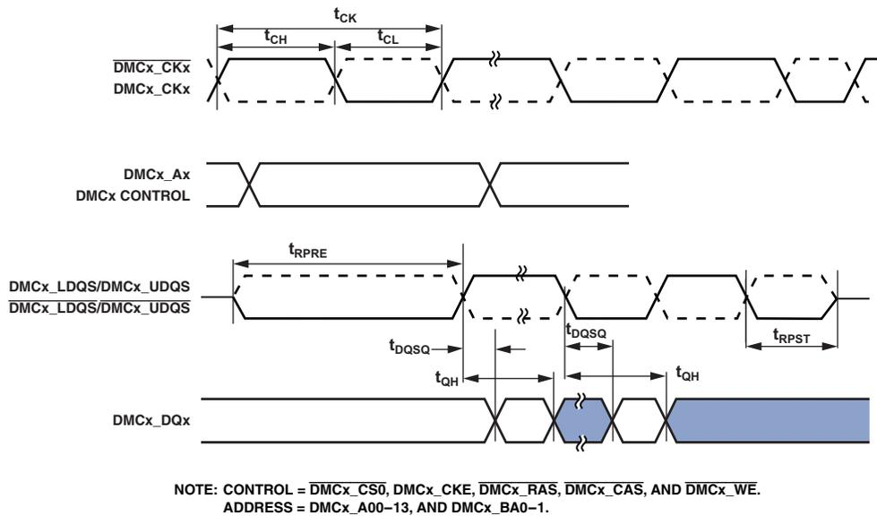
Figure 24. DDR3 SDRAM Controller Input AC Timing
