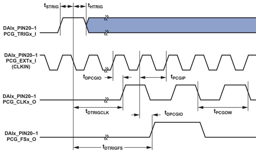
Figure 52. Precision Clock Generator (Direct Pin Routing)
