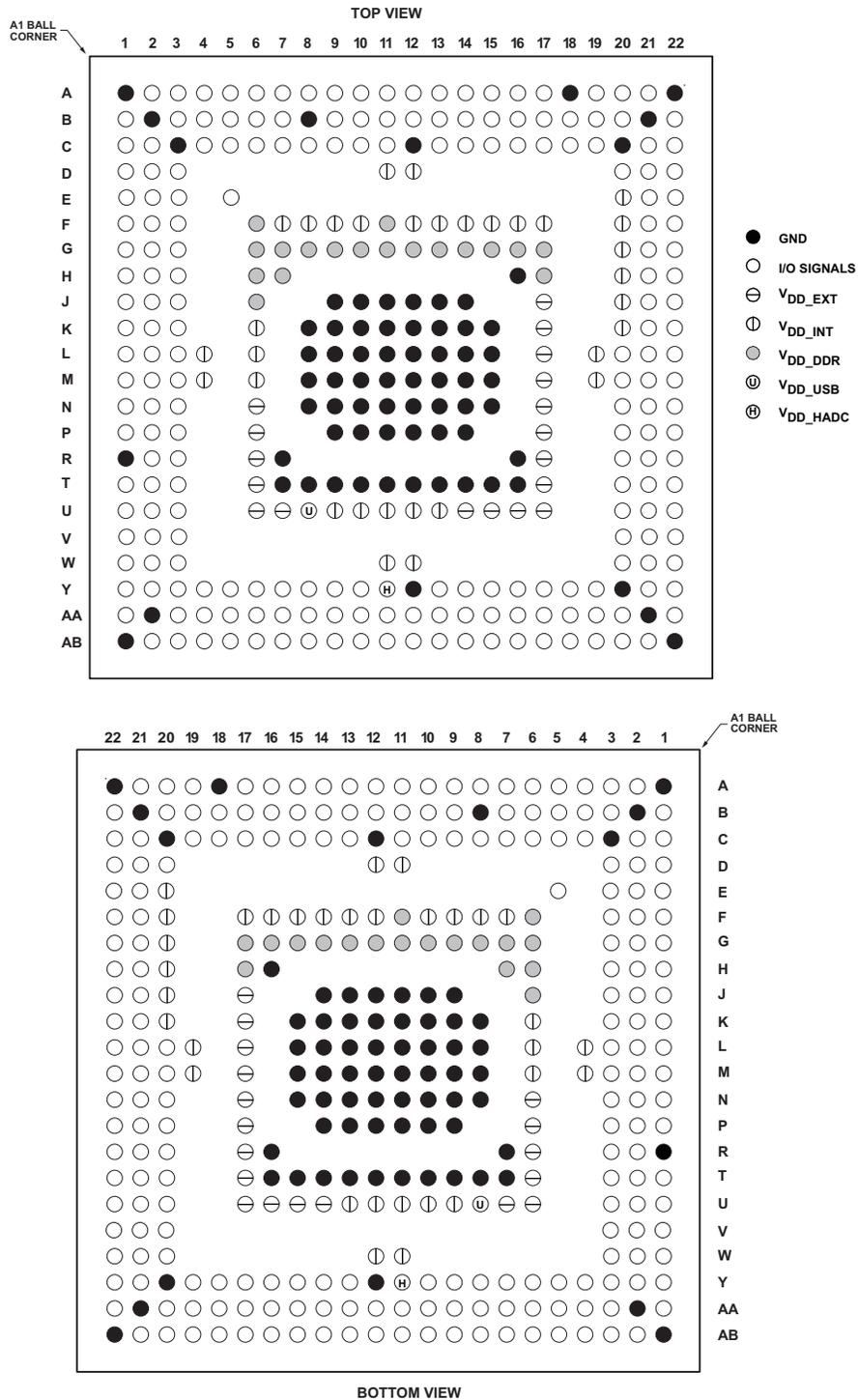
Figure 79. 349-Ball CSP\_BGA Configuration
