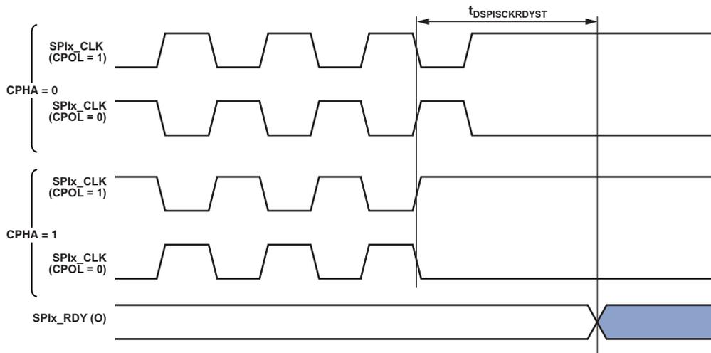
Figure 46. SPIx\_RDY Deassertion from Valid Input SPIx\_CLK Edge in Slave Mode Transmit (FCCH = 1)
