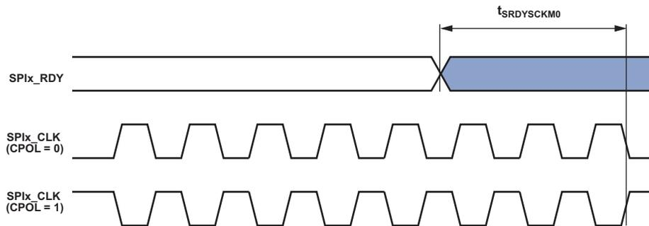
Figure 49. SPIx\_RDY Setup Before SPIx\_CLK with CPHA = 0
