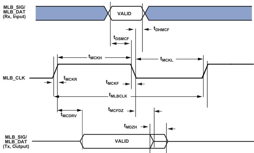
Figure 71. Media Local Bus Timing (3-Pin Interface)
