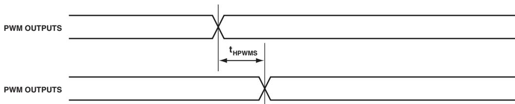
Figure 59. PWM Heightened-Precision Mode Timing, Output Skew
