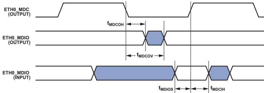
Figure 63. 10/100 Ethernet MAC Controller Timing: RMI Station Management
