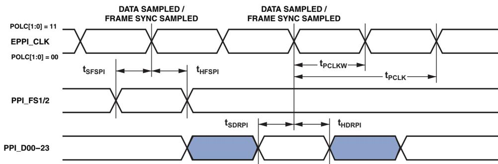
Figure 28. PPI Internal Clock GP Receive Mode with External Frame Sync Timing
