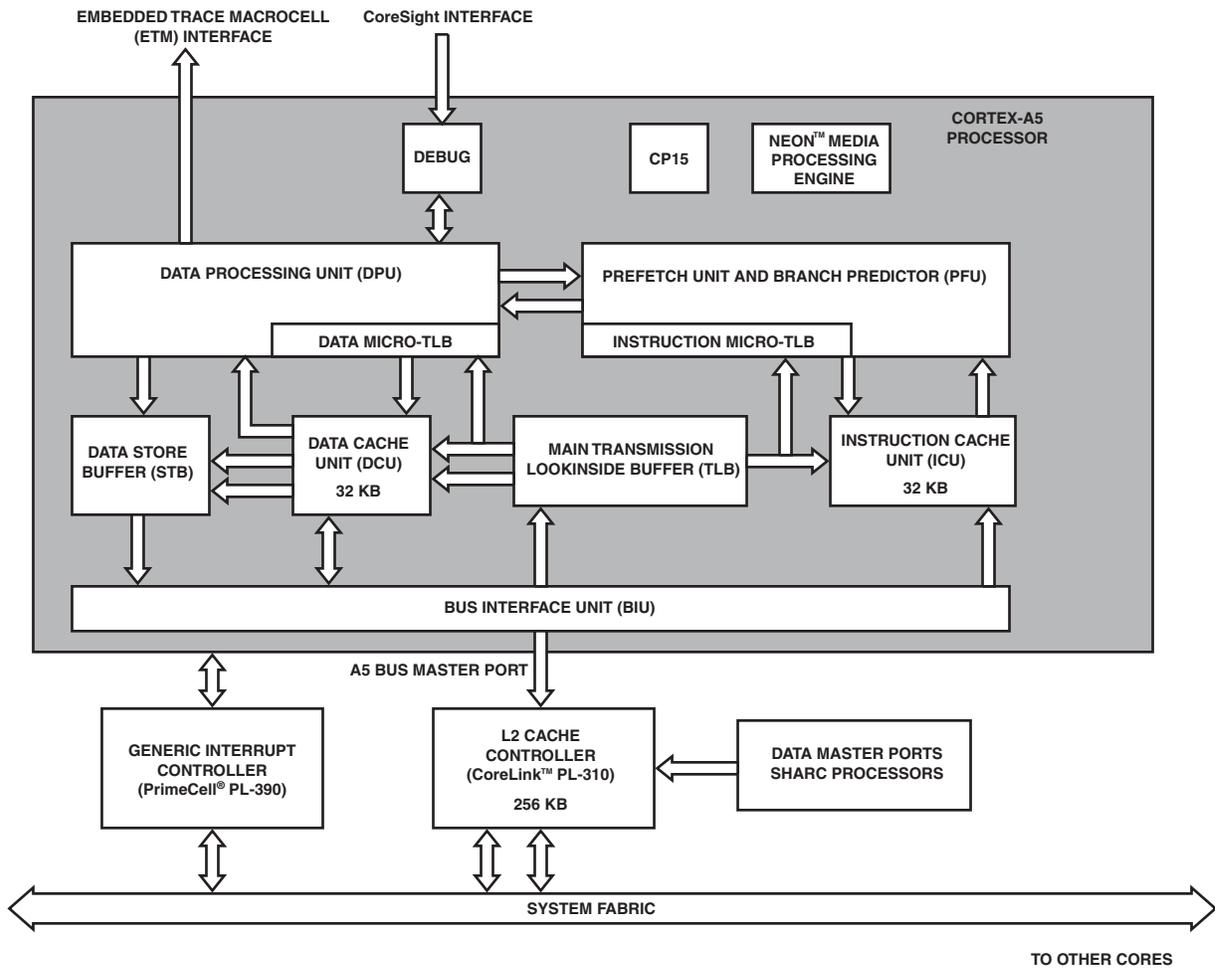
Figure 2. ARM Cortex A-5 Processor Block Diagram
