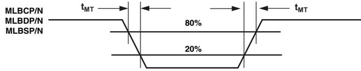
Figure 72. Media Local Bus 6-Pin Transition Time
