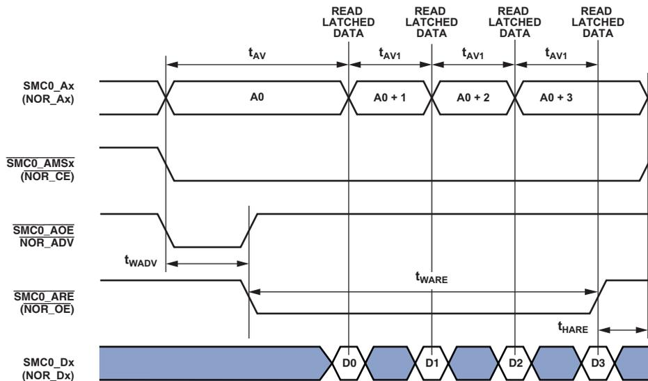
Figure 14. Asynchronous Page Mode Read
