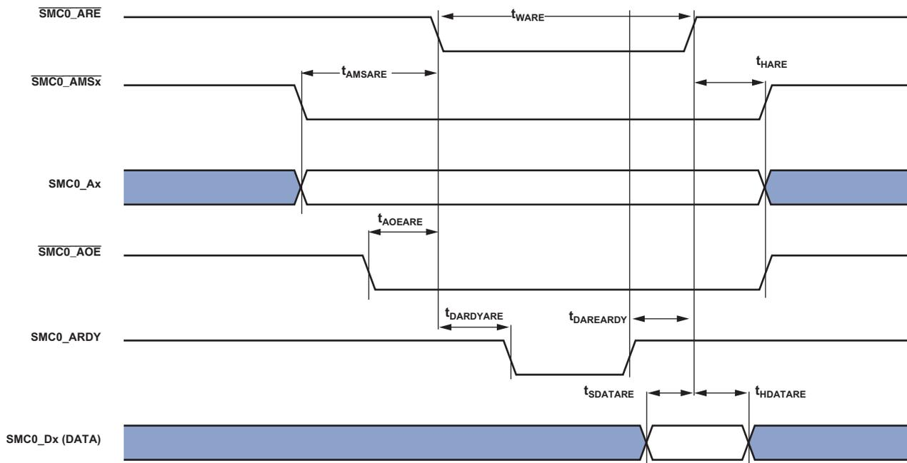
Figure 12. Asynchronous Read
