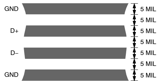
Figure 23. Typical Arrangement of Signal Tracks
