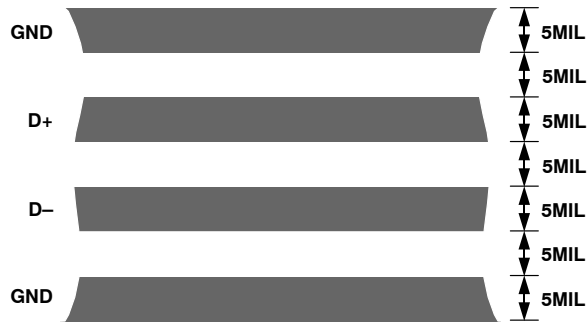
Figure 23. Typical Arrangement of Signal Tracks
