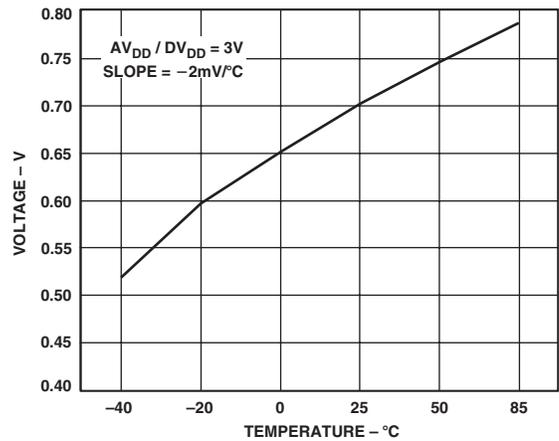
TPC 16. Typical Temperature Sensor Output vs. Temperature
