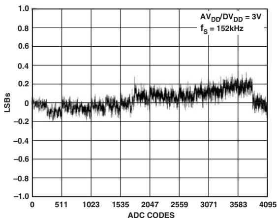
TPC 2. Typical INL Error,  $V_{DD} = 3$  V
