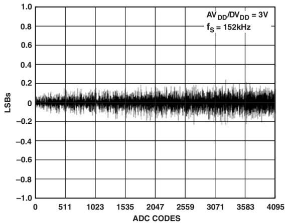
TPC 6. Typical DNL Error,  $V_{DD} = 3\text{ V}$
