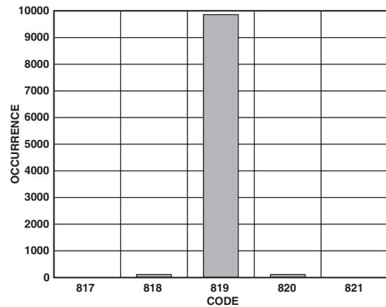
TPC 10. Code Histogram Plot,  $V_{DD} = 3\text{ V}$
