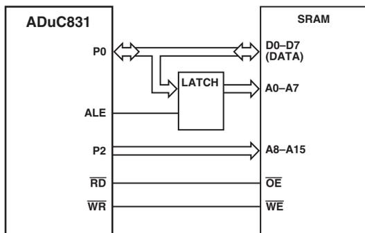
Figure 58. External Data Memory Interface (64 K Address Space)
