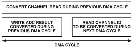
Figure 16. DMA Cycle
