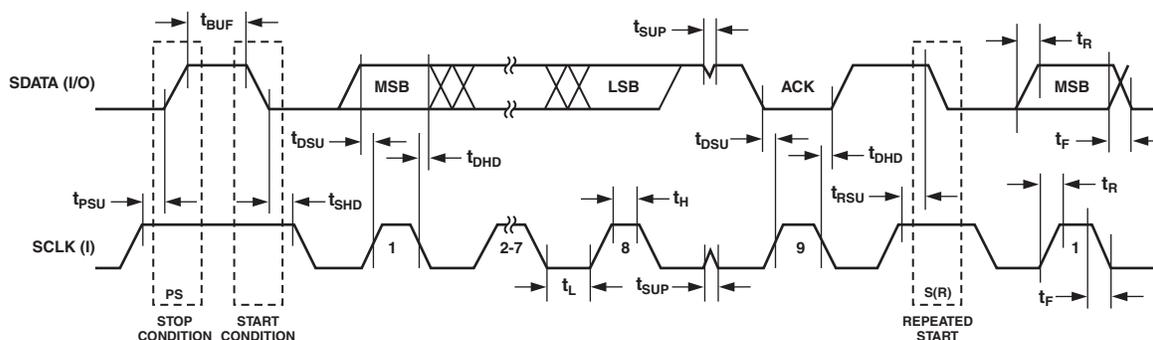
Figure 74. I<sup>2</sup>C Compatible Interface Timing
