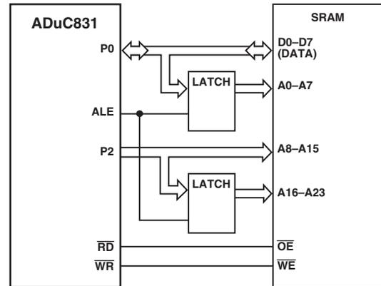
Figure 59. External Data Memory Interface (16 MBytes Address Space)
