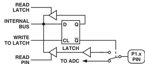
Figure 37. Port 1 Bit Latch and I/O Buffer
