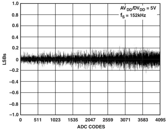
TPC 5. Typical DNL Error,  $V_{DD} = 5\text{ V}$
