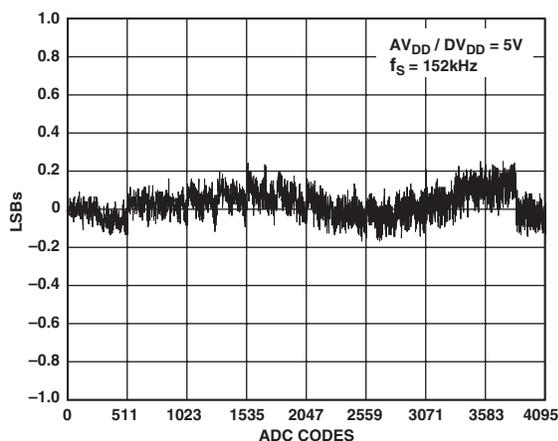
TPC 1. Typical INL Error,  $V_{DD} = 5$  V
