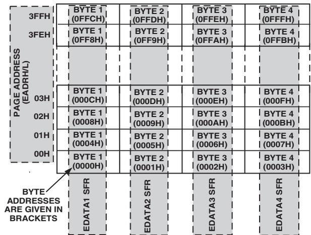
Figure 20. Flash/EE Data Memory Control and Configuration
