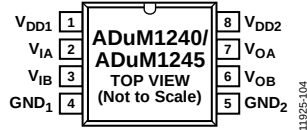
Figure 5. ADuM1240/ADuM1245 8-Lead SOIC (R-8) Pin Configuration
