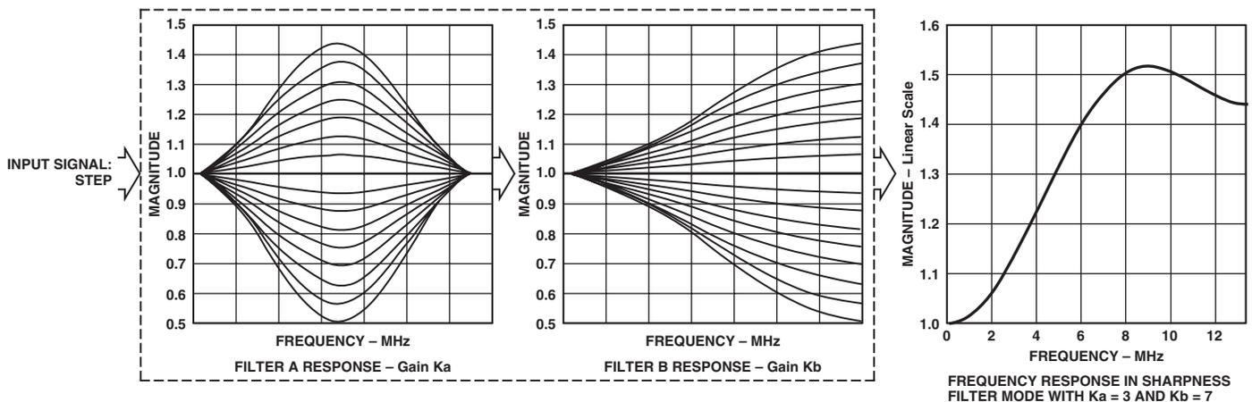
Figure 63. Sharpness and Adaptive Filter Control Block
