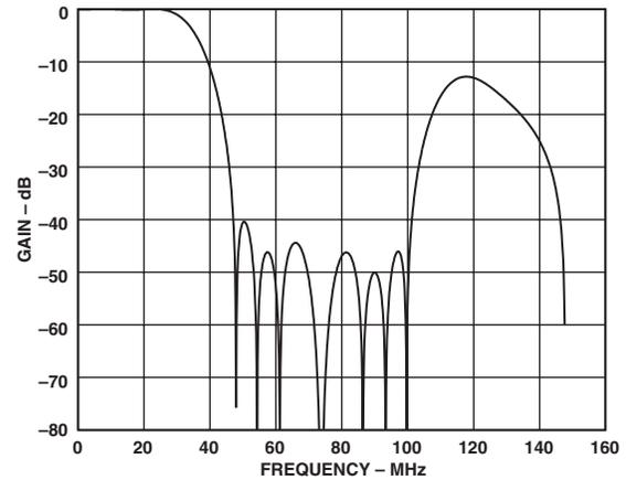
Figure 35. Y – HDTV 2× Oversampling Filter
