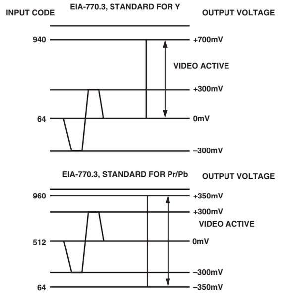
Figure 109. EIA-770.3 Standard Output Signals (1080 i, 720 p)
