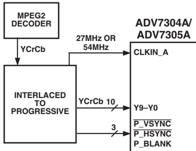
Figure 25. 1 × 10-Bit PS @ 27 MHz or 54 MHz
