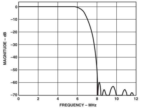
Figure 47. Luma SSAF Filter up to 12 MHz
