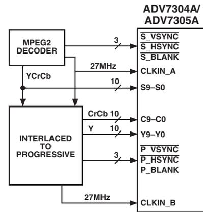
Figure 22. Simultaneous Progressive Scan and SD Input
