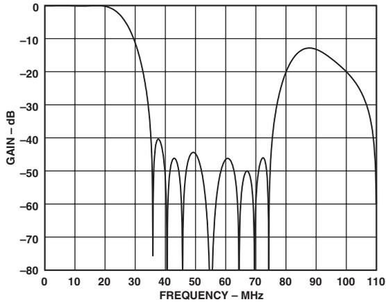
Figure 33. Y – PS 4× Oversampling Filter
