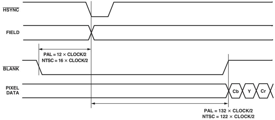
Figure 100. SD Timing Mode 1 Odd/Even Field Transitions, Master/Slave
