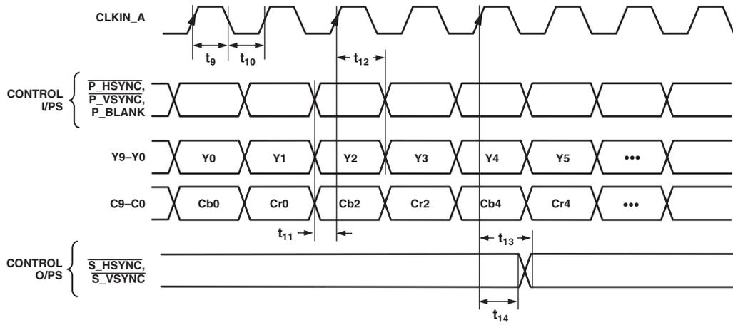
$t_9$  = CLOCK HIGH TIME,  $t_{10}$  = CLOCK LOW TIME,  $t_{11}$  = DATA SETUP TIME,  $t_{12}$  = DATA HOLD TIME
