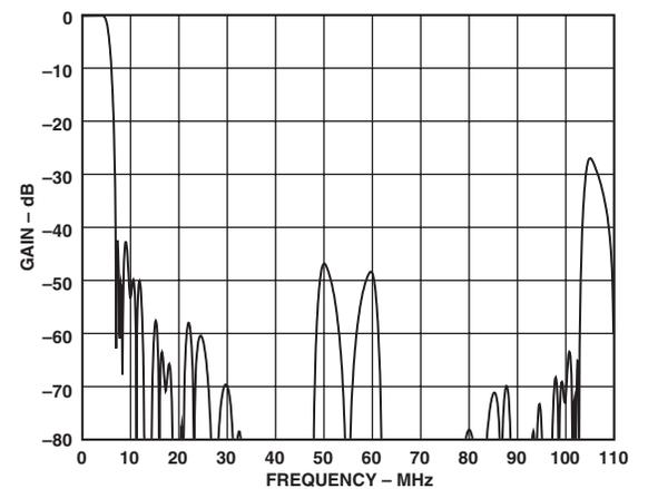
Figure 40. UV - PS 4x Oversampling Filter, SSAF
