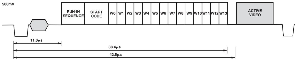
Figure 82. WSS Waveform
