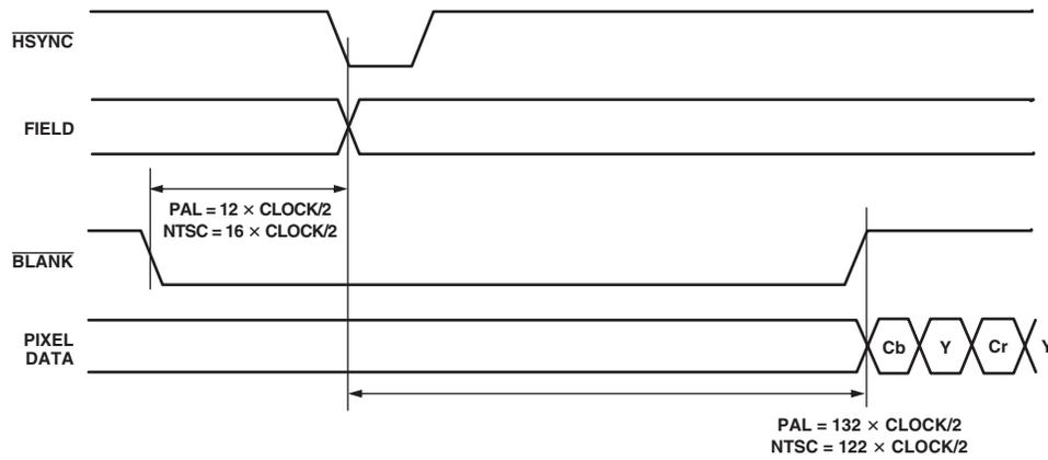
Figure 13. SD Timing Input for Timing Mode 1
