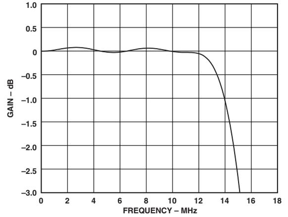
Figure 39. UV - HDTV 2x Oversampling Filter, Pass Band
