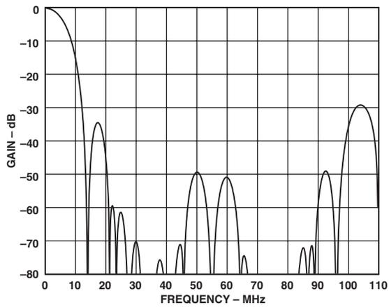
Figure 38. UV - PS 4x Oversampling Filter, Linear
