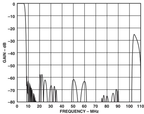
Figure 46. Luma SSAF Filter up to 108 MHz
