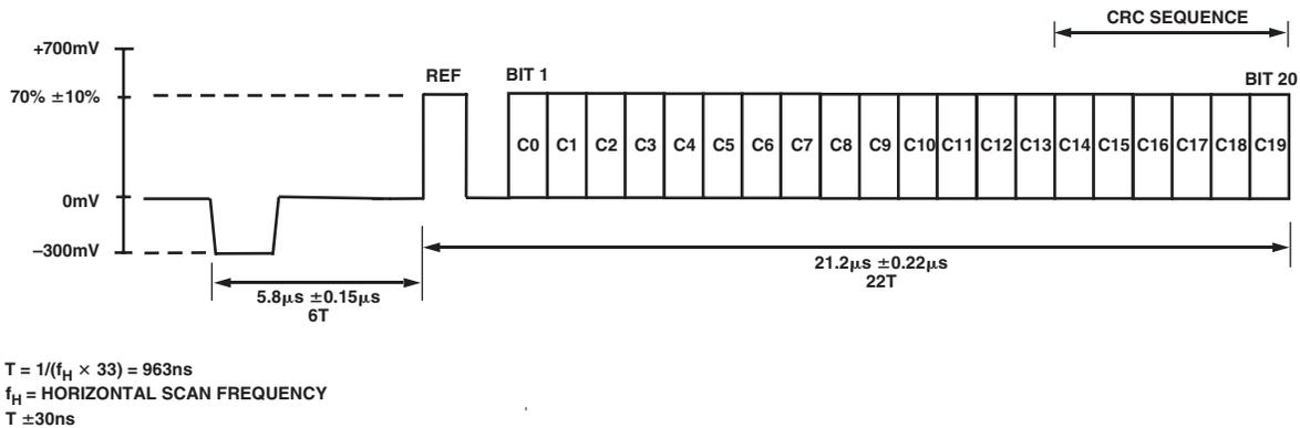
Figure 80. CGMS Waveform
