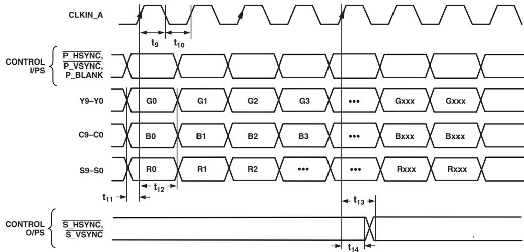
$t_9$  = CLOCK HIGH TIME,  $t_{10}$  = CLOCK LOW TIME,  $t_{11}$  = DATA SETUP TIME,  $t_{12}$  = DATA HOLD TIME
