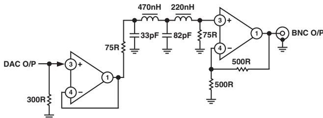
Figure 77. Example for Output Filter HDTV, 2× Oversampling
