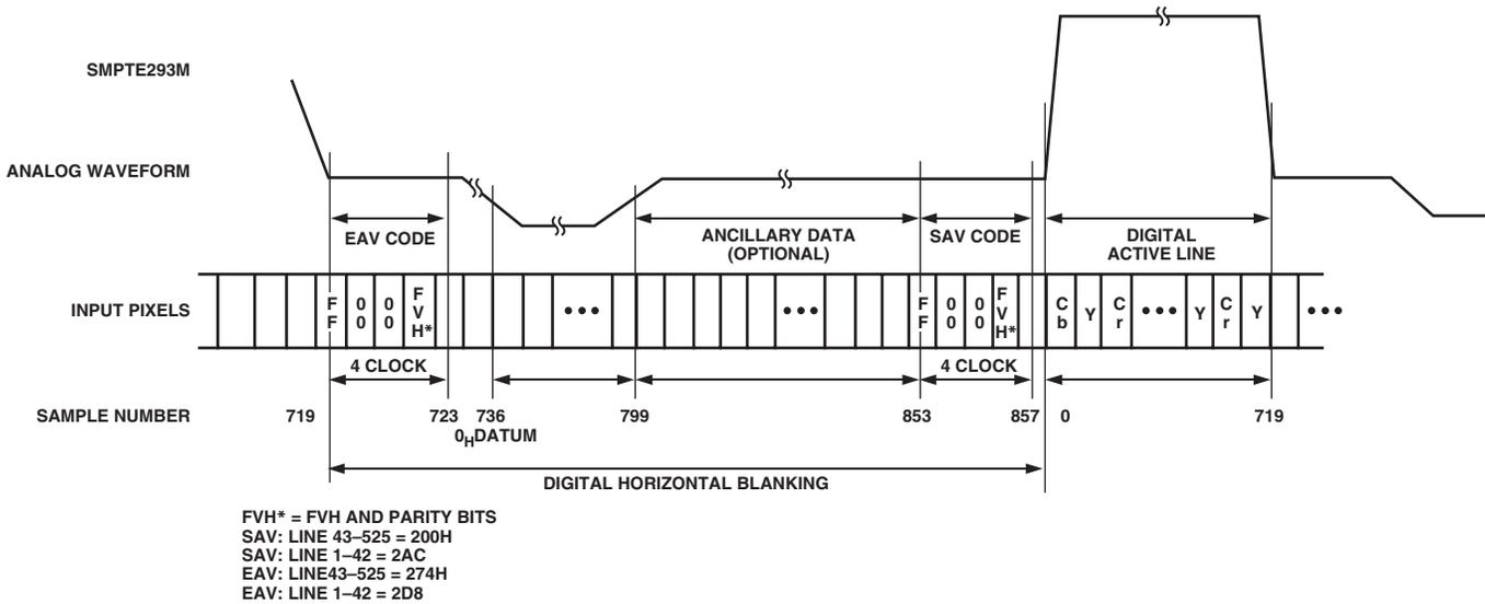
Figure 112. EAV/SAV Input Data Timing Diagram, SMPTE293M
