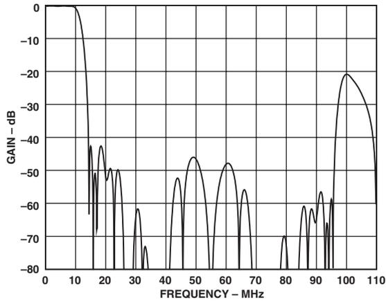
Figure 37. UV - HDTV 2x Oversampling Filter
