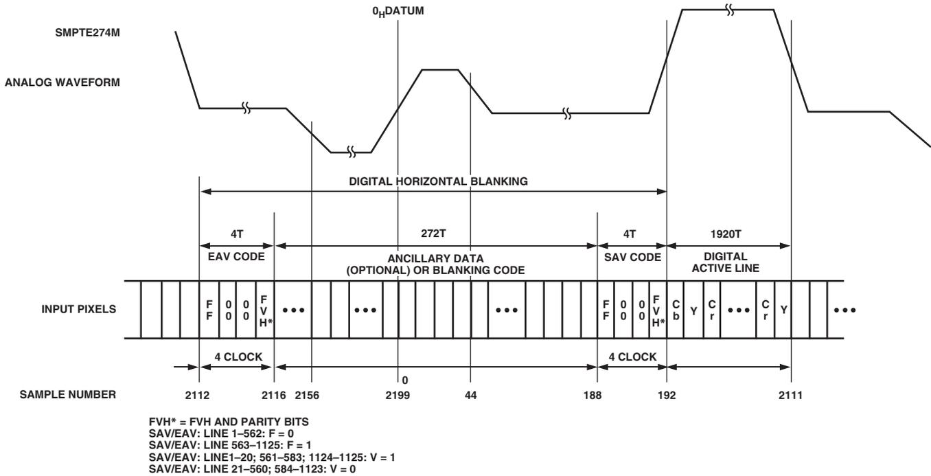
Figure 111. EAV/SAV Input Data Timing Diagram, SMPTE274M
