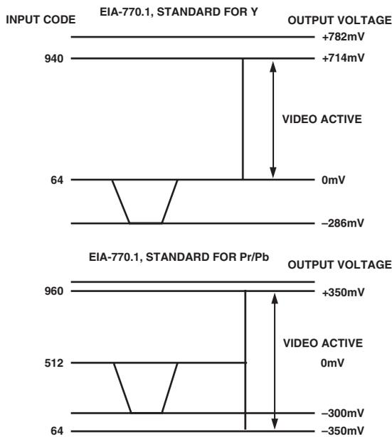
Figure 108. EIA-770.1 Standard Output Signals (525 p)
