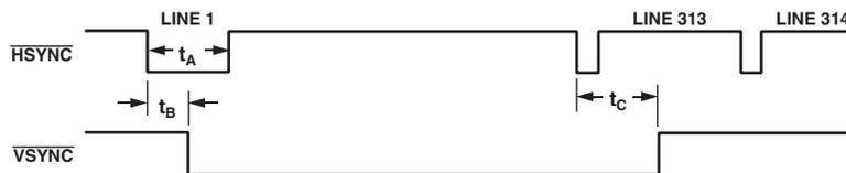
Figure 19. Timing Register 1 in PAL Mode
