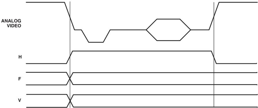
Figure 97. SD Master Mode 0 Data Transitions
