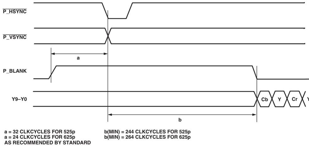
Figure 11. PS 4:2:2 1 × 10-Bit Interleaved @ 54 MHz Input Timing Diagram
