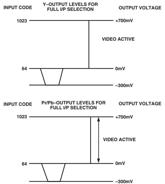
Figure 110. Output Levels for Full Input Selection
