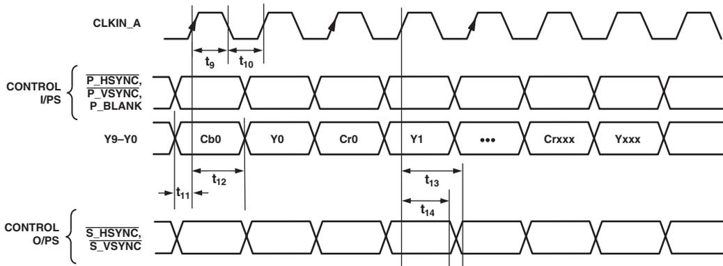
$t_9$  = CLOCK HIGH TIME,  $t_{10}$  = CLOCK LOW TIME,  $t_{11}$  = DATA SETUP TIME,  $t_{12}$  = DATA HOLD TIME
