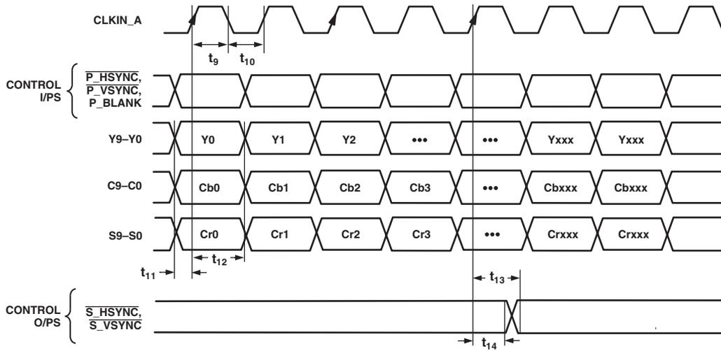
$t_9$  = CLOCK HIGH TIME,  $t_{10}$  = CLOCK LOW TIME,  $t_{11}$  = DATA SETUP TIME,  $t_{12}$  = DATA HOLD TIME
