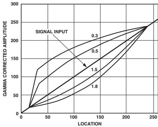
Figure 62. Signal Input (Ramp) and Selectable Gamma Output
