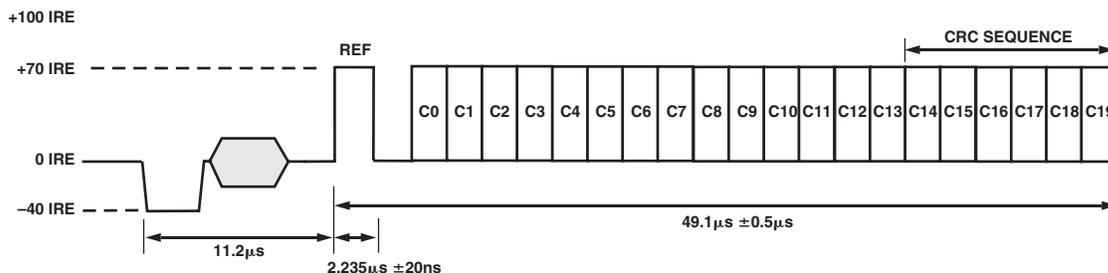
Figure 81. CGMS Waveform
