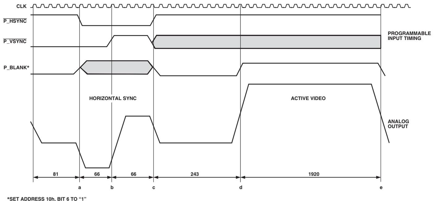
Figure 28. Async Timing Mode, Programming Input Control Signals for SMPTE295M Compatibility
