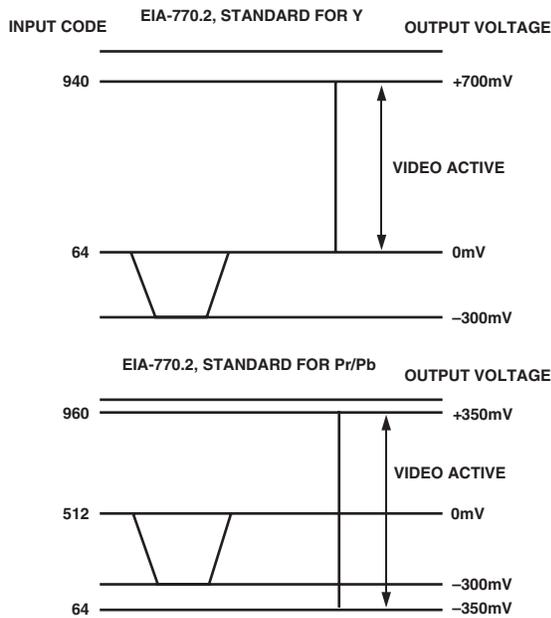
Figure 107. EIA-770.2 Standard Output Signals (525 p)
