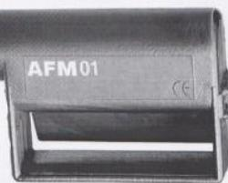
The air-flow monitor provides a simple alternative to indicate positive or negative air flow of fans. When properly installed and connected in series with an optical (i.e. LED) or audible signaling device, a bi-directional switch will activate an electrical contact if the air flow of the fan falls below 8.2 ft/s, turning the signaling device on or off.
