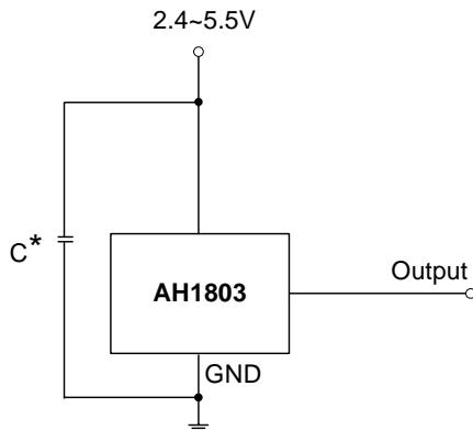
\* C is for power stabilization and to strengthen the noise immunity, the recommended capacitance is 10nF~100nF.
