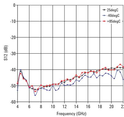
Figure 8. Typical Isolation ( $s_{12}$ ) over temperature
