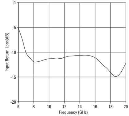
Figure 3 Typical Input Return Loss
