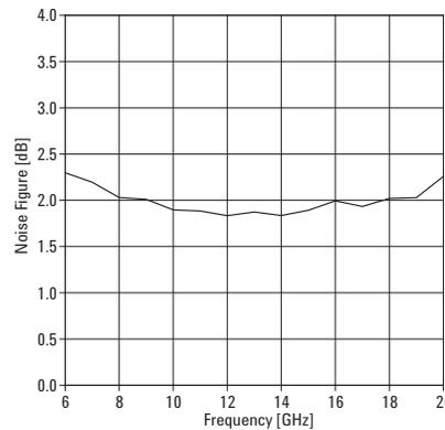
Figure 5. Typical Noise Figure into a 50 W load.
