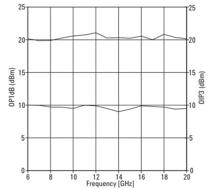
Figure 6. Typical Output  $P_{-1dB}$  and 3<sup>rd</sup> Order Intercept Pt.
