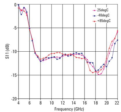
Figure 9. Typical Input Return Loss ( $s_{11}$ ) over temperature
