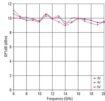
Figure 18. Typical OP<sub>1dB</sub> over Vdd (supply voltage.)
