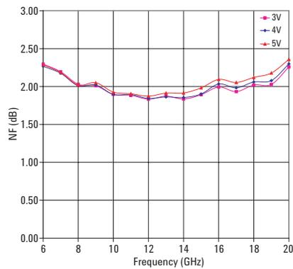
Figure 17. Typical Noise Figure over Vdd (supply voltage.)
