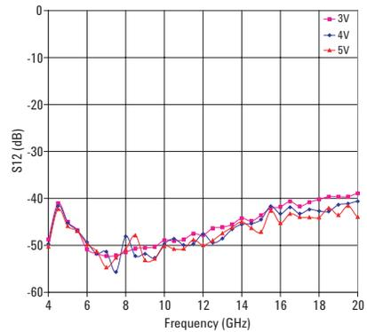
Figure 14. Typical Isolation over Vdd (supply voltage)
