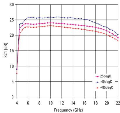
Figure 7. Typical Gain ( $s_{21}$ ) over temperature
