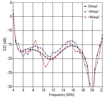
Figure 10. Typical Output Return Loss over Temperature
