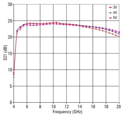
Figure 13. Typical Gain over Vdd (supply voltage.)
