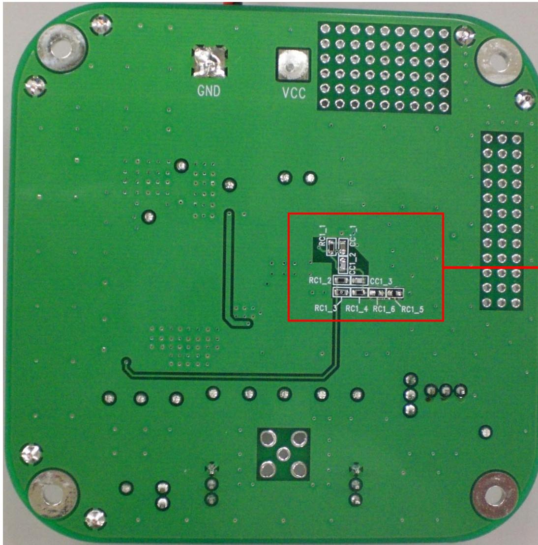
The RC constant for phase compensation is set for output voltage 5.0V.
