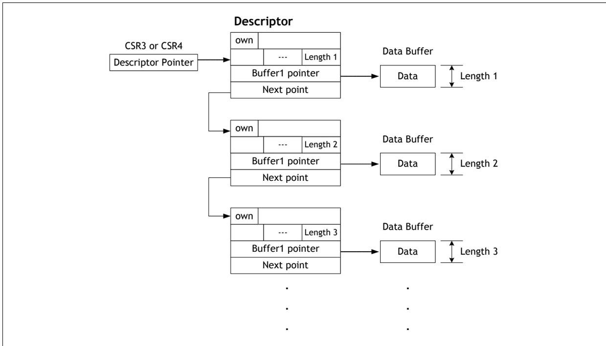
**Figure 6 Chain Structure of Frame Buffer**
