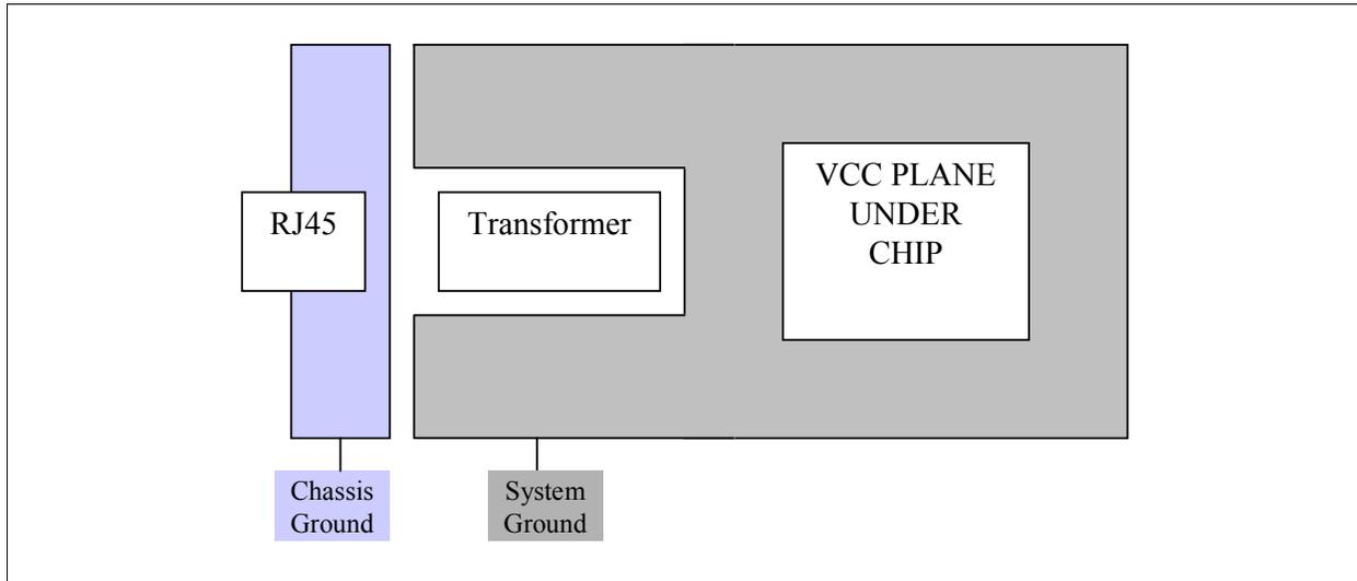
Figure 28 Ground Plane Arrangement
