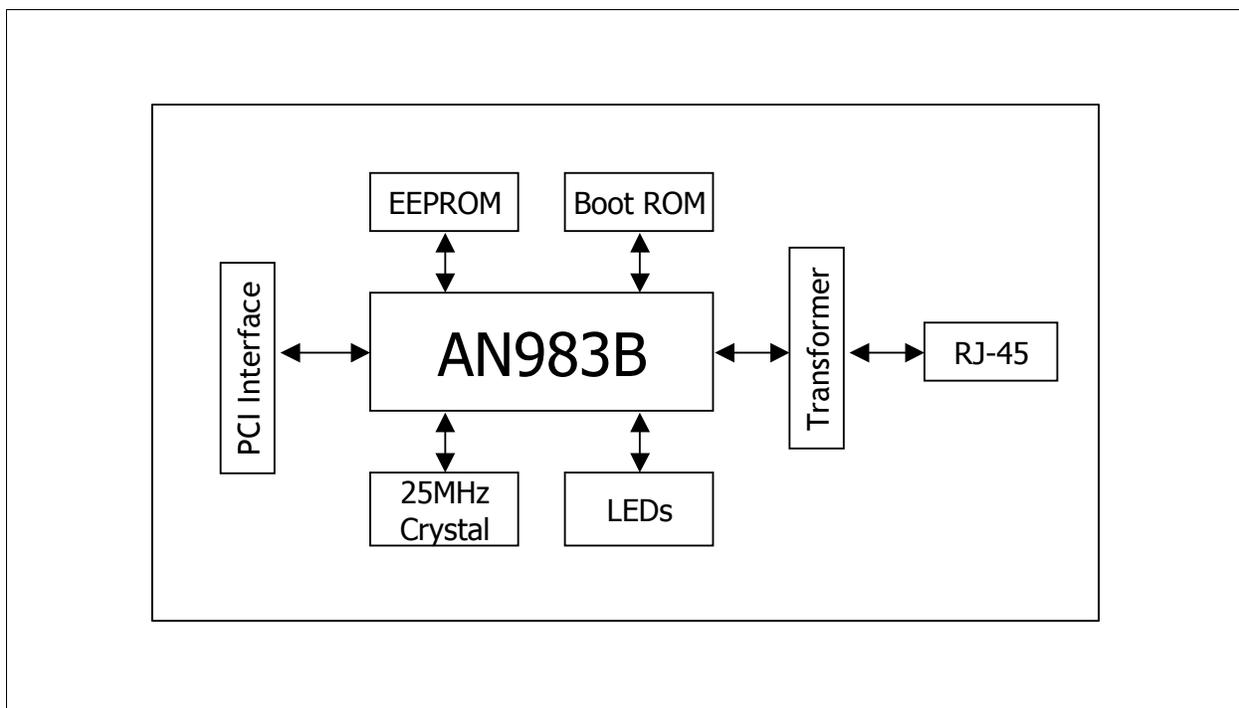
**Figure 1 System Diagram of the AN983B/BX**
