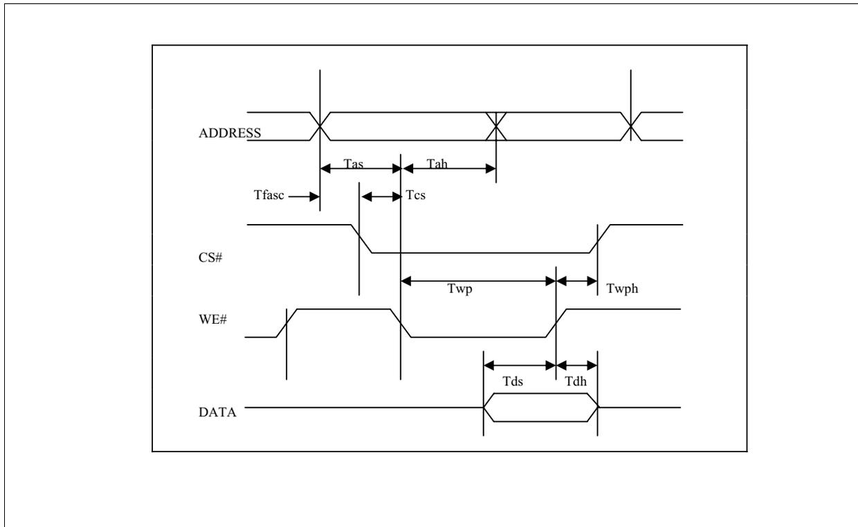
**Figure 18 Flash Write Timings**
