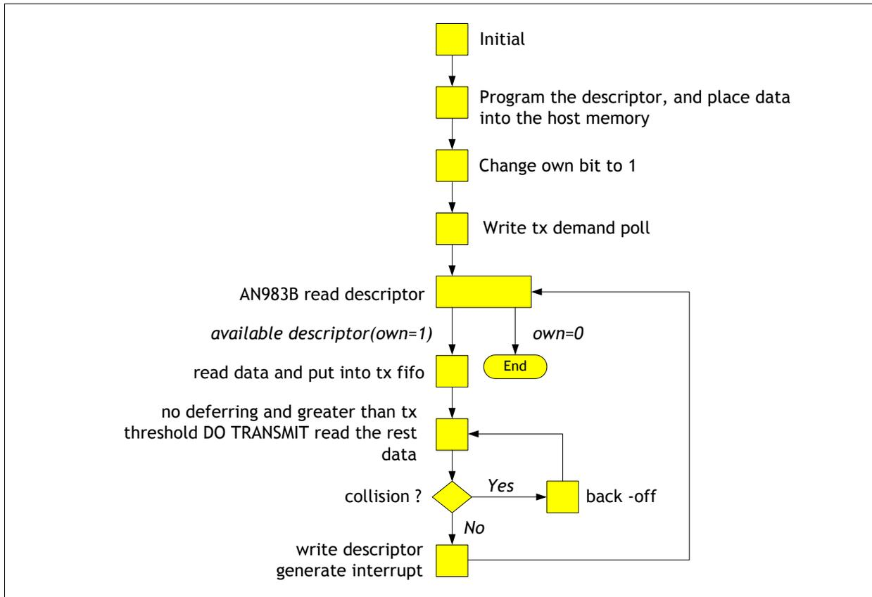
Figure 9 Transmit Flow
