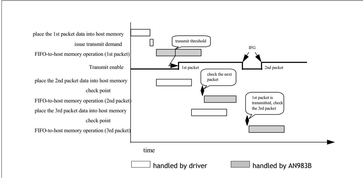
Figure 10 Transmit Data Flow of Pre-fetch Data
