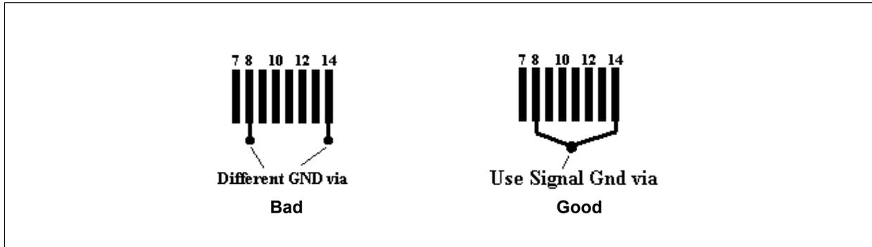
Figure 26 Ground Via Trace Arrangement
