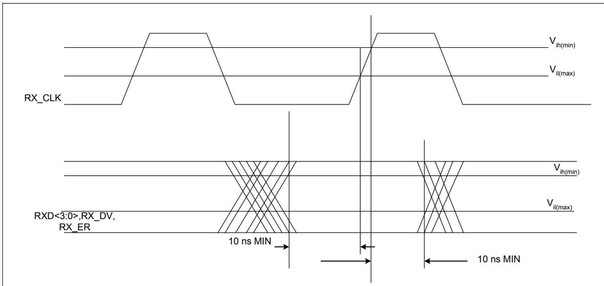
Figure 22 Receive Signal Timing Relations at the MII
