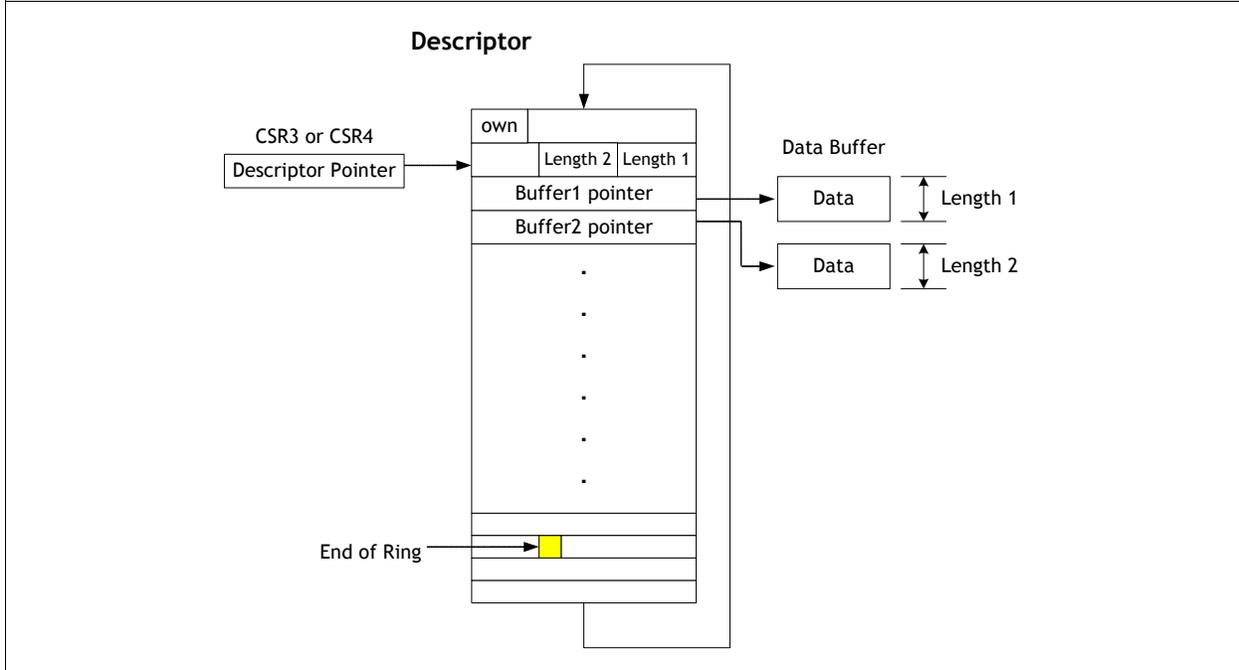
**Figure 5 Ring Structure of Frame Buffer**
