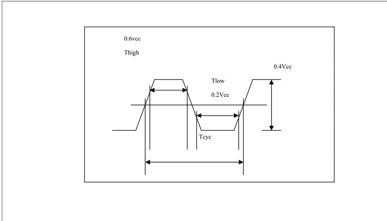
Figure 16 PCI Clock Waveform
