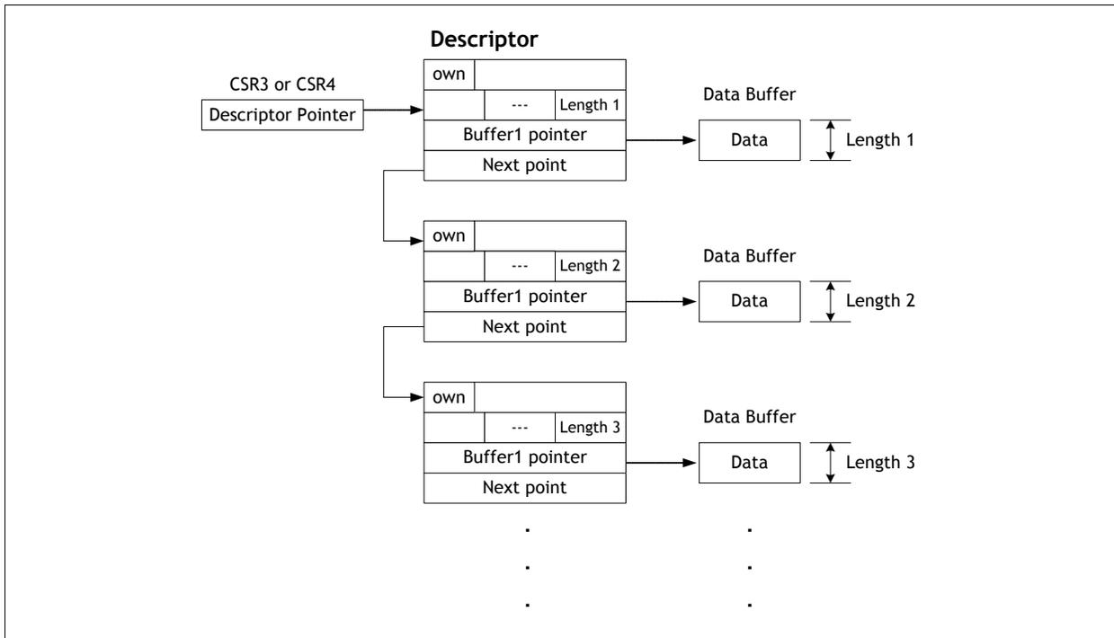
**Figure 6 Chain Structure of Frame Buffer**
