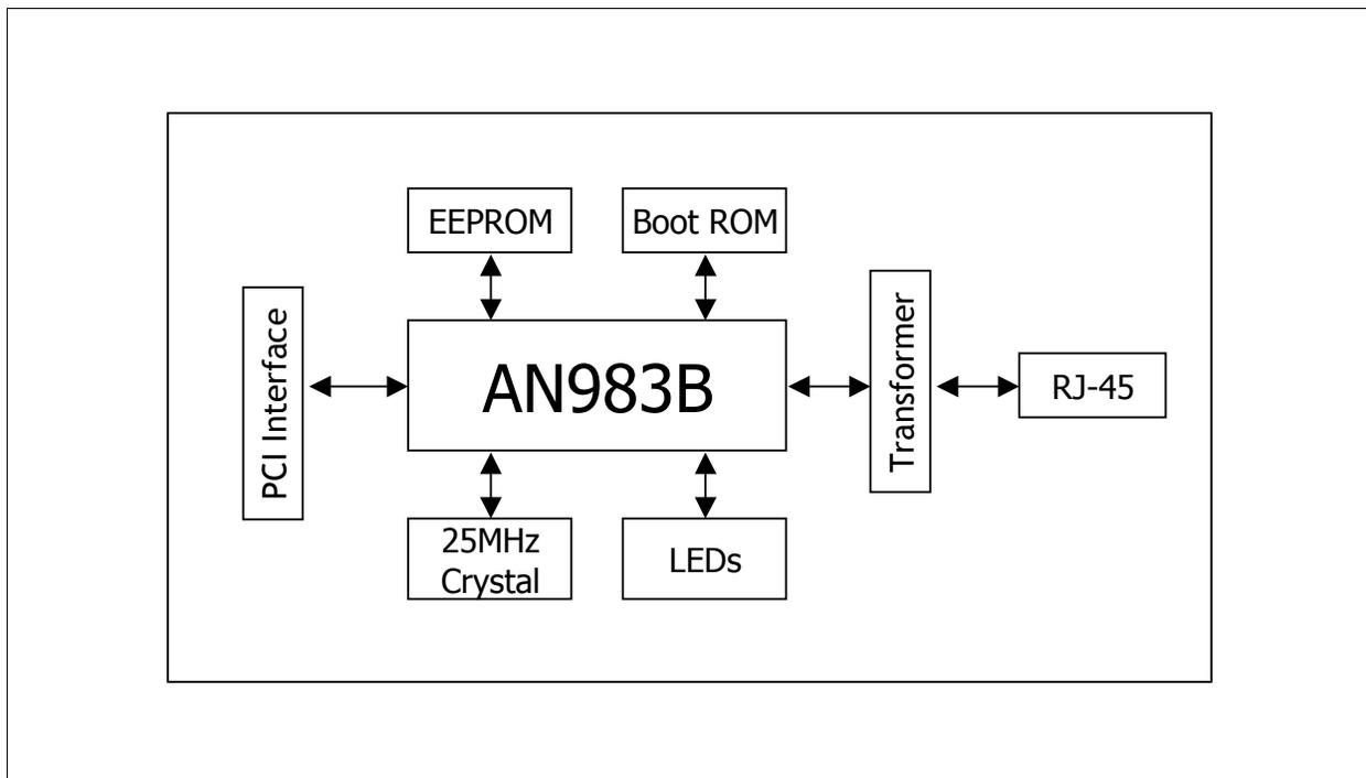
**Figure 1 System Diagram of the AN983B/BX**
