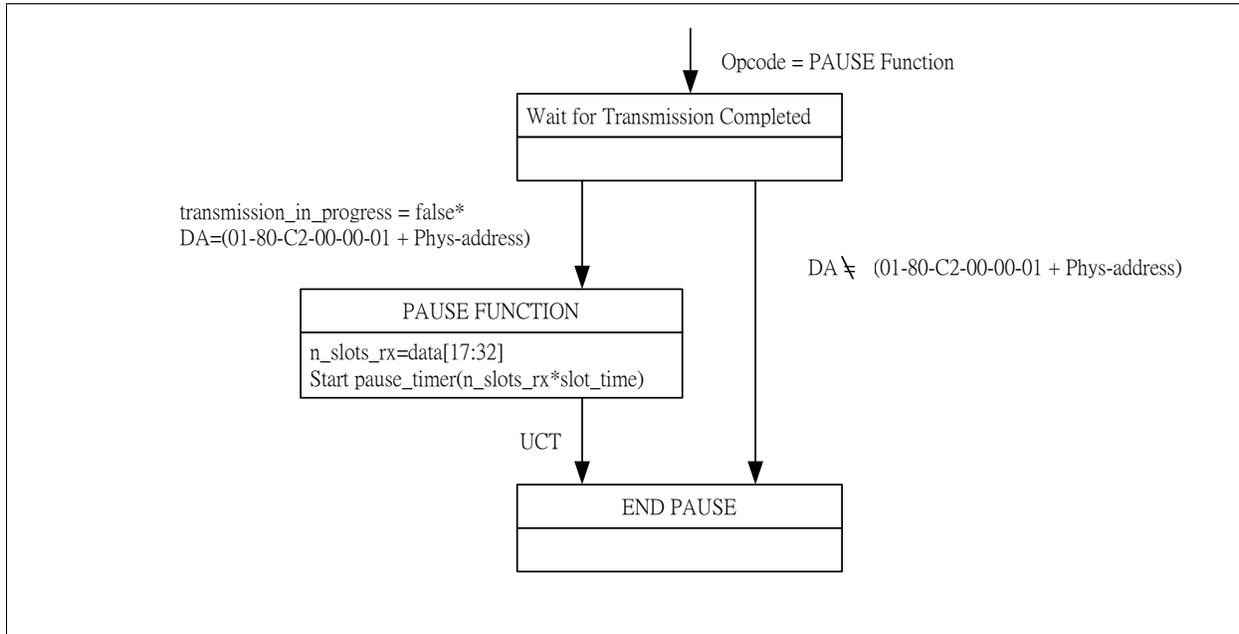
Figure 15 PAUSE Operation Receive State Diagram
