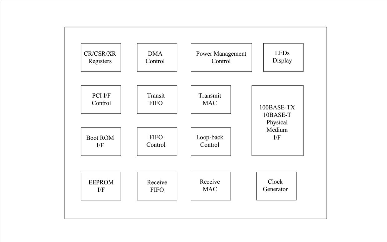
**Figure 2 Block Diagram of the AN983B/BX**
