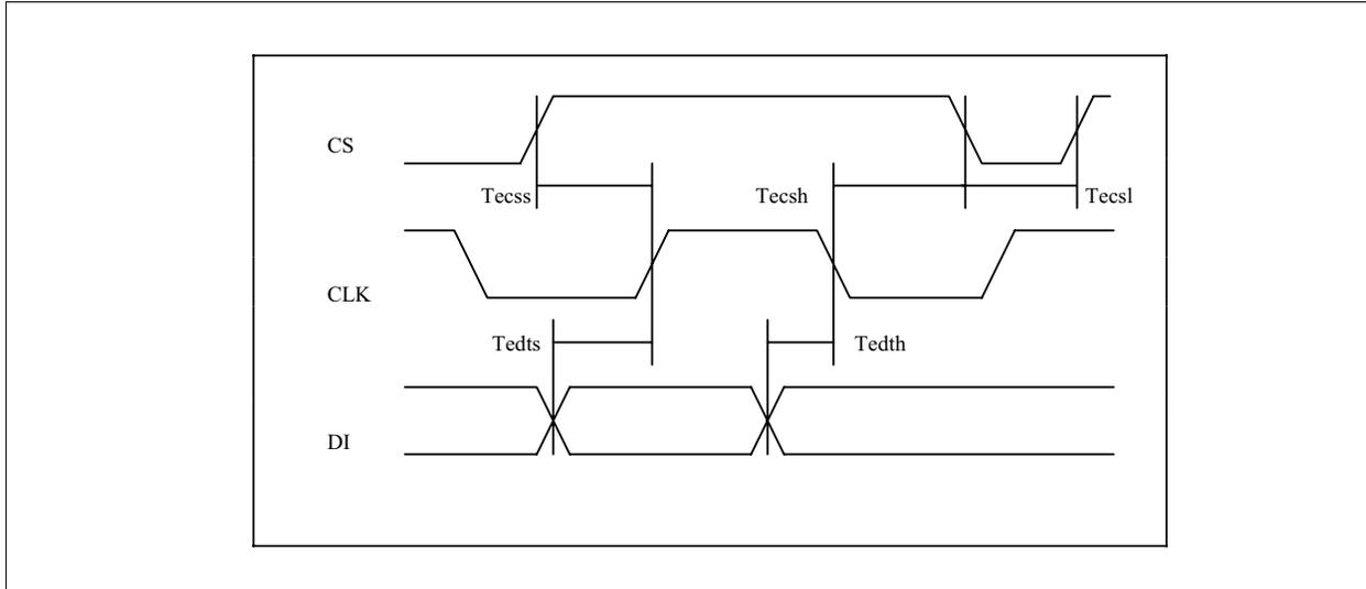
Figure 20 Serial EEPROM Timing
