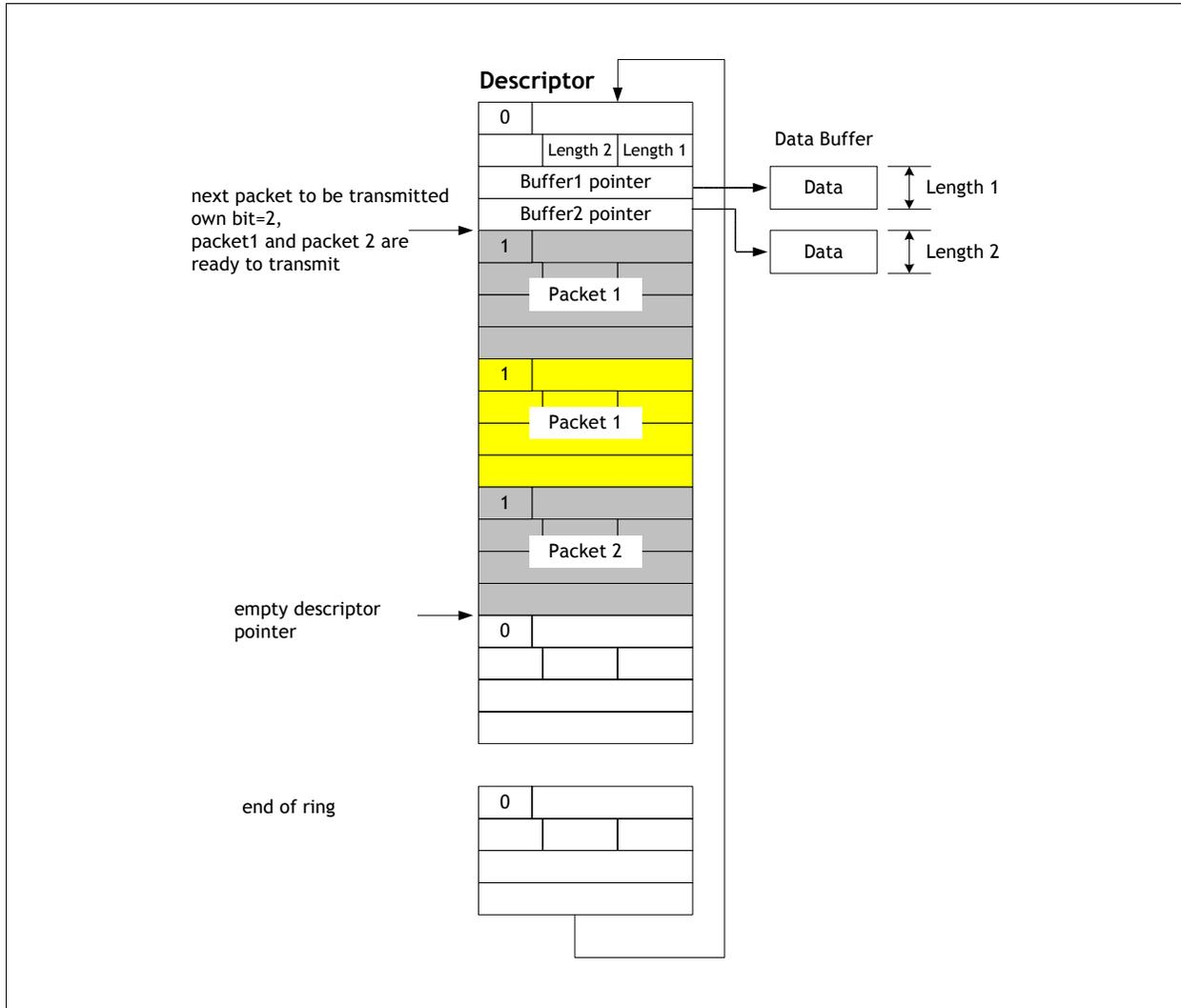
Figure 7 Transmit Pointers for Descriptor Management
