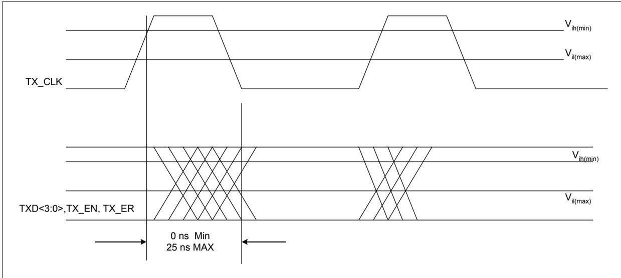
Figure 21 Transmit Signal Timing Relationships at the MII
