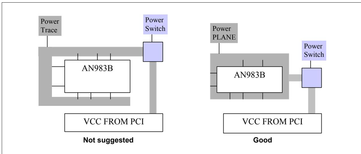
**Figure 27** Power Trace Arrangement
