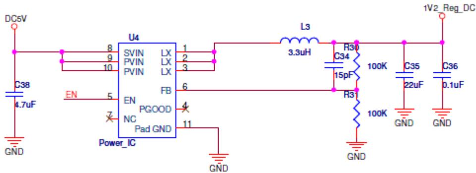
Notes: the Power IC used in the diagrams above is able to deliver up to 3A output current in case of changes or replacement in NAND Flash memories.
