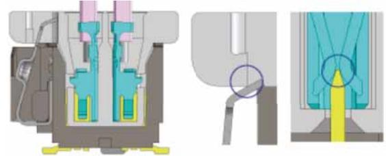
Simultaneous timing of locking function and Figure 1. contact mating provides a clearer tactile click.
