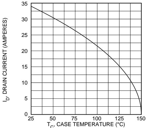
**FIGURE 6, MAXIMUM DRAIN CURRENT vs CASE TEMPERATURE**
