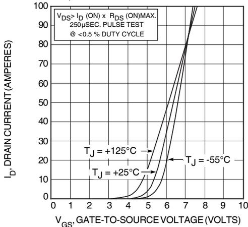
FIGURE 4, TRANSFER CHARACTERISTICS
