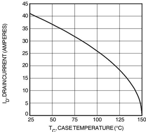
FIGURE 6, MAXIMUM DRAIN CURRENT vs CASE TEMPERATURE
