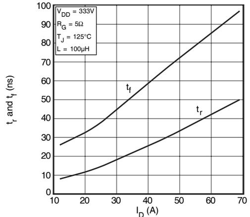
FIGURE 15, RISE AND FALL TIMES vs CURRENT
