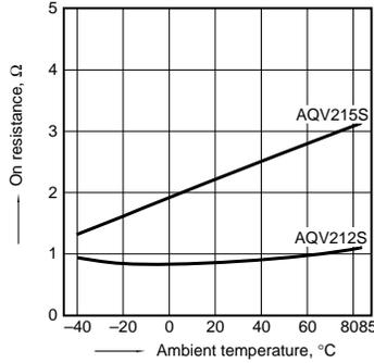
2.-(2) On resistance vs. ambient temperature characteristics
