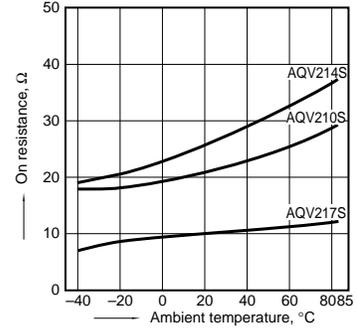
2.-(3) On resistance vs. ambient temperature characteristics
