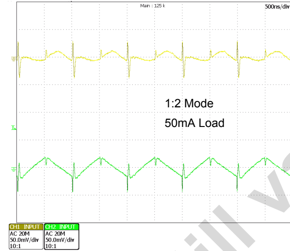
Figure 11. Charge Pump input and output ripple
