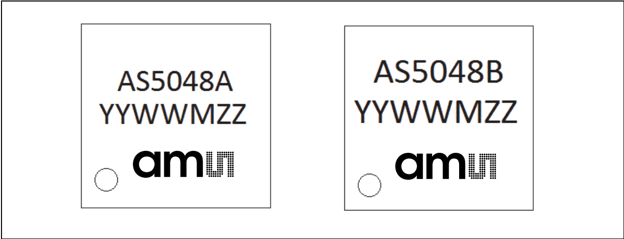
Figure 38: Package Markings for AS5048A & AS5048B
