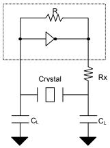
$$\begin{split} C_\text{L} &= 2^*(C_\text{P} - C_\text{S}),\\ \text{Where } C_\text{P} &= \text{Load capacitance of crystal}\\ C_\text{S} &= \text{Stray capacitance due to } C_\text{IN,} \text{ PCB, Trace etc.} \end{split}$$
