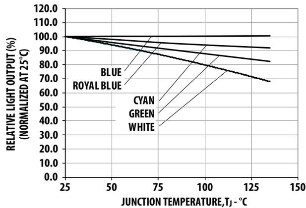
Figure 20. Relative Light Output vs. Junction Temperature.
