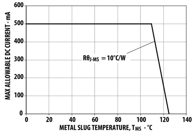
Figure 11. Maximum Forward Current vs. Metal Slug Temperature.
