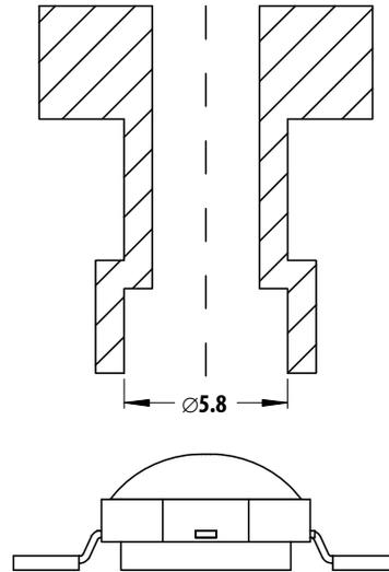
Figure 25. Recommended pick and place nozzle tip.
