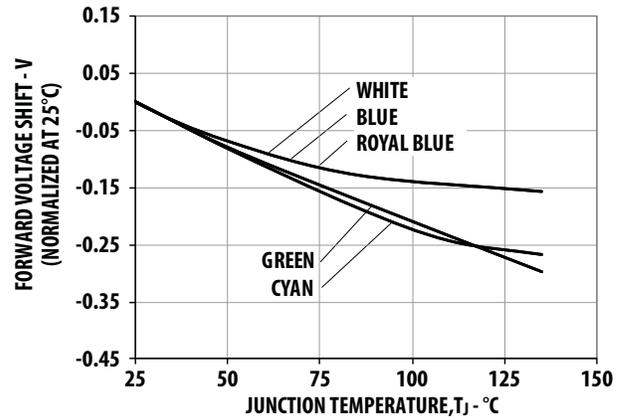
Figure 21. Forward Voltage Shift vs. Junction Temperature.
