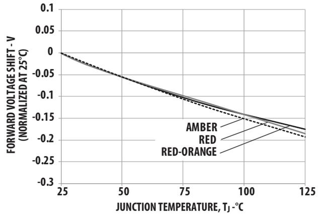
Figure 9. Forward Voltage Shift vs. Junction Temperature.
