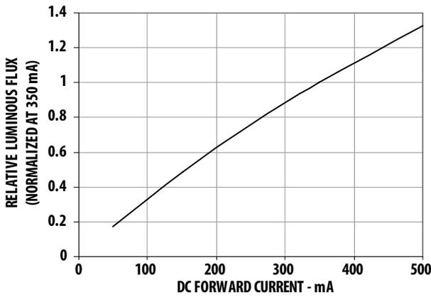
Figure 14. Relative Luminous Flux vs. Mono Pulse Current.
