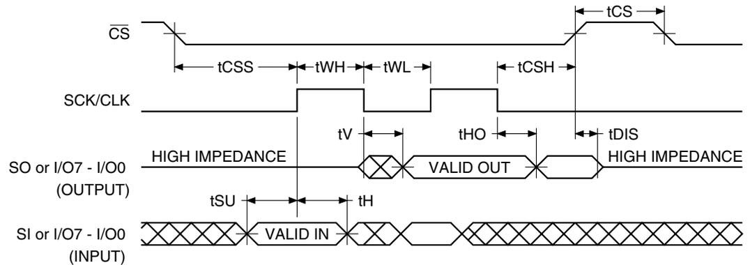
**Waveform 2 – Inactive Clock Polarity High and SPI Mode 3**
