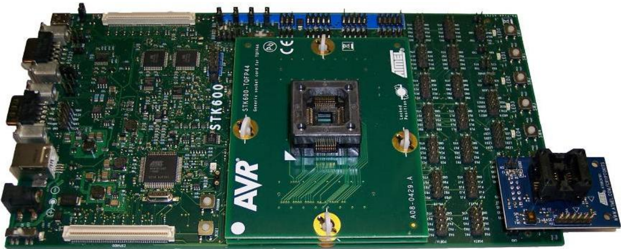
Figure 2-2. Atmel AT88CK101BK8 adapter board mounted to STK600
