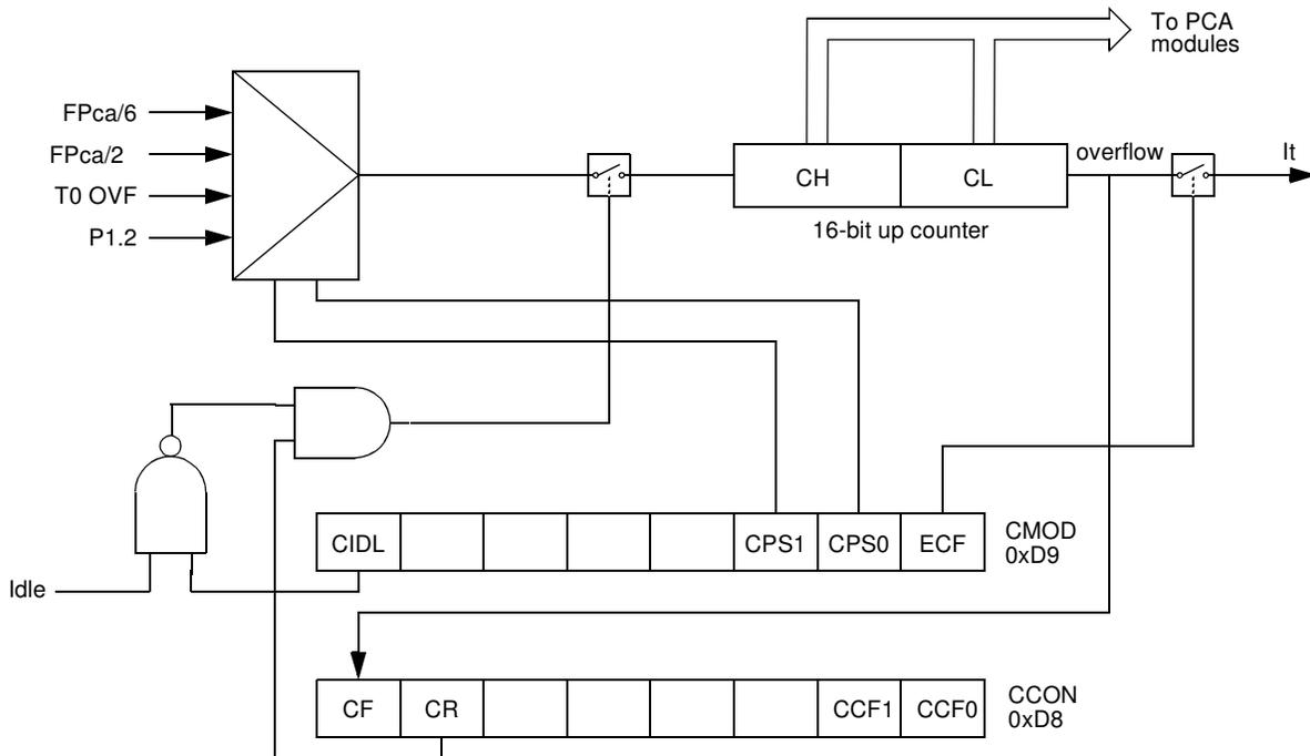
The CMOD register includes three additional bits associated with the PCA.
