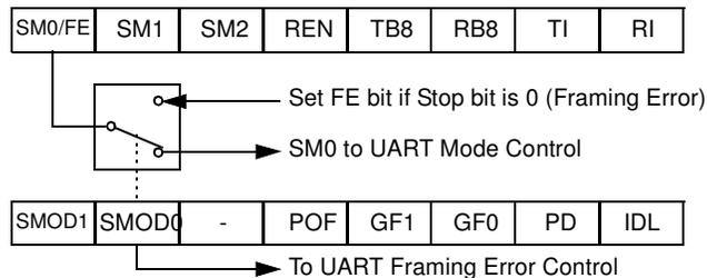
When this feature is enabled, the receiver checks each incoming data frame for a valid stop bit. An invalid stop bit may result from noise on the serial lines or from simultaneous transmission by two CPUs. If a valid stop bit is not found, the Framing Error bit (FE) in SCON register bit is set.
