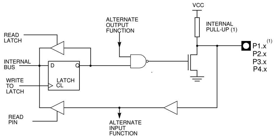
Note: 1. The internal pull-up can be disabled on P1 when analog function is selected.
