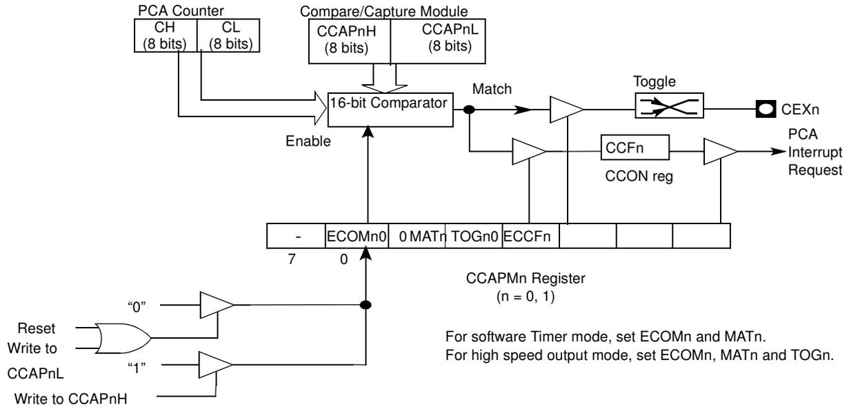
**High Speed Output Mode** In this mode the CEX output (on port 1) associated with the PCA module will toggle each time a match occurs between the PCA counter and the module's capture registers. To activate this mode the TOG, MAT, and ECOM bits in the module's CCAPMn SFR must be set.
