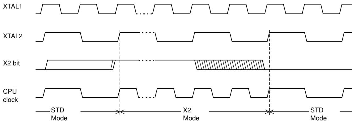
Note: 1. In order to prevent any incorrect operation while operating in the X2 Mode, users must be aware that all peripherals using the clock frequency as a time reference (UART, timers...) will have their time reference divided by 2. For example, a free running timer generating an interrupt every 20 ms will then generate an interrupt every 10 ms. A UART with a 4800 baud rate will have a 9600 baud rate.
