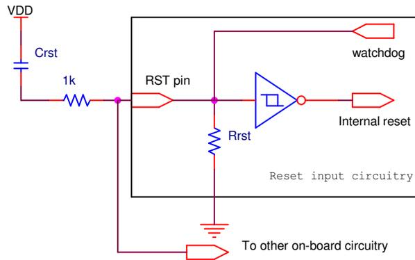
Figure 7 shows the reset circuitry when an external reset circuit is used.
