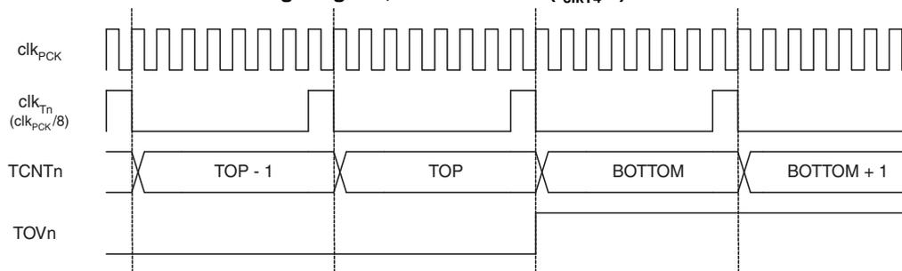
**Figure 15-18. Timer/Counter Timing Diagram, Setting of OCF1x, with Prescaler ( $f_{clkT4}/8$ )**
