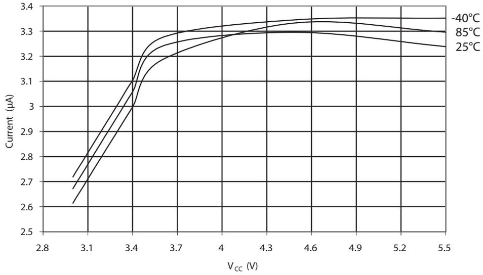
**Figure 30-41. ADC Internal V<sub>REF</sub> vs. V<sub>CC</sub>**
