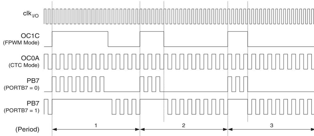
In this example, Timer/Counter0 provides the carrier, while the modulating signal is generated by the Output Compare unit C of the Timer/Counter1.
