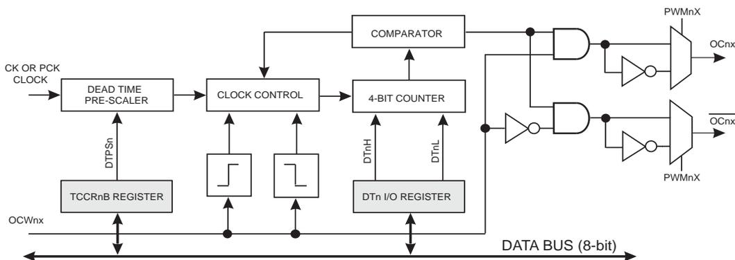
The length of the counting period is user adjustable by selecting the dead time prescaler setting by using the DTPS41:40 control bits, and selecting then the dead time value in I/O register DT4. The DT4 register consists of two 4-bit fields, DT4H and DT4L that control the dead time periods of the PWM output and its' complementary output separately in terms of the number of prescaled dead time generator clock cycles. Thus the rising edge of
