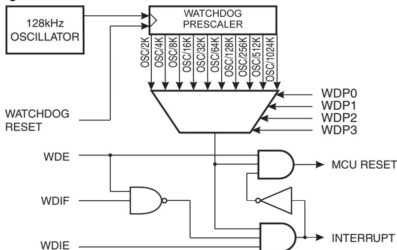
The Watchdog Timer (WDT) is a timer counting cycles of a separate on-chip 128kHz oscillator. The WDT gives an interrupt or a system reset when the counter reaches a given time-out value. In normal operation mode, it is required that the system uses the WDR - Watchdog Timer Reset - instruction to restart the counter before the time-out value is reached. If the system doesn't restart the counter, an interrupt or system reset will be issued.
