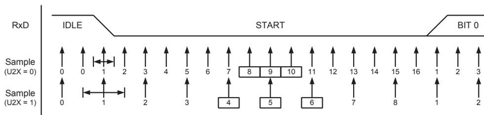
When the clock recovery logic detects a high (idle) to low (start) transition on the RxDn line, the start bit detection sequence is initiated. Let sample 1 denote the first zero-sample as shown in [Figure 18-5](#). The clock
