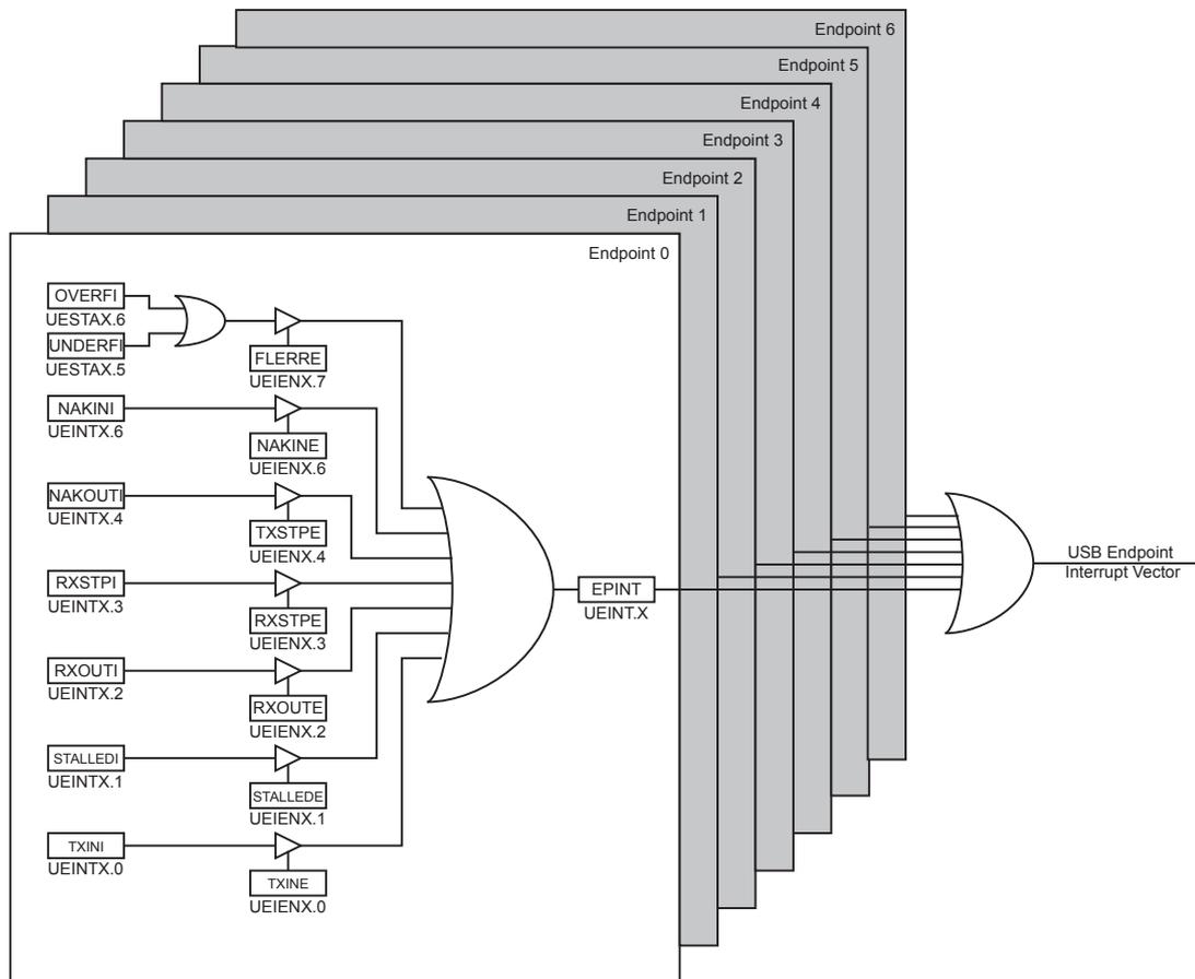
Each endpoint has eight interrupts sources associated with flags, and each source can be enabled or not to trigger the corresponding endpoint interrupt. If, for an endpoint, at least one of the sources is enabled to trigger interrupt, the corresponding event(s) will make the program branch to the USB Endpoint Interrupt vector. The user may determine the source (endpoint) of the interrupt by reading the UEINT register, and then handle the event detected by polling the different flags.
