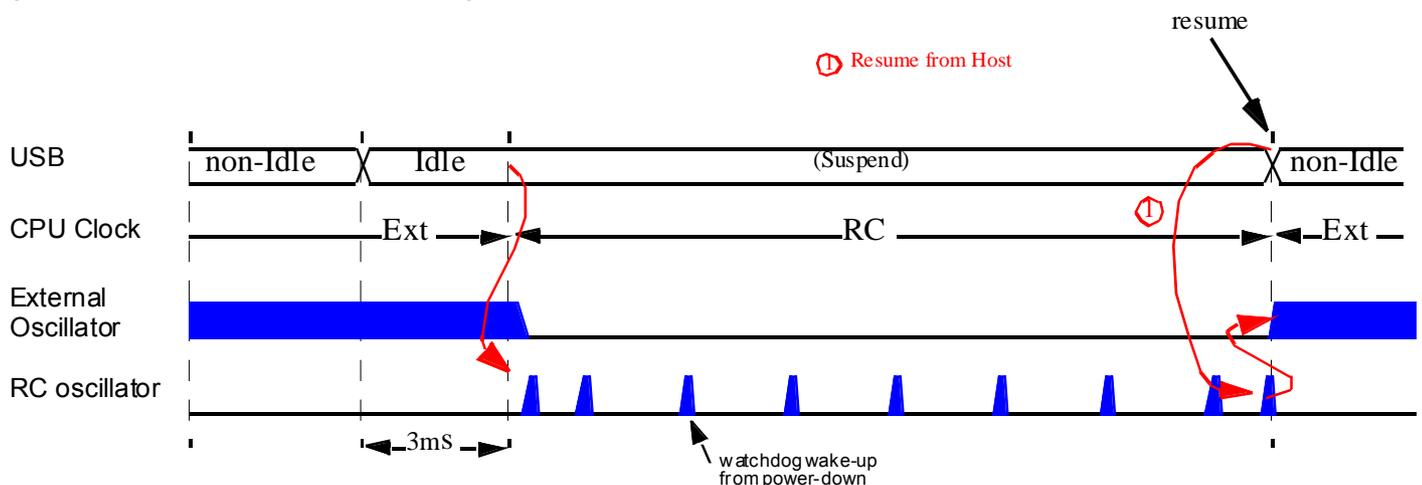
Figure 6-5. Example of Clock Switching with Wake-up from Device
