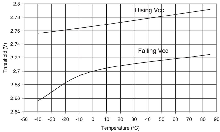
Figure 30-29. BOD Thresholds vs. Temperature (BODLEVEL is 3.5V)
