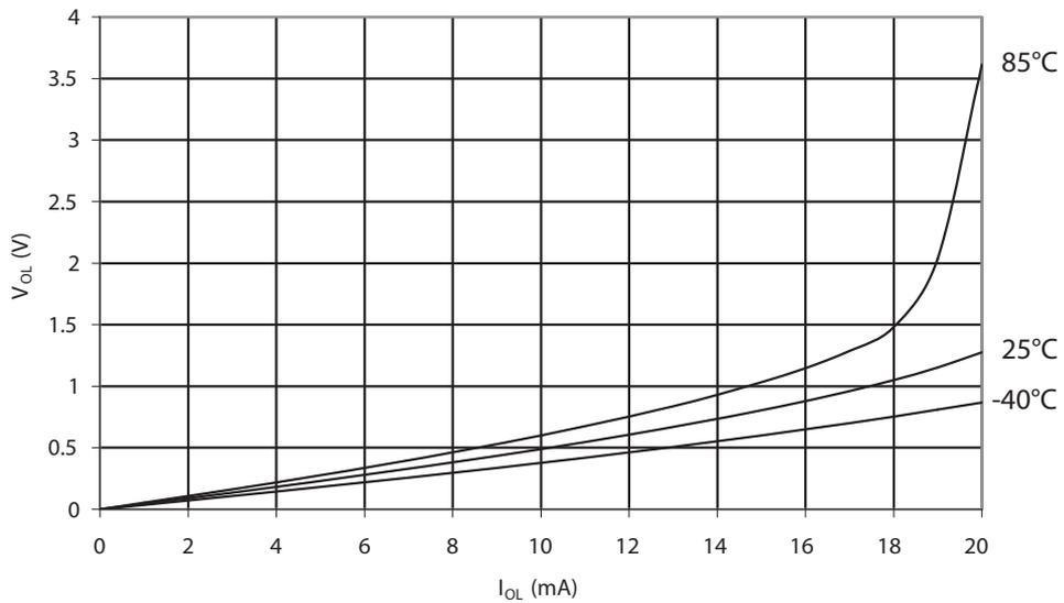
Figure 30-18. I/O Pin Output Voltage vs. Sink Current ( $V_{CC} = 5V$ )
