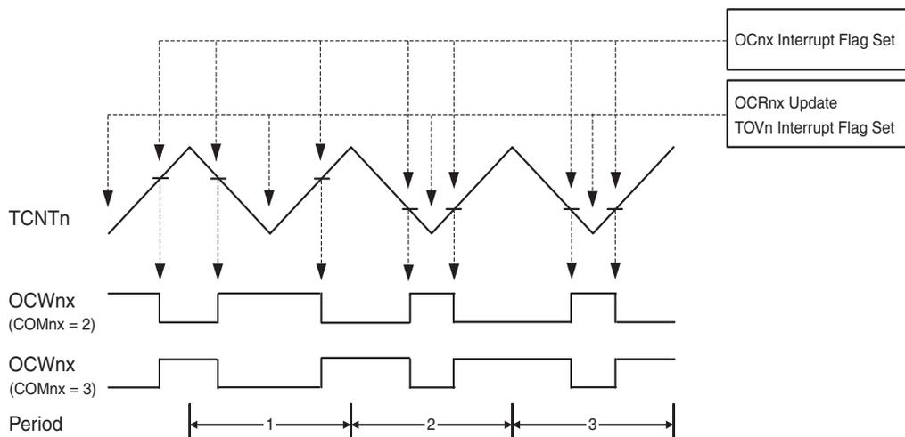
The Timer/Counter Overflow Flag (TOV4) is set each time the counter reaches BOTTOM. The Interrupt Flag can be used to generate an interrupt each time the counter reaches the BOTTOM value.
