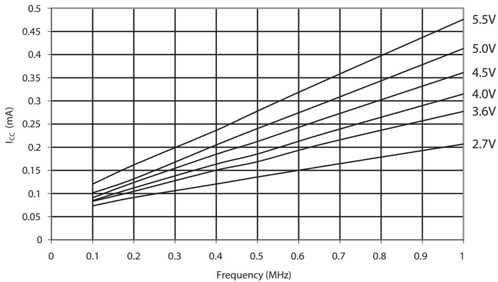
Figure 30-8. Idle Supply Current vs. Frequency (1 - 16MHz) T = 25°C
