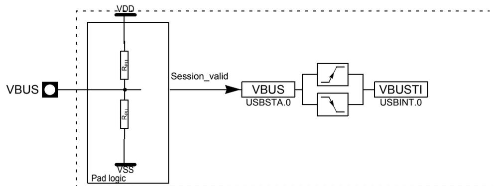
The control logic of the VBUS pad outputs a signal regarding the VBUS voltage level:
