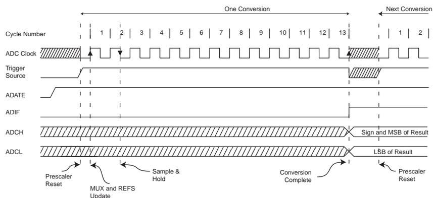
**Figure 24-7. ADC Timing Diagram, Free Running Conversion**
