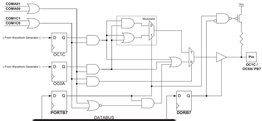
When the modulator is enabled the type of modulation (logical AND or OR) can be selected by the PORTB7 Register. When PORTB7=0, logical AND will be performed and when PORTB7=1, logical OR will be performed (see [Figure 16-3 on page 178](#)).
