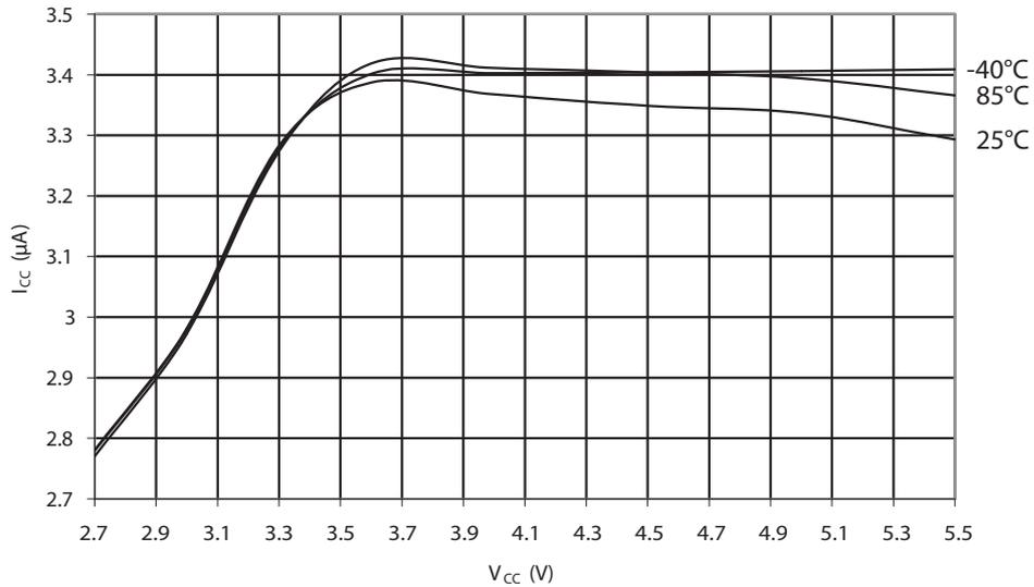
**Figure 30-40. USB Regulator Level with load 75Ω vs. V<sub>CC</sub>**
