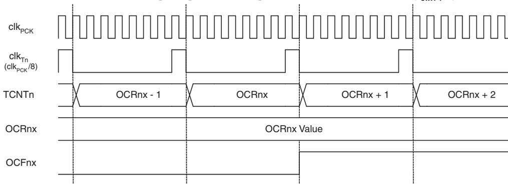
**Figure 15-19. Timer/Counter Timing Diagram, with Prescaler ( $f_{clkT4}/8$ )**
