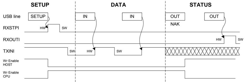
A NAK handshake is always generated at the first status stage command.
