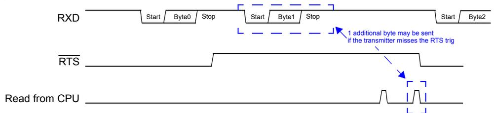
$\overline{\text{RTS}}$  will rise at 2/3 of the last received stop bit if the receive fifo is full.
