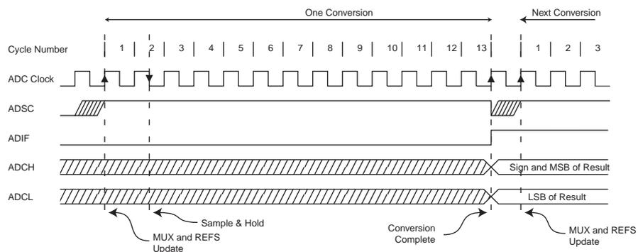
**Figure 24-6. ADC Timing Diagram, Auto Triggered Conversion**
