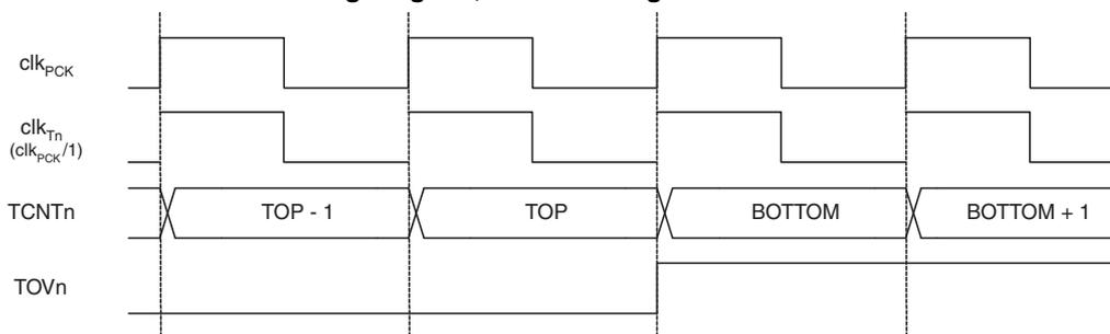
**Figure 15-17. Timer/Counter Timing Diagram, with Prescaler ( $f_{clkT4}/8$ )**
