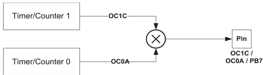
When the modulator is enabled, the two output compare channels are modulated together as shown in the block diagram (Figure 16-1).
