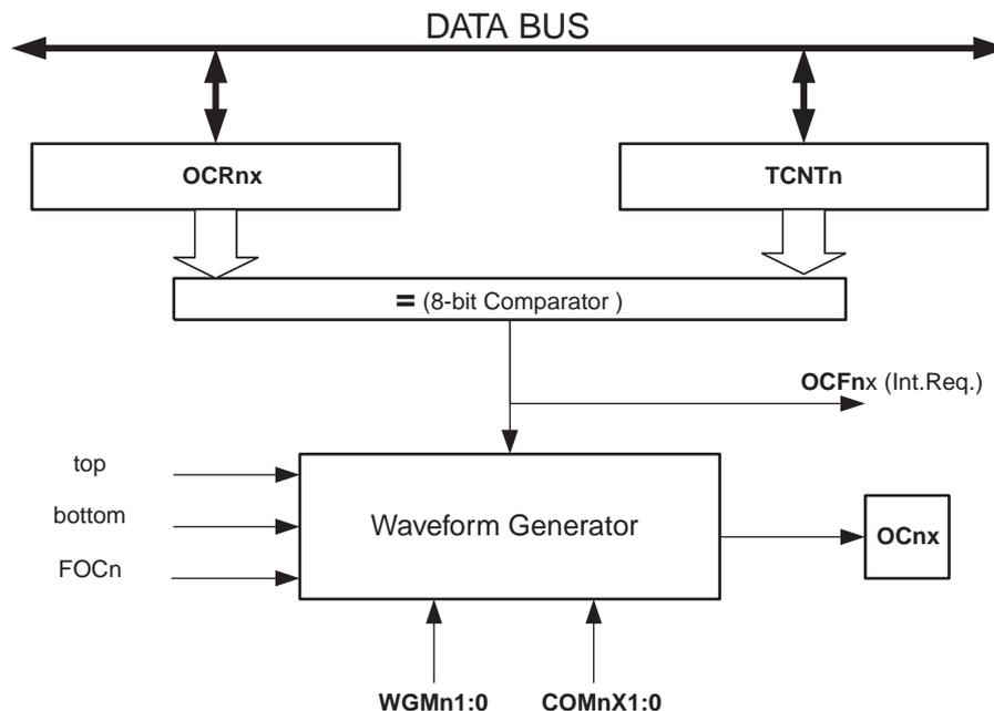
The OCR0x Registers are double buffered when using any of the Pulse Width Modulation (PWM) modes. For the normal and Clear Timer on Compare (CTC) modes of operation, the double buffering is disabled. The double buffering synchronizes the update of the OCR0x Compare Registers to either top or bottom of the
