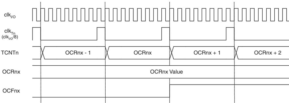
Figure 13-11 shows the setting of OCF0A and the clearing of TCNT0 in CTC mode and fast PWM mode where OCR0A is TOP.
