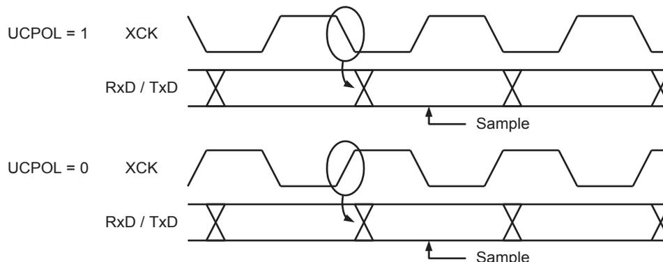
The UC POLn bit UCRSC selects which XCKn clock edge is used for data sampling and which is used for data change. As the above figure shows, when UC POLn is zero the data will be changed at rising XCKn edge and sampled at falling XCKn edge. If UC POLn is set, the data will be changed at falling XCKn edge and sampled at rising XCKn edge.
