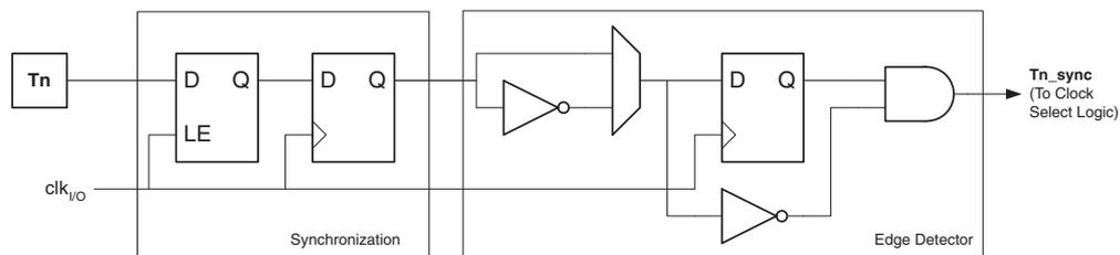
The synchronization and edge detector logic introduces a delay of 2.5 to 3.5 system clock cycles from an edge has been applied to the T<sub>n</sub> pin to the counter is updated.
