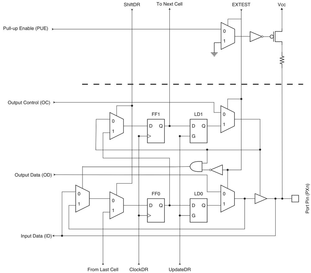
**Figure 26-4. General Port Pin Schematic Diagram**
