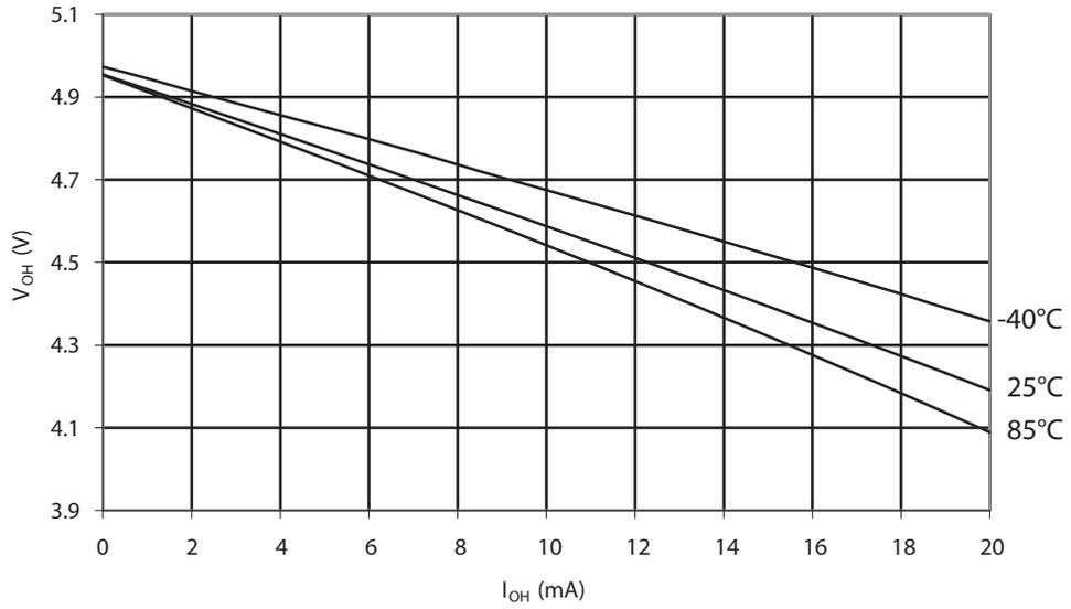
**Figure 30-21. USB DP LO Pull-Up Resistor Current vs. USB Pin Voltage**
