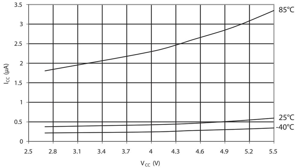
Figure 30-11. Power-Down Supply Current vs.  $V_{CC}$  (WDT Enabled)
