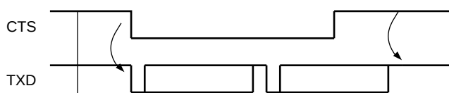
Figure 37-29. Transmitter Behavior when Operating with Hardware Handshaking
