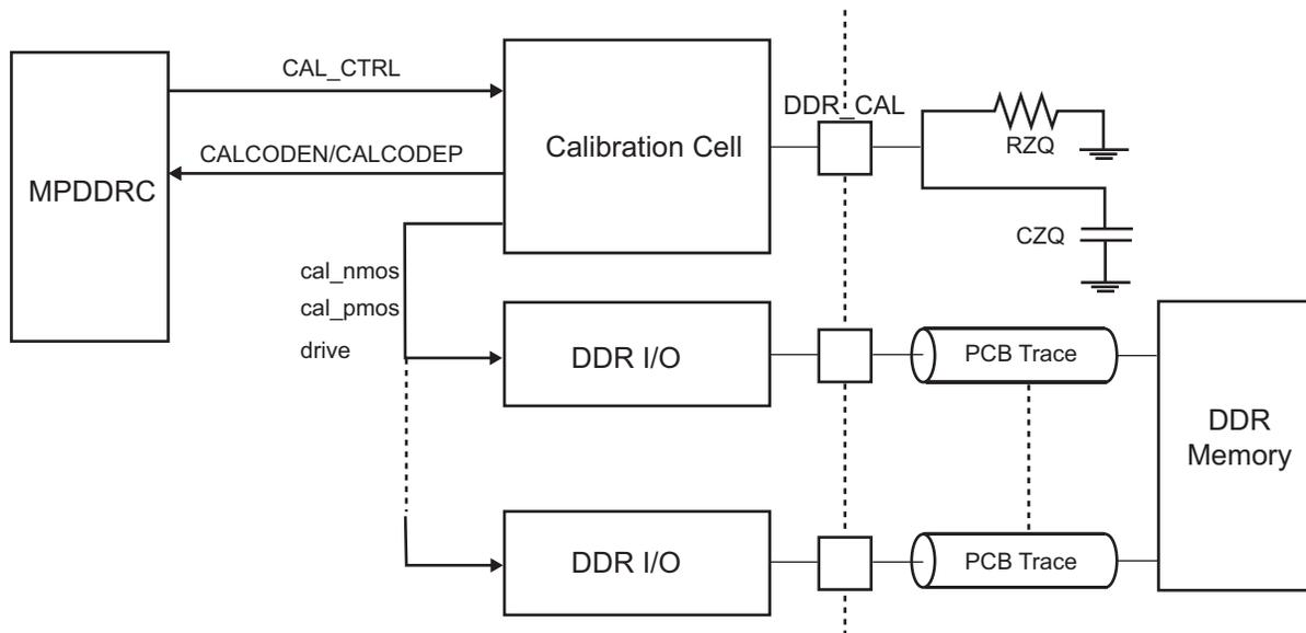
The calibration cell provides an input pin, DDR\_CAL, loaded with one of the following resistor RZQ values:
