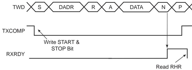
**Figure 47-89: Master Read with Multiple Data Bytes**
