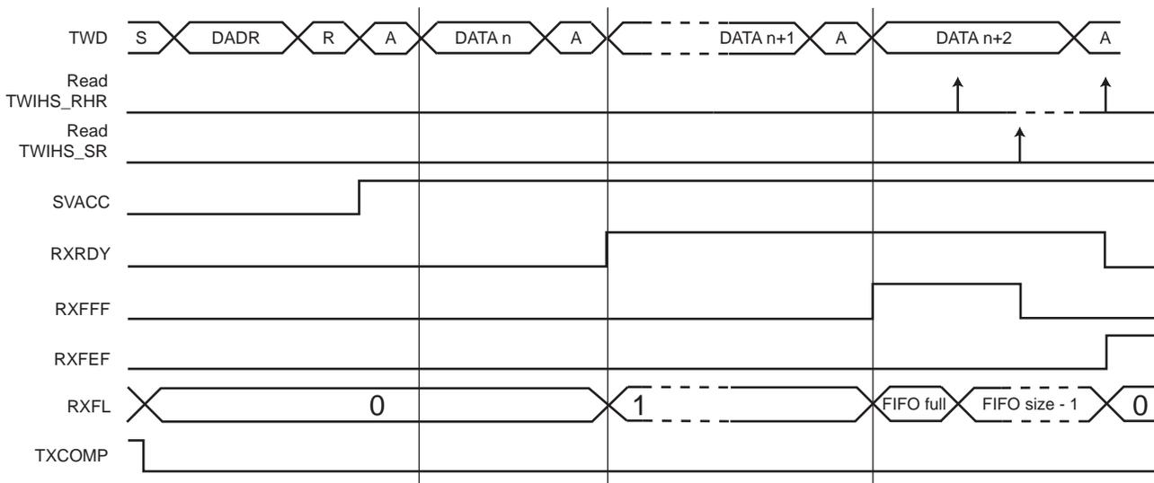
TXRDY and RXRDY behavior can be modified using the TXRDYM and RXRDYM fields in the TWIHS FIFO Mode Register (TWIHS\_FMR). In Single Data mode, there is no need to modify the TXRDY and RXRDY behavior; however, it may be useful in Multiple Data Mode.
