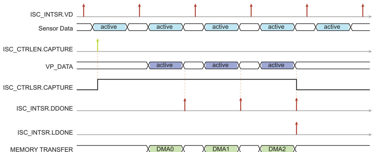
The linked list DMA transfer is terminated when an item of the list is programmed with the field ISC\_DCTRL.DE cleared or when the ISC\_DNDA.NDA field is equal to zero. This configuration also clears the ISC\_CTRLISR.CAPTURE field and sets the ISC\_INTSR.LDONE interrupt flag.
