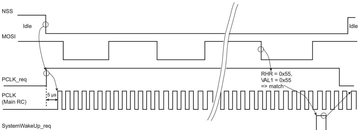
**Figure 49-15: Asynchronous Event Generating Only Partial Wakeup**
