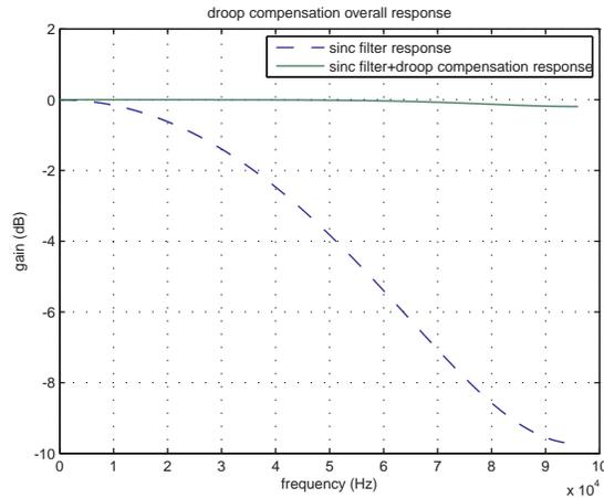
**Figure 55-6: Droop Compensation Filter 0 to 20 kHz Band Flatness**
