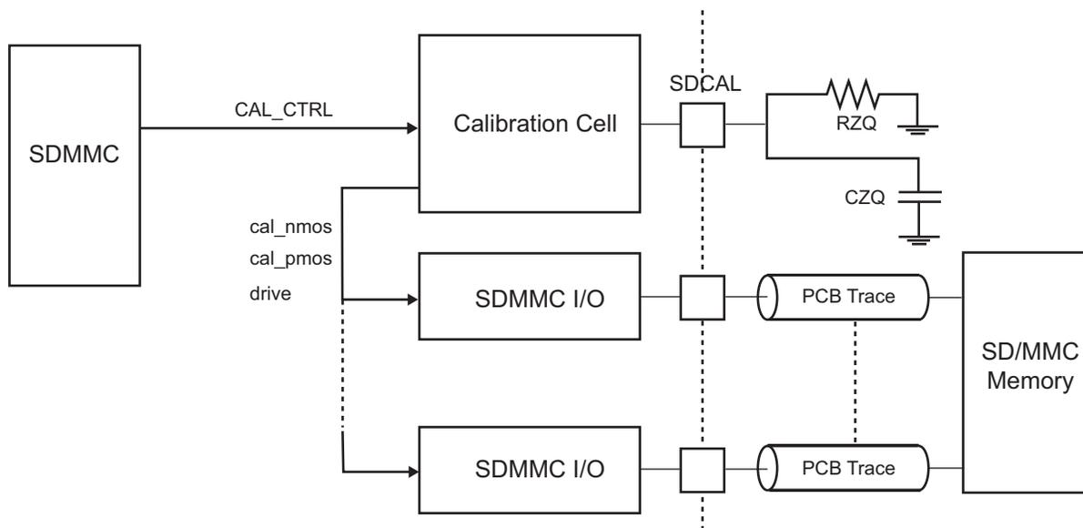
The calibration cell provides an input pin SDCAL loaded with a 20 K $\Omega$  resistor for 1.8V memories and a 16.9 K $\Omega$  resistor for 3.3V memories. According to the e.MMC specification, the output impedance calibration is mandatory for HS200 mode (1.8V) when it is not for other modes (3.3V).
