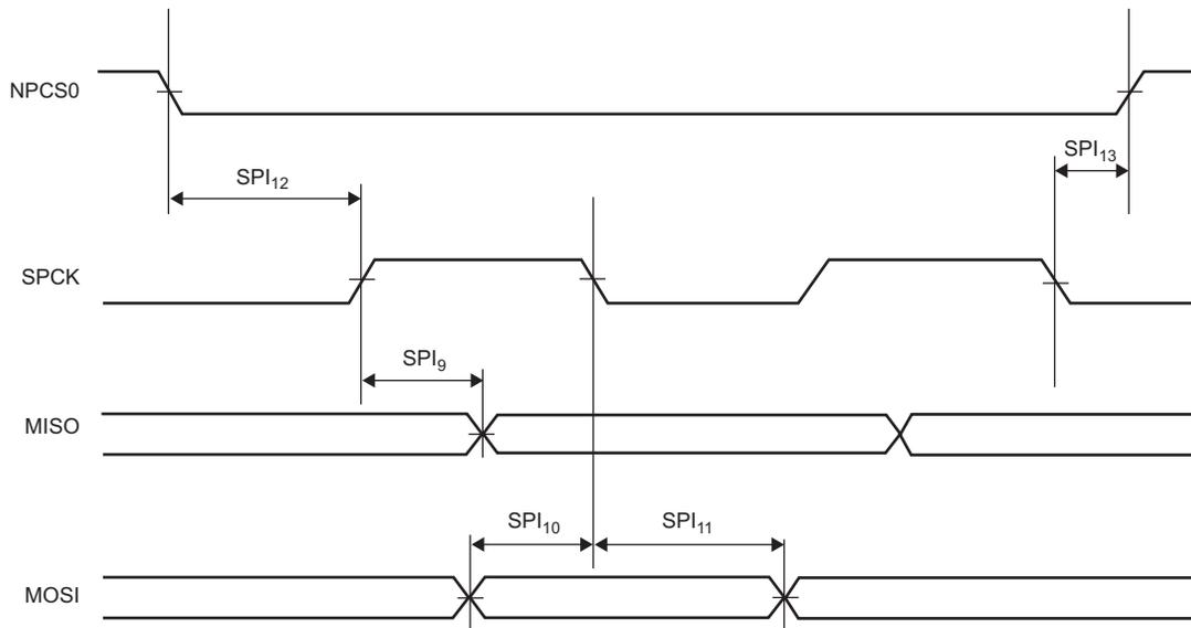
**Figure 66-23: SPI Slave Mode - NPCS Timings**
