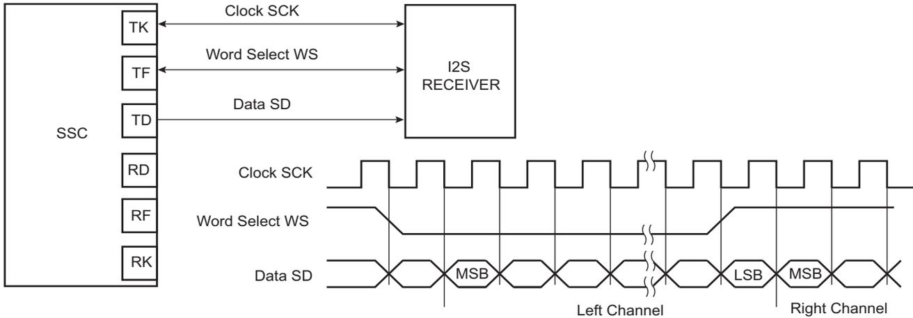
**Figure 45-4: Codec Application Block Diagram**
