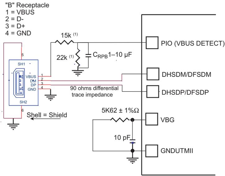
**Note 1:** The values shown on the 22 kΩ and 15 kΩ resistors are only valid with 3.3-V supplied PIOs.
