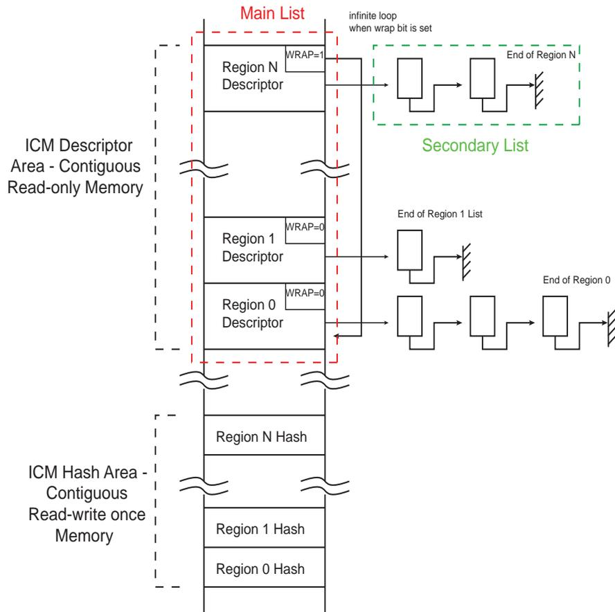
Each region descriptor supports gathering of data through the use of the Secondary List. Unlike the Main List, the Secondary List cannot modify the configuration attributes of the region. When the end of the Secondary List has been encountered, the ICM returns to the Main List. Memory integrity monitoring can be considered as a background service and the mandatory bandwidth shall be very limited. In order to limit the ICM memory bandwidth, use ICM\_CFG.BBC to control the ICM memory load.
