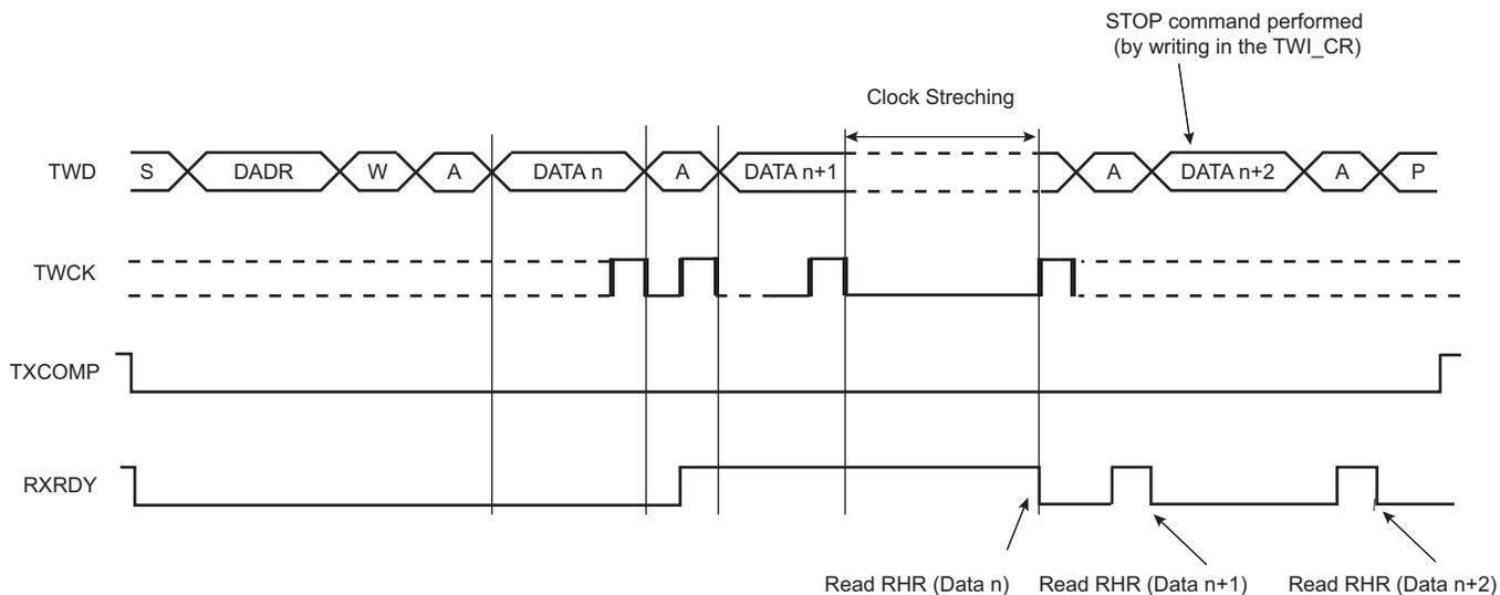
RXRDY is used as receive ready for the DMA receive channel.
