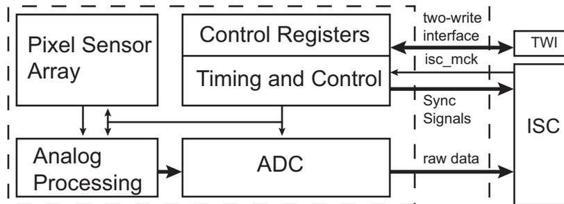
Figure 52-5: Raw Bayer Sensor with Embedded Image Processor
