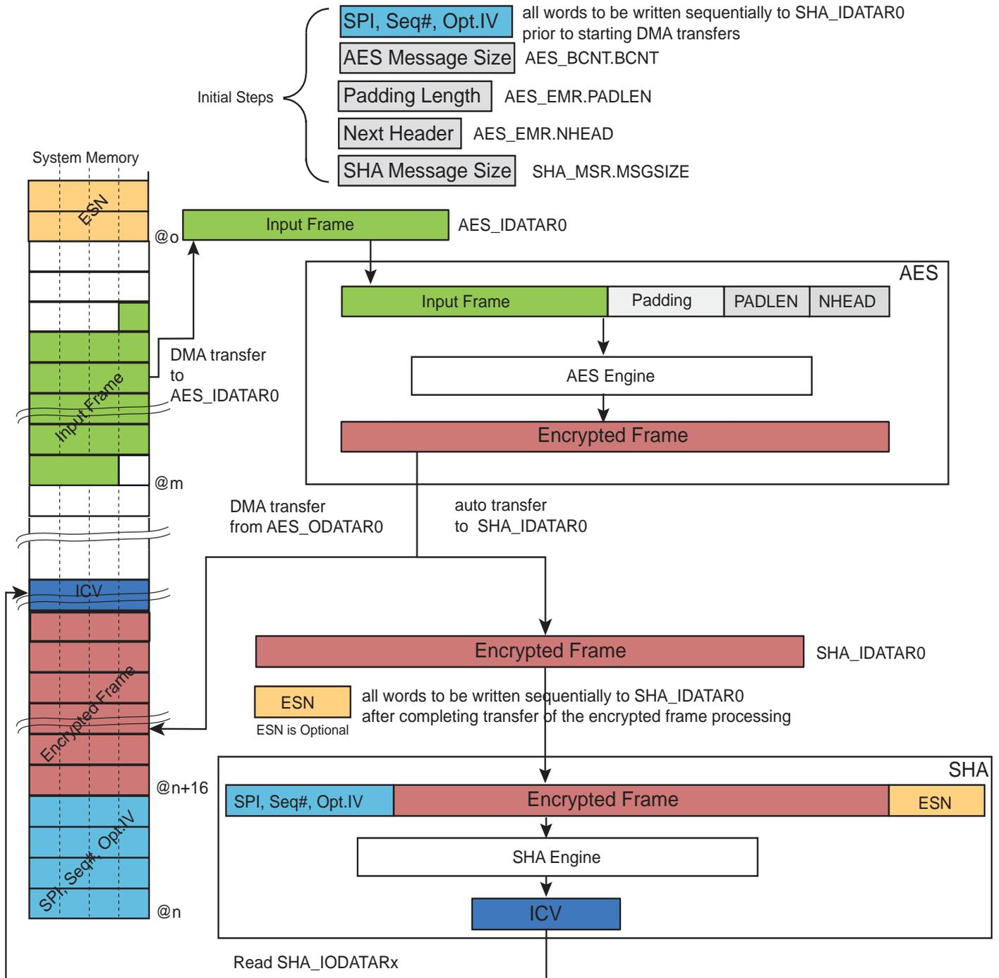
To decipher an ESP IPsec frame without the optional ESN trailer information, two DMA channels are required and the SHA must be configured in Automatic padding mode.
