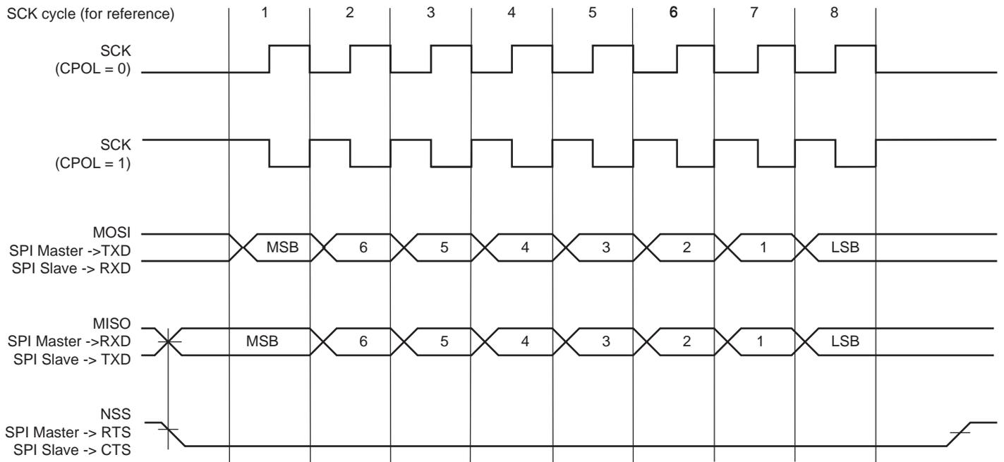
**Figure 47-40: SPI Transfer Format (CPHA = 0, 8 bits per transfer)**
