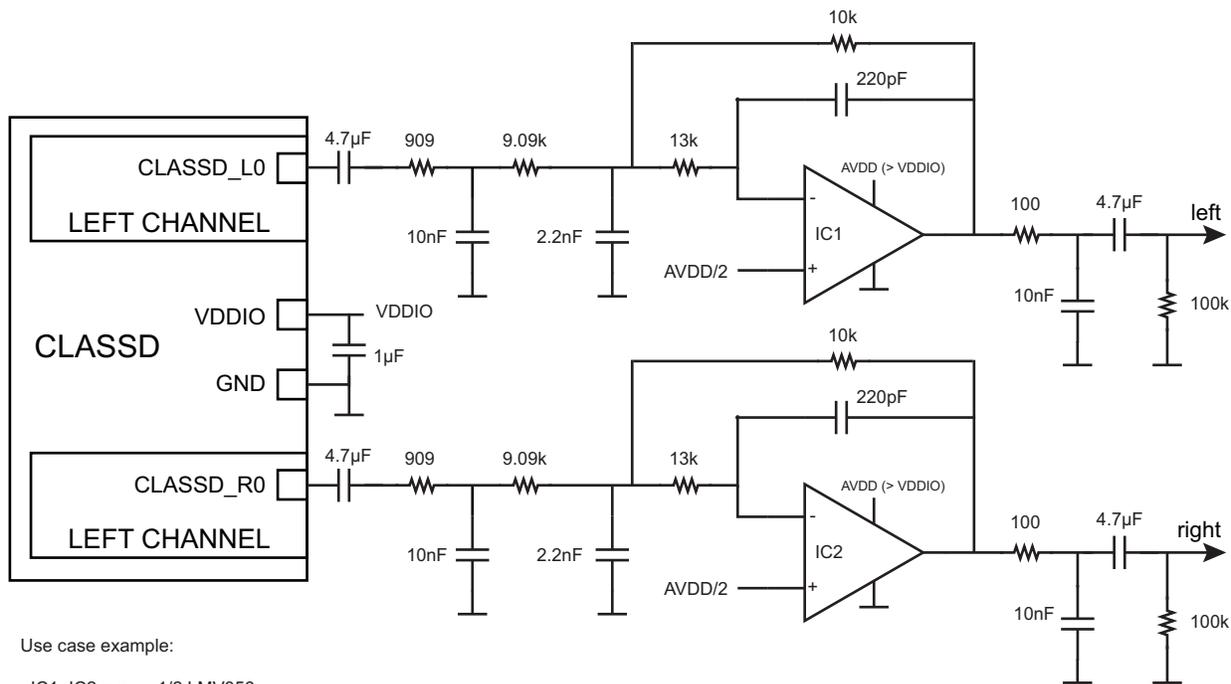
**Figure 43-21: Use Case 4B: Stereo Audio DAC With Passive Low Pass Filter and Single-ended Outputs**
