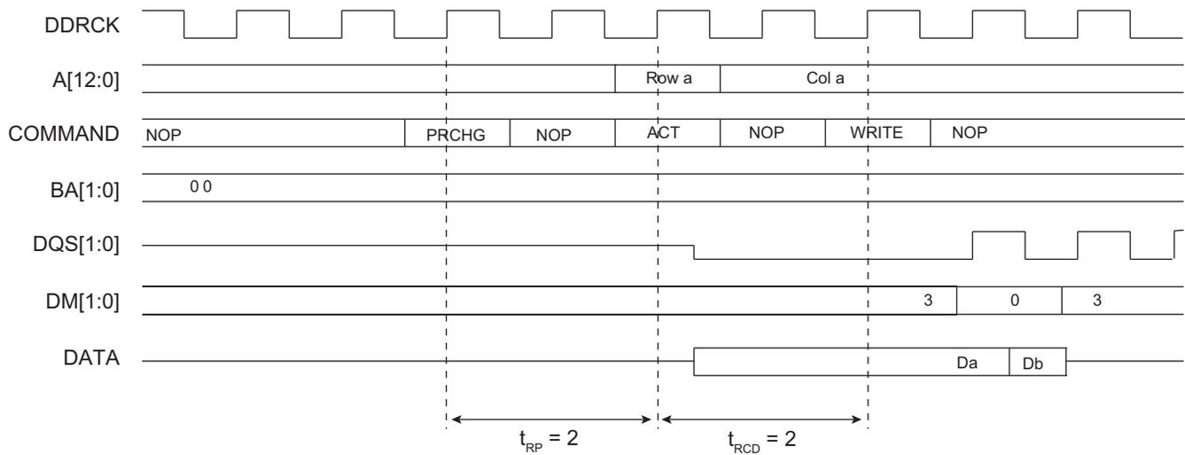
**Figure 36-3: Single Write Access, Row Closed, DDR2-SDRAM Devices**
