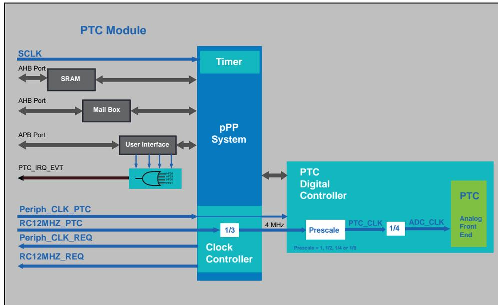
The RC12MHZ clock is internally divided by 3 in the PTC module, and so a 4 MHz clock is provided to the PTC digital controller. This controller can divide the clock further by 1, 1/2, 1/4 or 1/8 to slow down the PTC clock.
