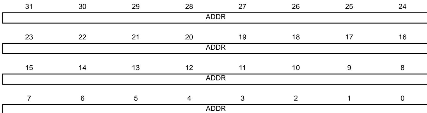
The unicast hash enable (UNIHEN) and the multicast hash enable (MITIHEN) bits in the [GMAC Network Configuration Register](#) enable the reception of hash matched frames. See [Section 40.6.9 "Hash Addressing"](#).
