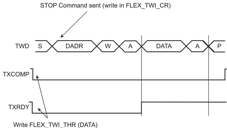
**Figure 47-86: Master Write with Multiple Data Bytes**
