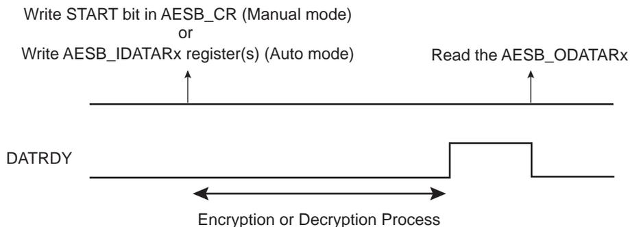
If the user does not want to read the output data registers between each encryption/decryption, the AESB\_ISR.DATRDY bit will not be cleared. If the AESB\_ISR.DATRDY bit is not cleared, the user cannot know the end of the following encryptions/decryptions.
