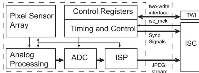
Figure 52-8: Serial CMOS Sensor with External Parallel Bridge
