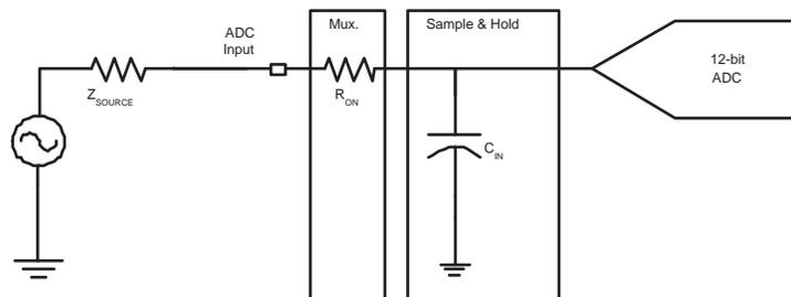
During the tracking phase, the ADC tracks the input signal during the tracking time shown below:
