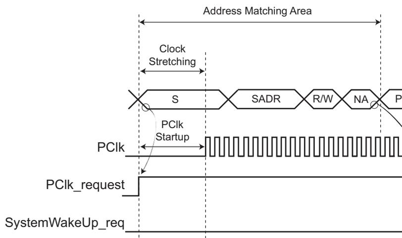
**Figure 46-46: Address Match and Data Match (Data Matching Enabled)**
