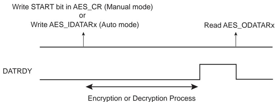
If the user does not want to read AES\_ODATARx between each encryption/decryption, the DATRDY flag will not be cleared. If the DATRDY flag is not cleared, the user cannot know the end of the following encryptions/decryptions.
