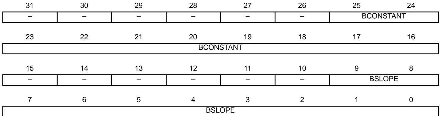
**BSLOPE:** Blue Color Slope for Piecewise Interpolation (signed 10 bits 1:3:6)
