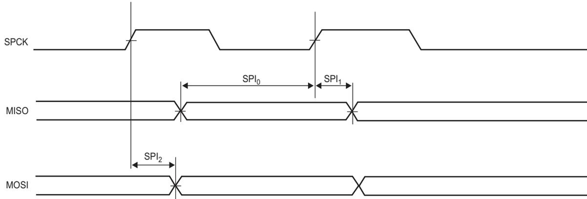
Figure 66-13: FLEXCOM in SPI Master Modes 0 and 3
