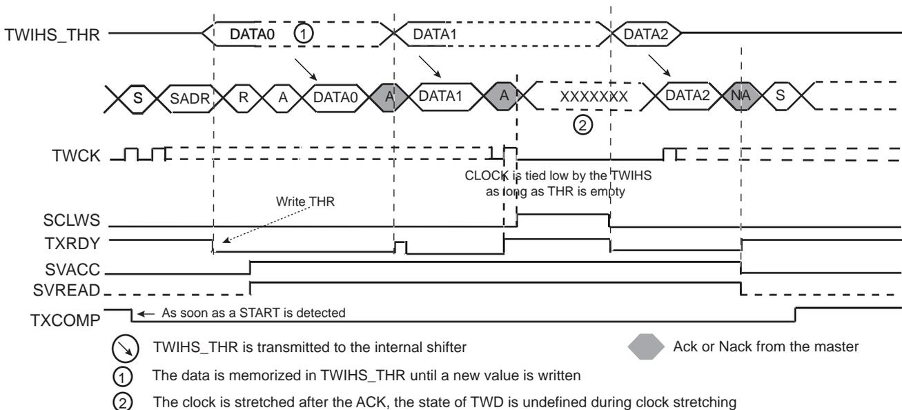
**Note 1:** TXRDY is reset when data has been written in the TWIHS\_THR to the internal shifter and set when this data has been acknowledged or non acknowledged.
