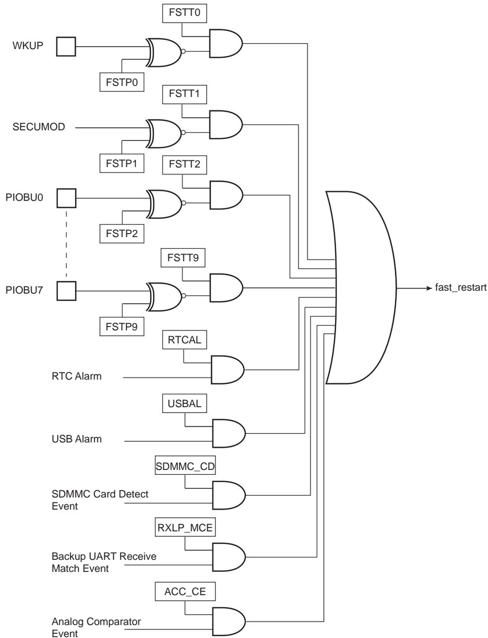
The PMC user interface does not provide the source of the fast startup, but the user can recover this information by reading the PIO Controller and the status registers of the RTC, ACC, RXLP, and USB Controller.
