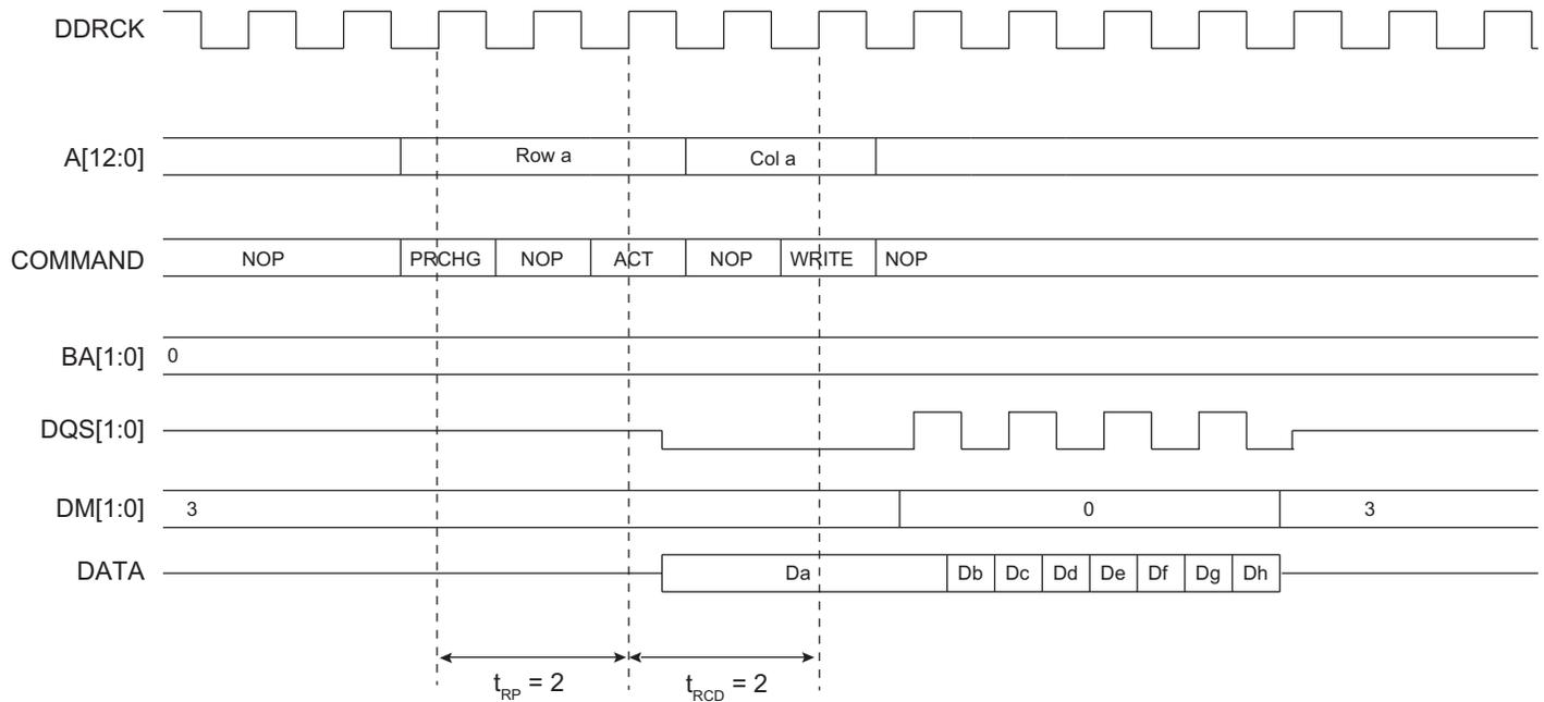
**Figure 36-5: Burst Write Access, Row Closed, DDR2-SDRAM Devices**
