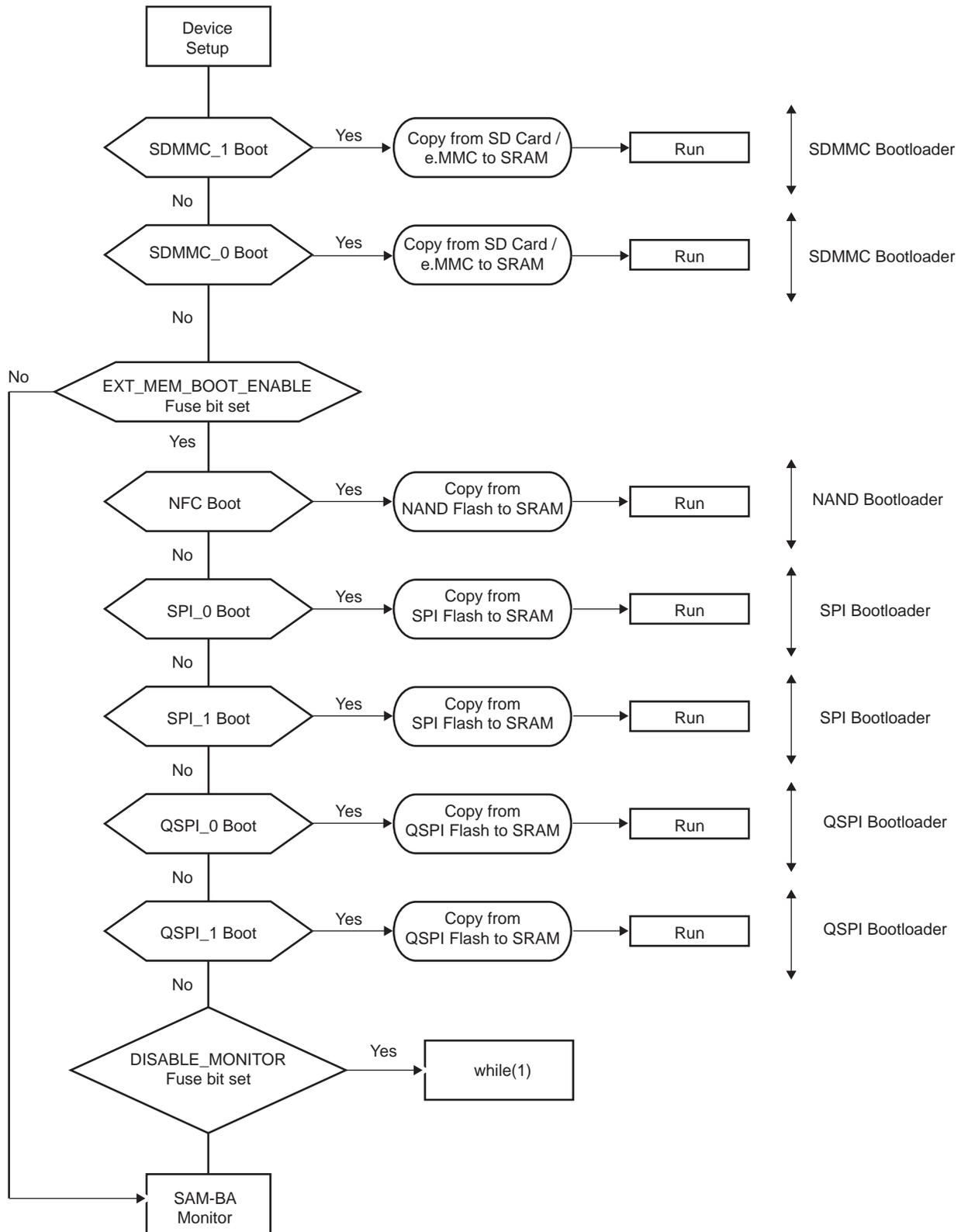
Figure 16-5: NVM Boot Diagram
