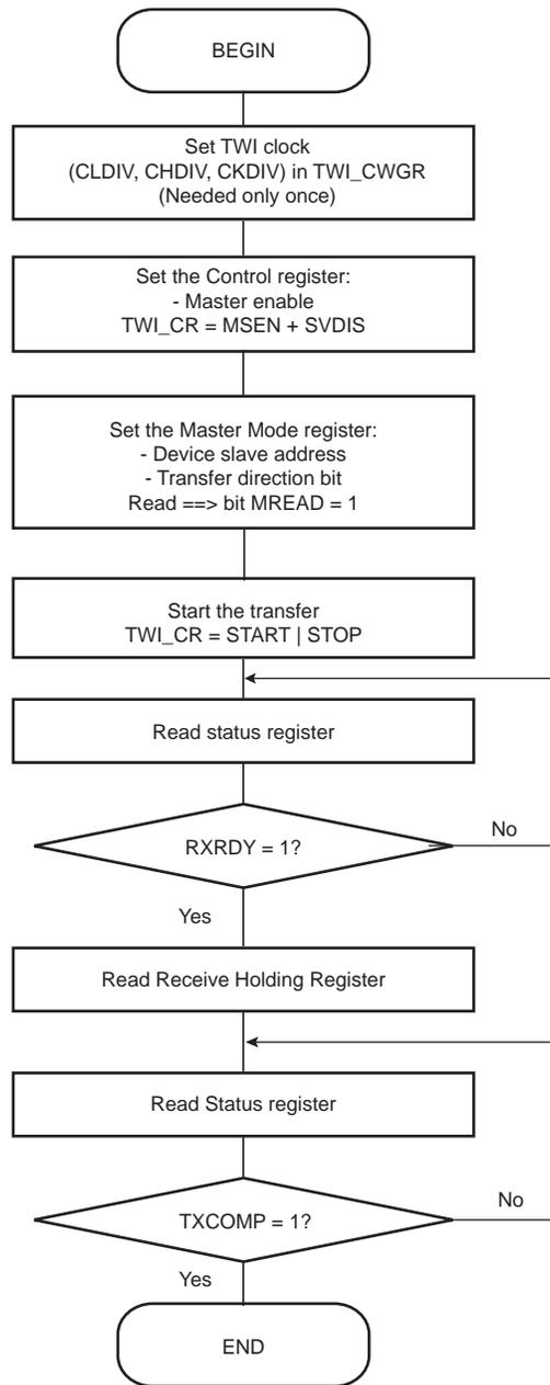
Figure 46-22: TWIHS Read Operation with Single Data Byte and Internal Address
