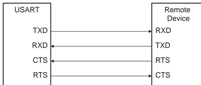
Setting the USART to operate with hardware handshaking is performed by writing the FLEX\_US\_MR.USART\_MODE field to the value 0x2.
