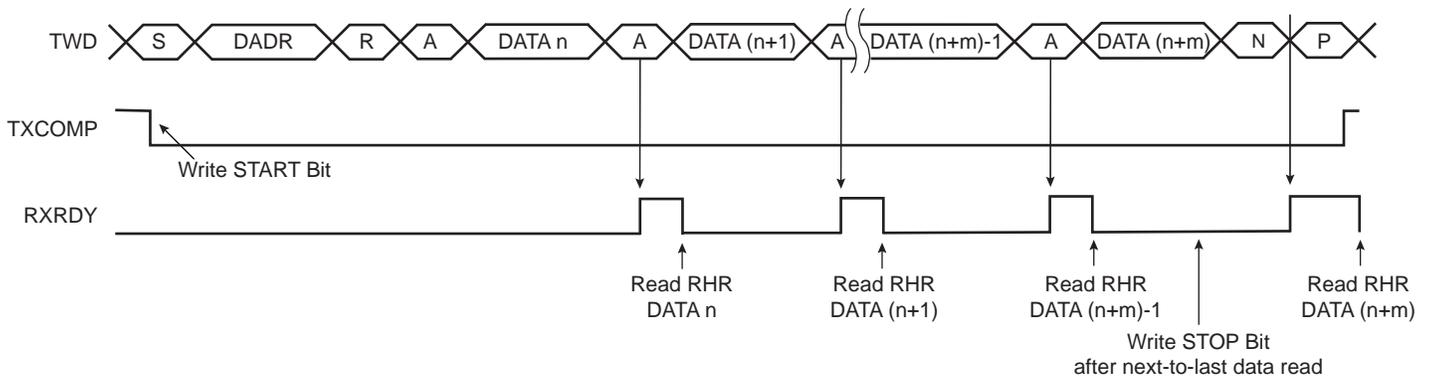
**Figure 47-90: Master Read Clock Stretching with Multiple Data Bytes**
