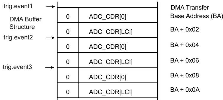
If the last channel is driven by a device with a slower variation compared to other channels (temperature sensor for example), the channel can be enabled/disabled at any time. However, this may not be optimal for downstream processing.
