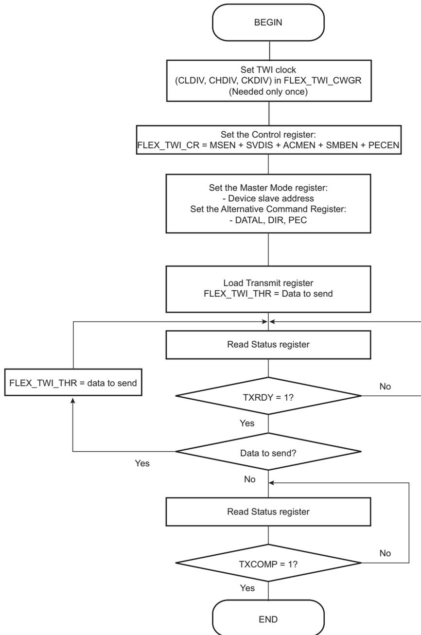
Figure 47-100: TWI Write Operation with Multiple Data Bytes and Read Operation with Multiple Data Bytes (Sr)
