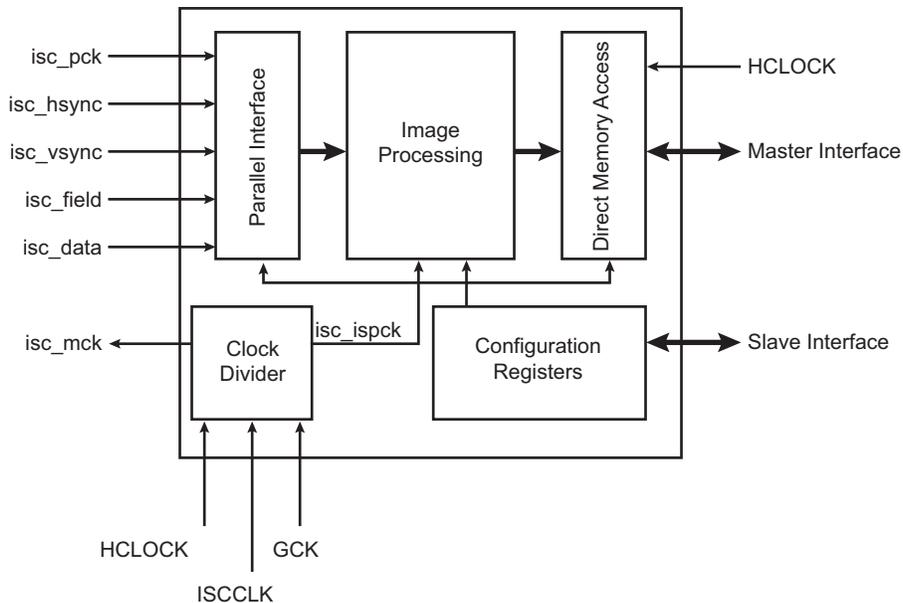
Figure 52-2: Image Sensor Controller Raw Bayer Signal Processor
