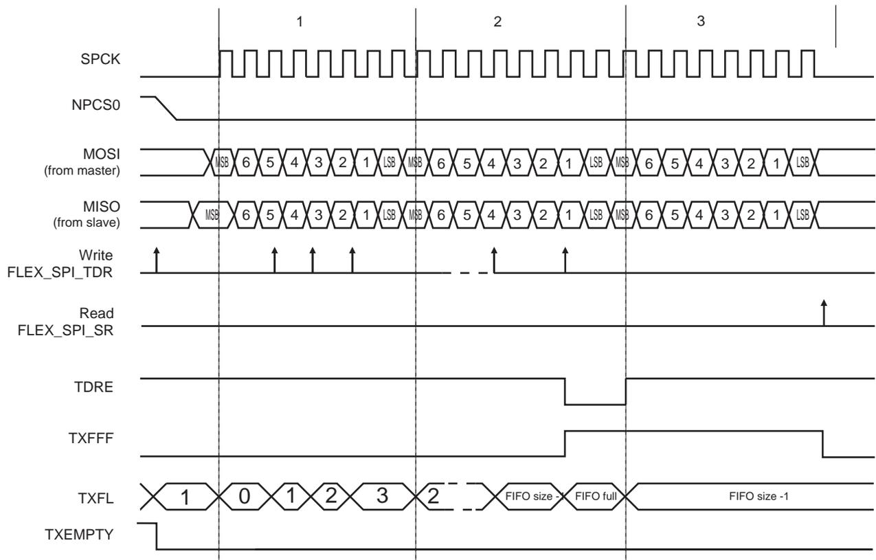
**Figure 47-82: RDRF in Single Data Mode and RXRDYM = 0**
