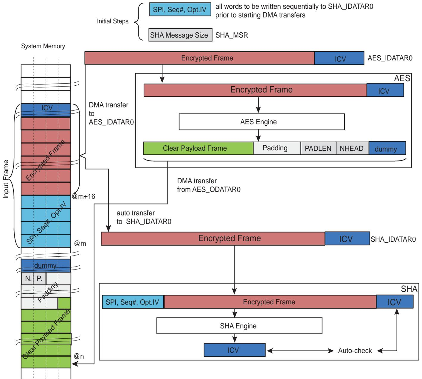
Figure 60-15: Decryption of an ESP IPsec Frame with ESN
