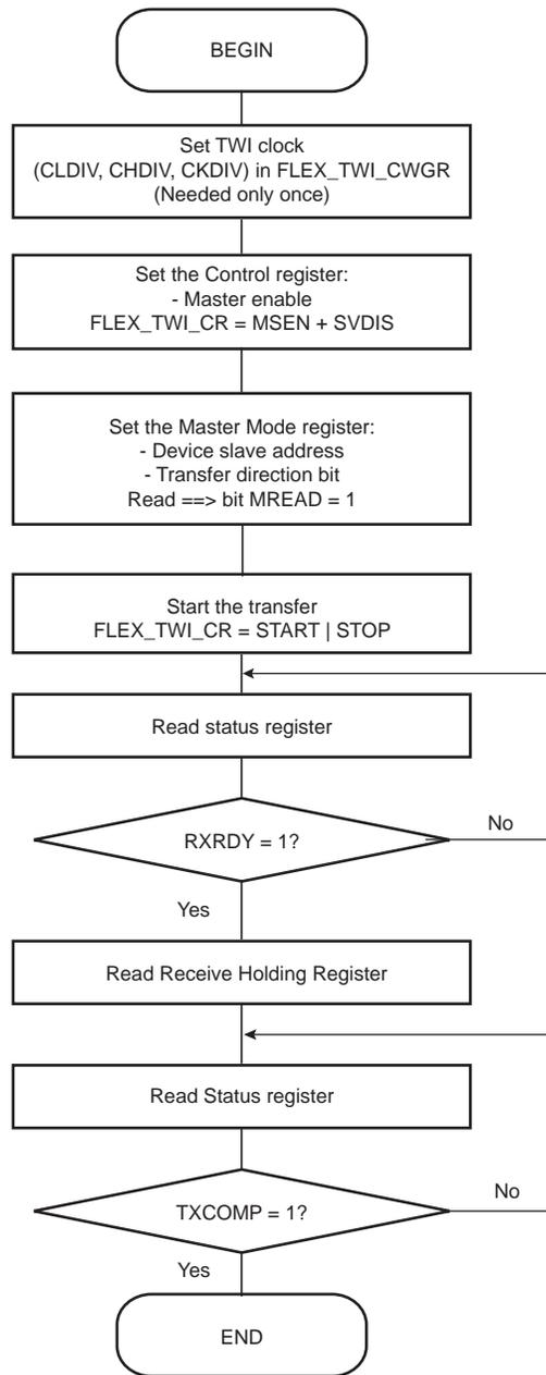
Figure 47-103: TWI Read Operation with Single Data Byte and Internal Address
