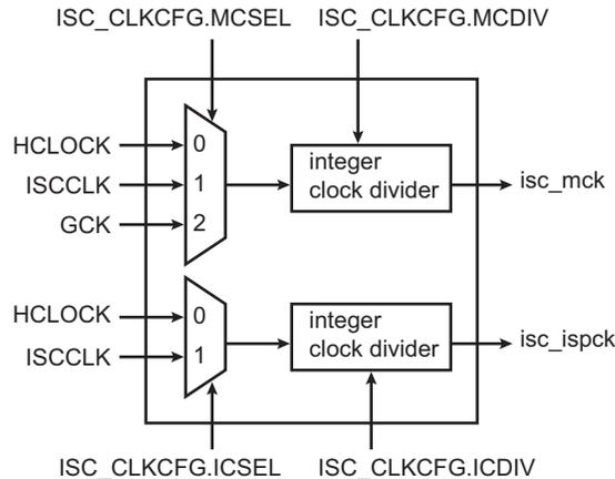
The ISC digital pipeline requires internally a functional clock named `isc_ispck`. This clock is also fully programmable. This `isc_ispck` is enabled using the `ISC_CLKEN.ICEN` field. This clock is mandatory for ISC operation. The ISC module is designed to accept input signals that are asynchronous to the `isc_ispck`. Synchronization is done internally as long as the following relationship holds:
