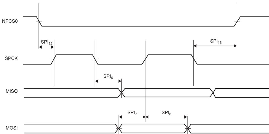
**Figure 66-15: FLEXCOM in SPI Slave Modes 1 and 2**
