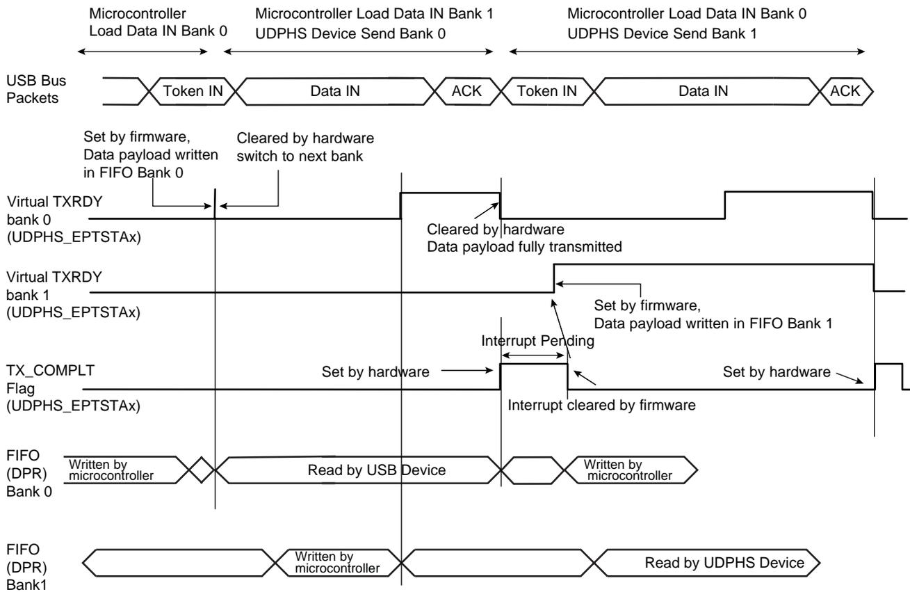
**Figure 41-11: Data IN Followed By Status OUT Transfer at the End of a Control Transfer**
