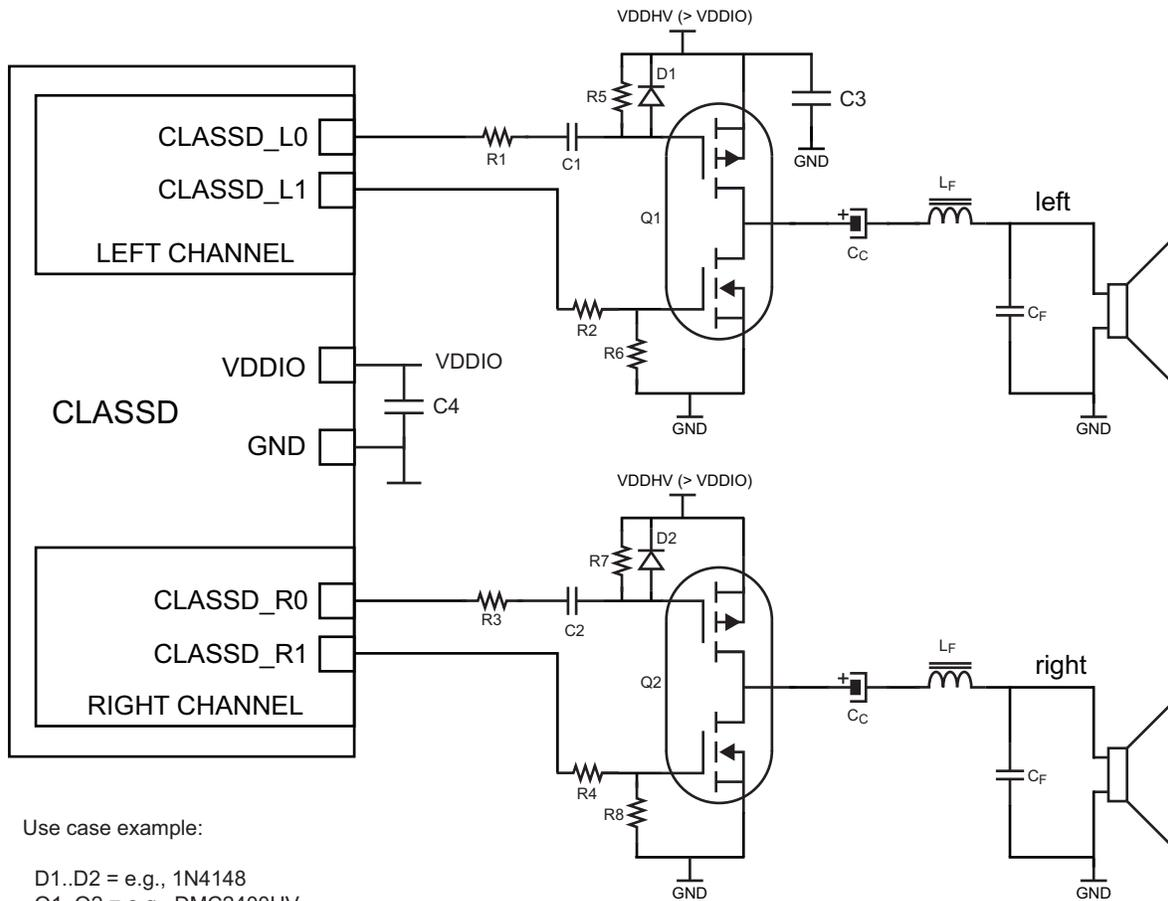
In the Use Case 2 application schematic, the drive network of the MOSFETs gates follows the principles described in Use Case 1.
