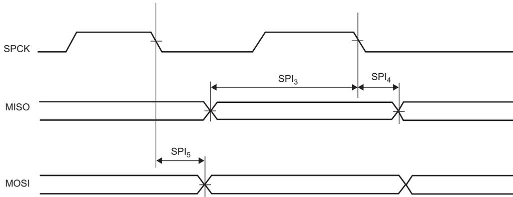
Figure 66-14: FLEXCOM in SPI Slave Modes 0 and 3
