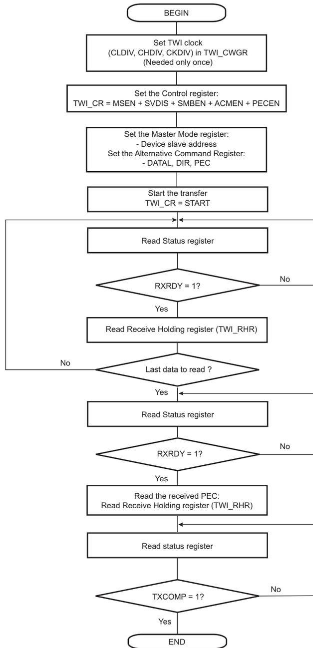
Figure 46-26: TWIHS Read Operation with Multiple Data Bytes + Write Operation with Multiple Data Bytes (Sr)
