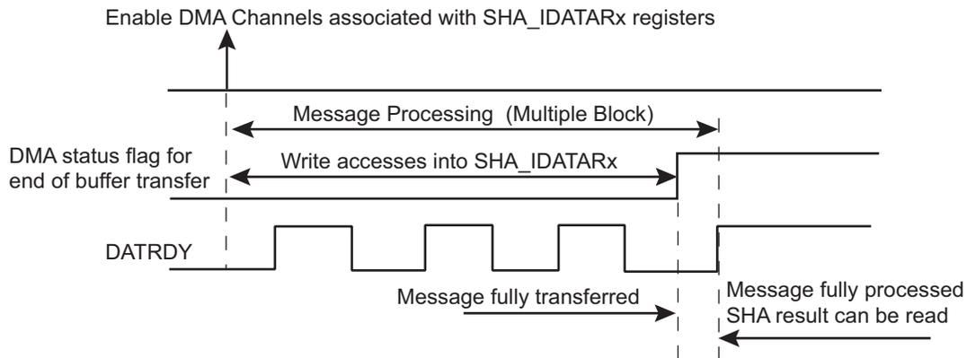
**Figure 61-4: interrupts Processing with DMA and Automatic Padding**
