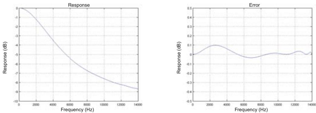
**Figure 43-9: De-emphasis Filter: Frequency Response & Error (f<sub>s</sub> = 44.1 kHz)**
