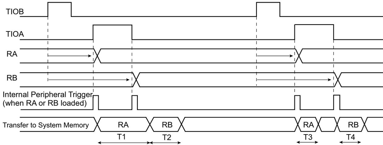
T1,T2,T3,T4 = System Bus load dependent ( $t_{\min} = 8$  Peripheral Clocks)
