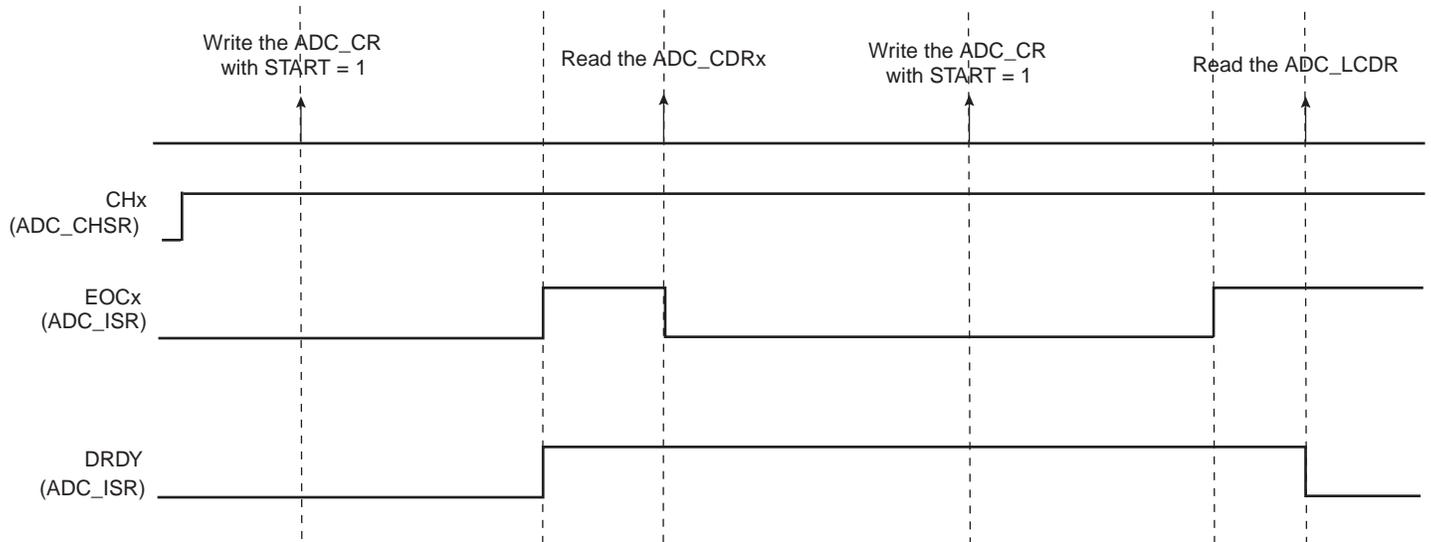
If ADC\_CDR is not read before further incoming data is converted, the corresponding OVREx flag is set in the Overrun Status register (ADC\_OVER).
