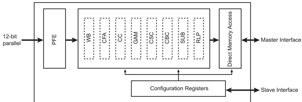
The ISC video pipeline integrates the following submodules:
