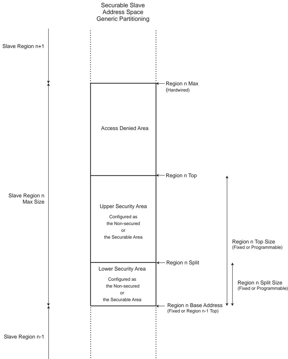
A set of Bus Matrix security registers allows to specify, for each AHB slave, slave security region or slave security area, the security mode required to access this slave, slave security region or slave security area.
