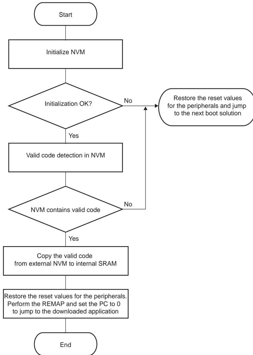
The NVM bootloader program first initializes the PIOs related to the NVM device. Then it configures the right peripheral depending on the NVM and tries to access this memory. If the initialization fails, it restores the reset values for the PIO and the peripheral, and then tries to fulfill the same operations on the next NVM of the sequence.
