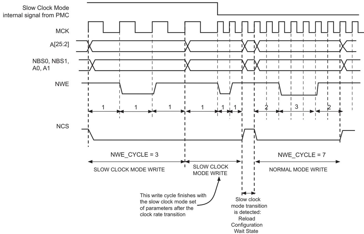
**Figure 37-30: Recommended Procedure to Switch from Slow Clock Mode to Normal Mode or from Normal Mode to Slow Clock Mode**
