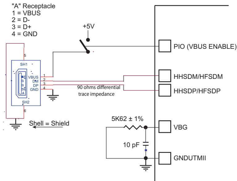
**3:** Typical USB High Speed Device connection, refer to [Section 41. “USB High Speed Device Port \(UDPHS\)”](#).
