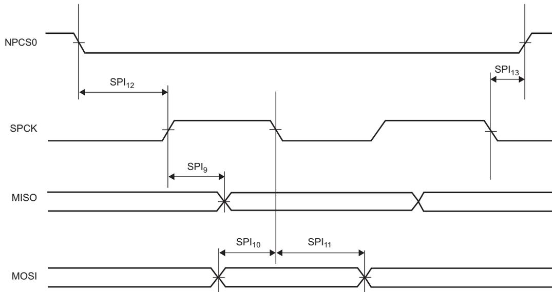
**Figure 66-16: FLEXCOM in SPI Slave Mode - NPCS Timings**
