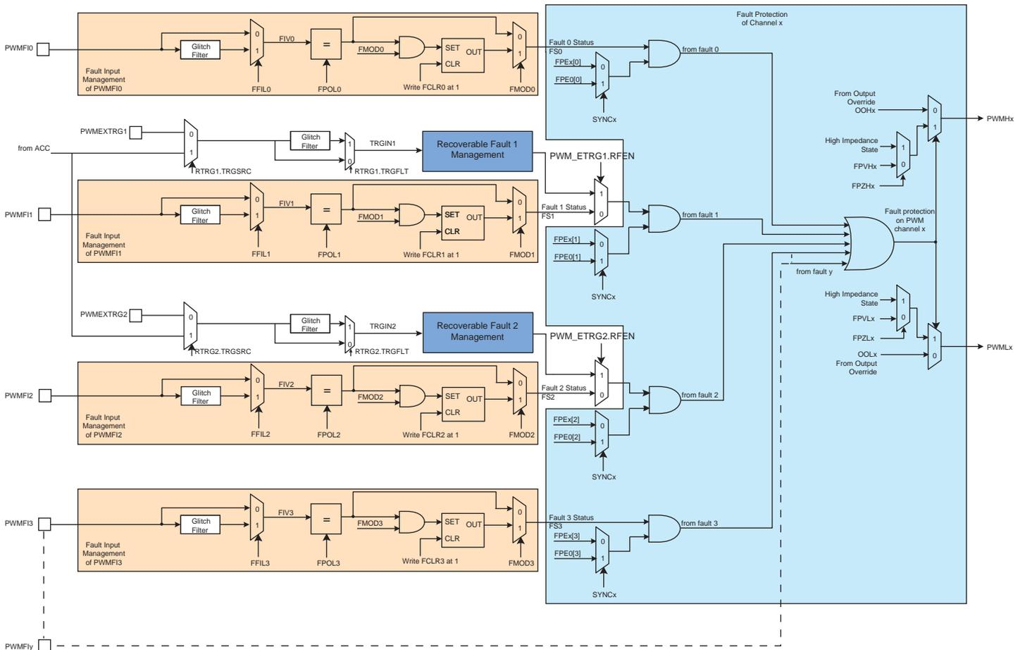
The polarity level of the fault inputs is configured by the FPOL field in the [PWM Fault Mode Register \(PWM\\_FMR\)](#). For fault inputs coming from internal peripherals such as ADC or Timer Counter, the polarity level must be FPOL = 1. For fault inputs coming from external GPIO pins the polarity level depends on the user's implementation.
