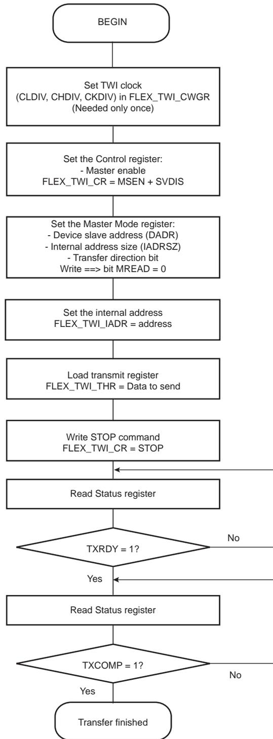
Figure 47-97: TWI Write Operation with Multiple Data Bytes with or without Internal Address
