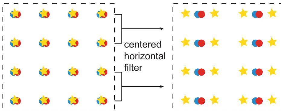
The SUB422 module performs luminance and chrominance packing. When the line length is odd, the missing luminance is a copy of the last but one luminance. It also means that the final dma stream written to memory is equal to the original horizontal size plus one when the line length is odd.
