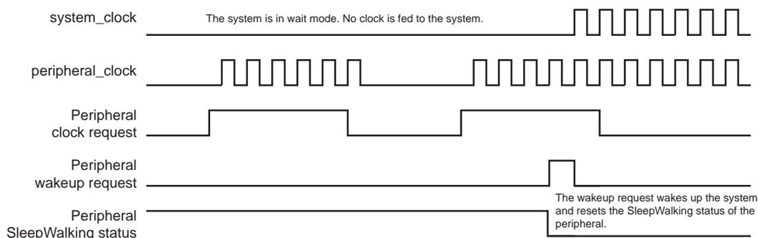
When the system is in Active mode, peripherals enabled for asynchronous partial wakeup have their respective clocks stopped until the peripherals request a clock. When a peripheral requests the clock, the PMC provides the clock without CPU intervention.
