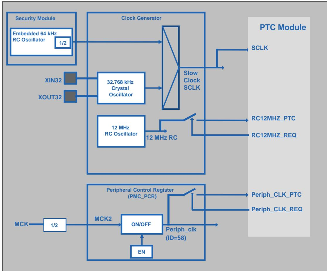
The PTC module operates both from a peripheral clock synchronous to the master clock of the system and from an asynchronous clock source directly connected to the embedded 12 MHz RC oscillator. The selected clocks must be enabled in the PMC before they can be used by the PTC. By default, the 12 MHz RC oscillator is enabled at startup of the product.
