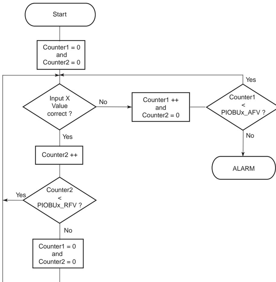
At reset state, the debouncers are not activated (PIOBU\_AFV and PIOBU\_RFV fields set to 0), which implies that no alarm can be generated.
