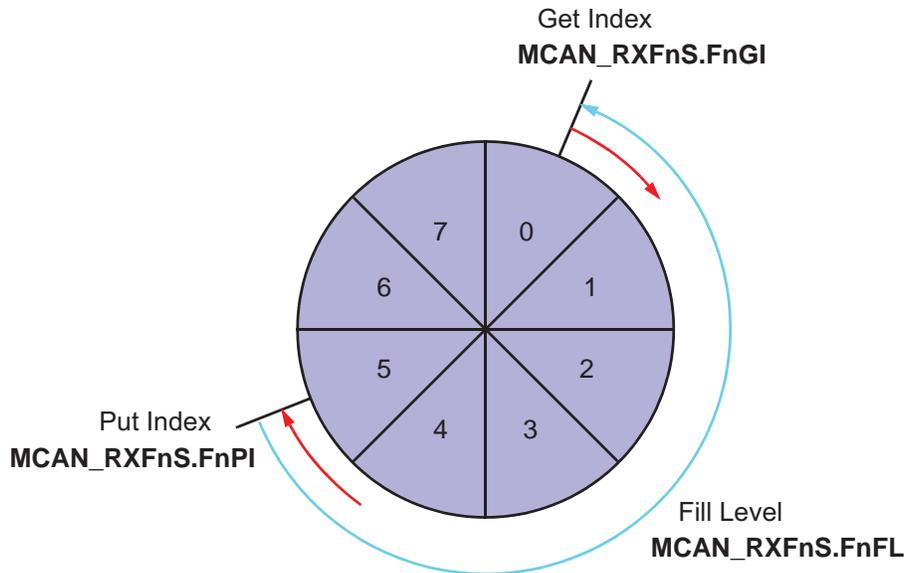
When reading from an Rx FIFO, Rx FIFO Get Index MCAN\_RXFnS.FnGI x FIFO Element Size has to be added to the corresponding Rx FIFO start address MCAN\_RXFnC.FnSA.
