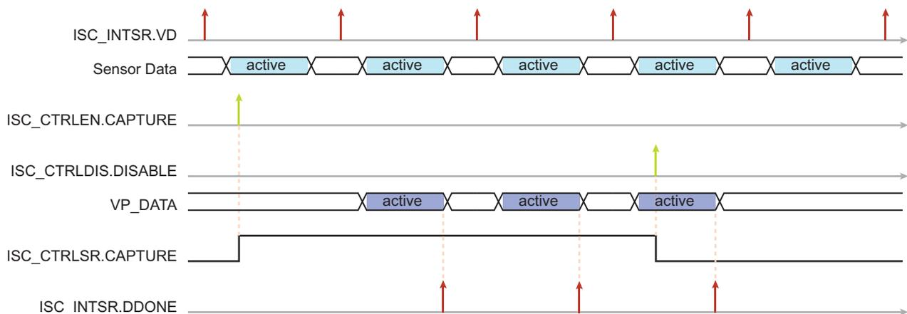
When Continuous Acquisition mode is activated (ISC\_PFE\_CFG0.CONT is set), the data transfer terminates when either a DMA end of list is reached, a software disable is performed or a software reset is activated. The ISC\_INTSR.DDONE is set at the end of the DMA data transfer.
