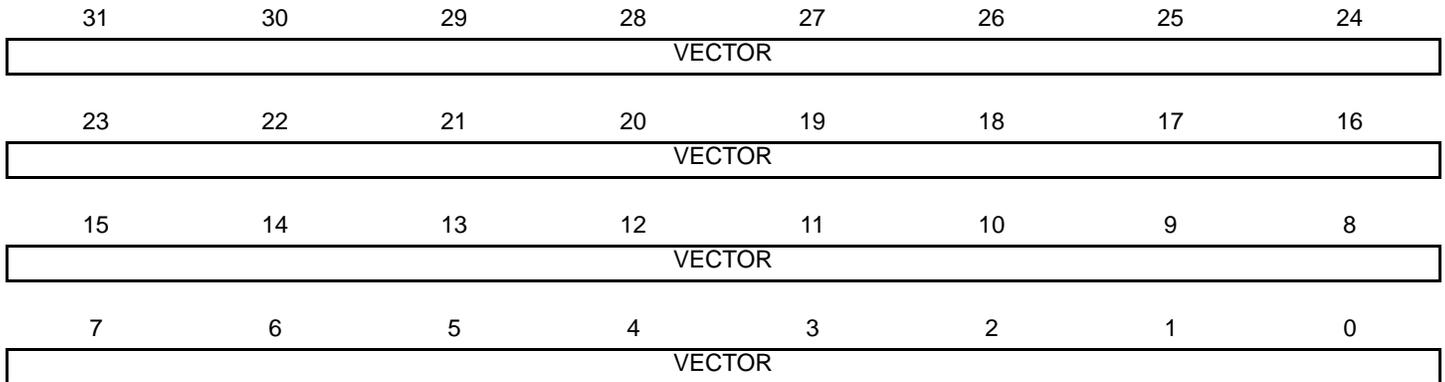
This register can only be written if the WPEN bit is cleared in the [AIC Write Protection Mode Register](#).
