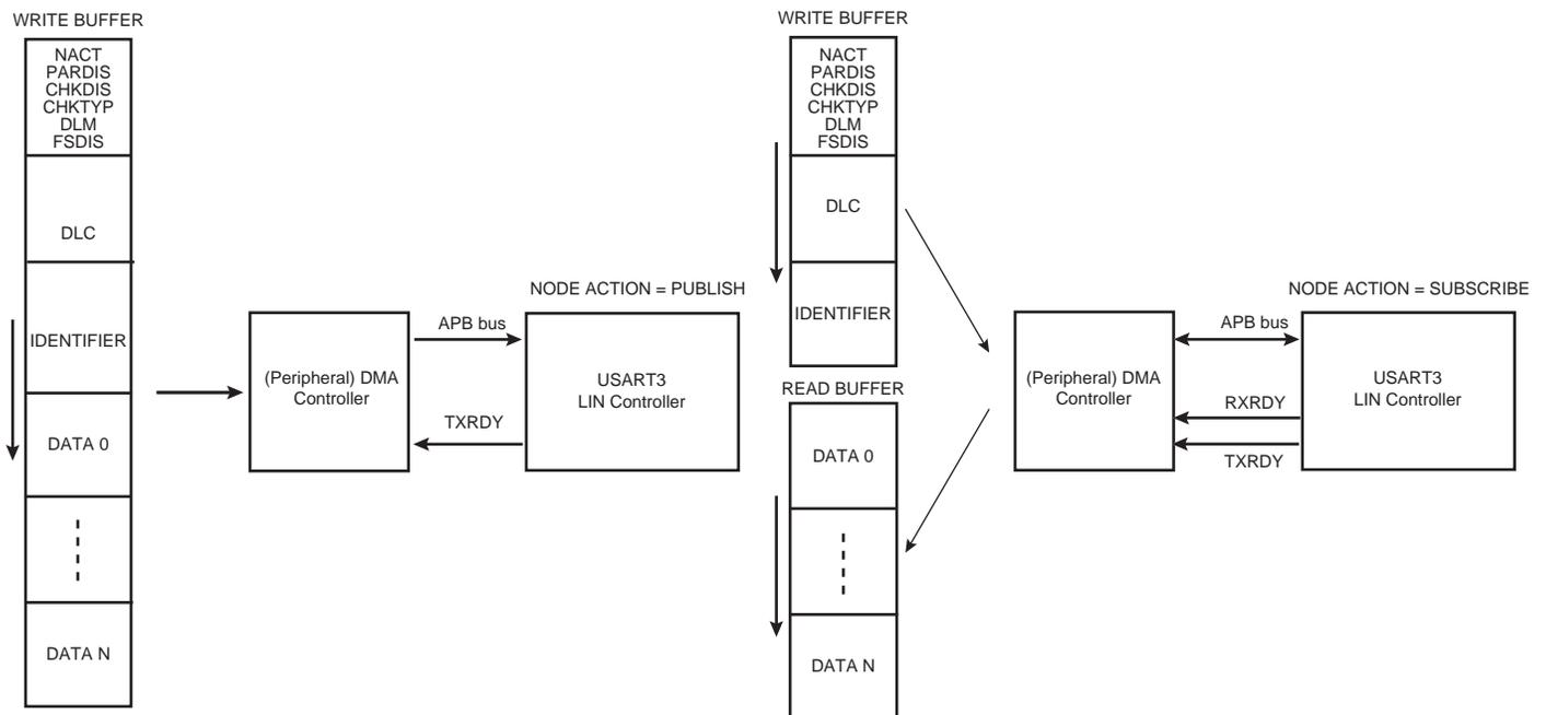
**Figure 47-54: Master Node with DMAC (PDCM = 0)**
