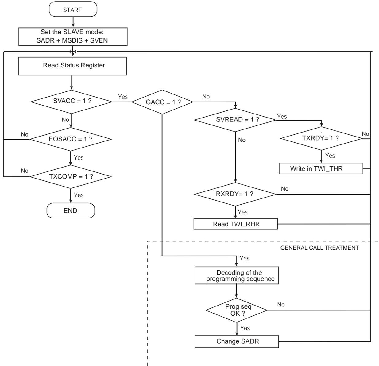
**Figure 46-49: Read Write Flowchart in Slave Mode with SMBus PEC**
