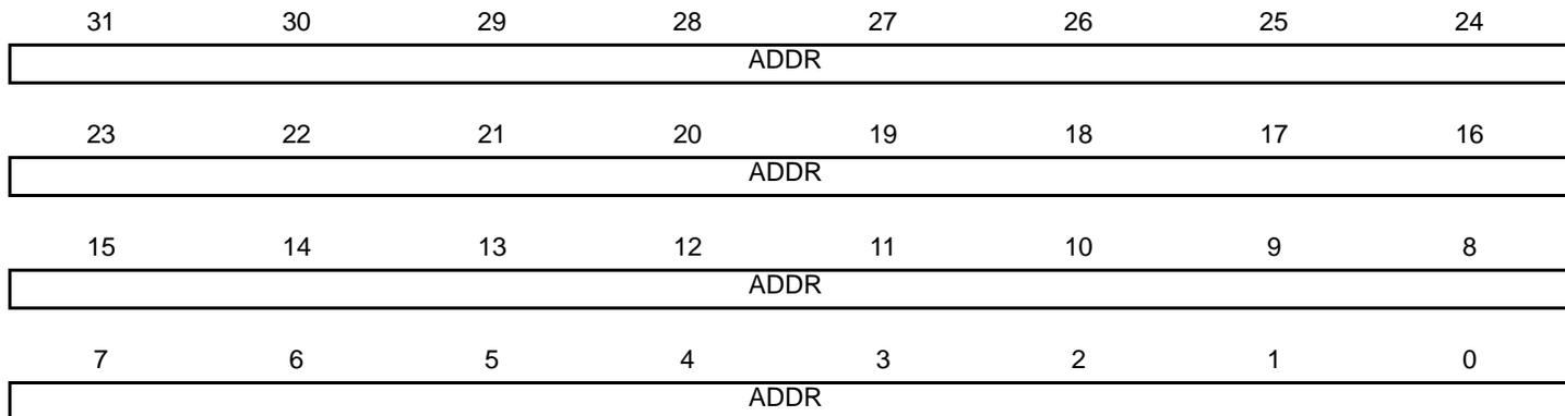
**ADDR: DMA Transfer Overlay 1 Address**
