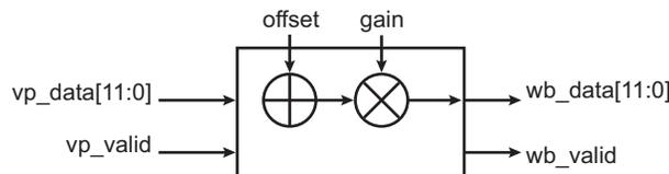
There are four {gain, offset} sets for each Bayer component. The output value is clipped.
