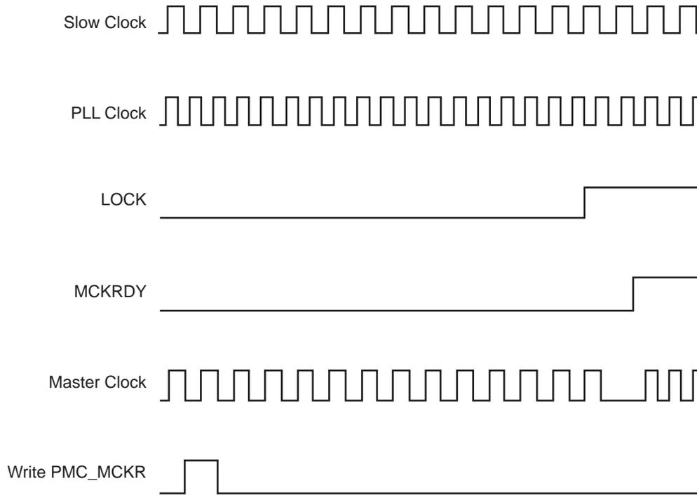
**Figure 33-12: Switch Master Clock from Main Clock to Slow Clock**
