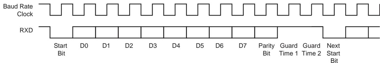
**Figure 47-32: T = 0 Protocol with Parity Error**
