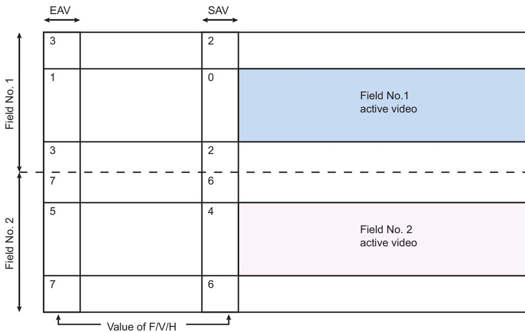
**Figure 52-13: Frame Timing Relationship for Progressive Systems**
