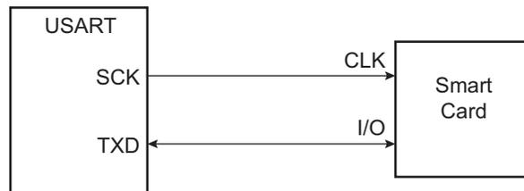
When operating in ISO7816, either in T = 0 or T = 1 modes, the character format is fixed. The configuration is 8 data bits, even parity and 1 or 2 stop bits, regardless of the values programmed in the CHRL, MODE9, PAR and CHMODE fields. MSBF can be used to transmit LSB or MSB first. Parity Bit (PAR) can be used to transmit in Normal or Inverse mode. See [Section 47.10.6 "USART Mode Register"](#) and [PAR: Parity Type](#).
