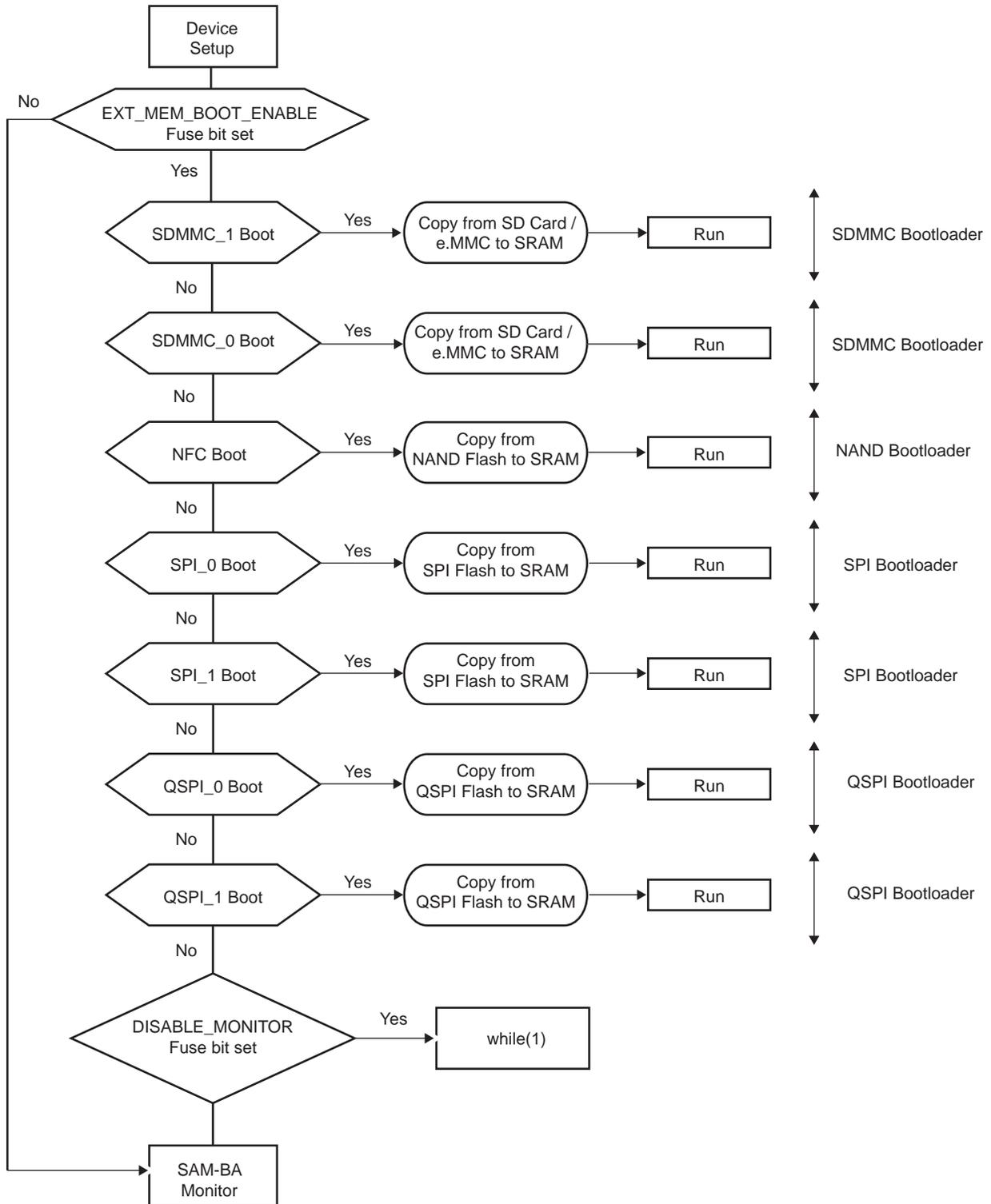
**Figure 16-4: NVM Bootloader Program Description for MRL C Parts**
