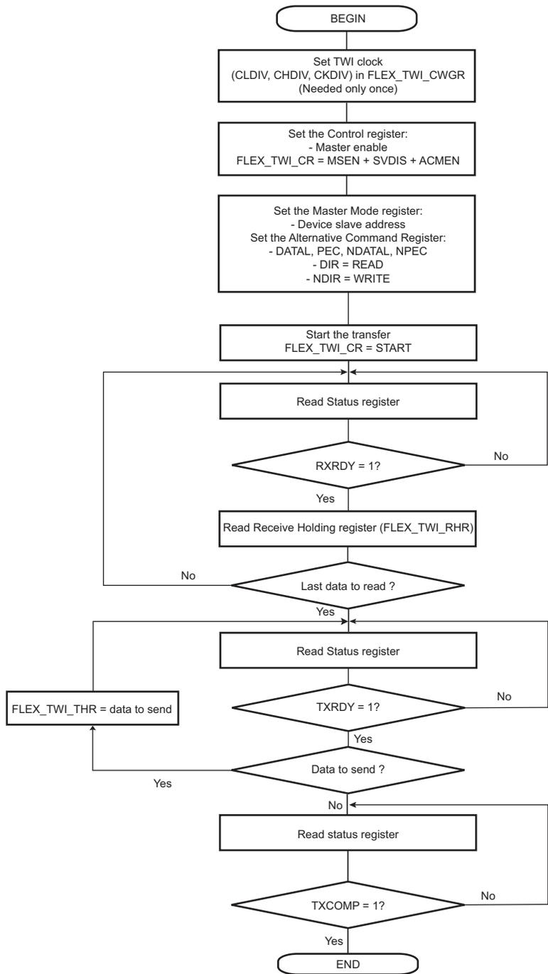
Figure 47-109: TWI Read Operation with Multiple Data Bytes + Write with Alternative Command Mode with PEC
