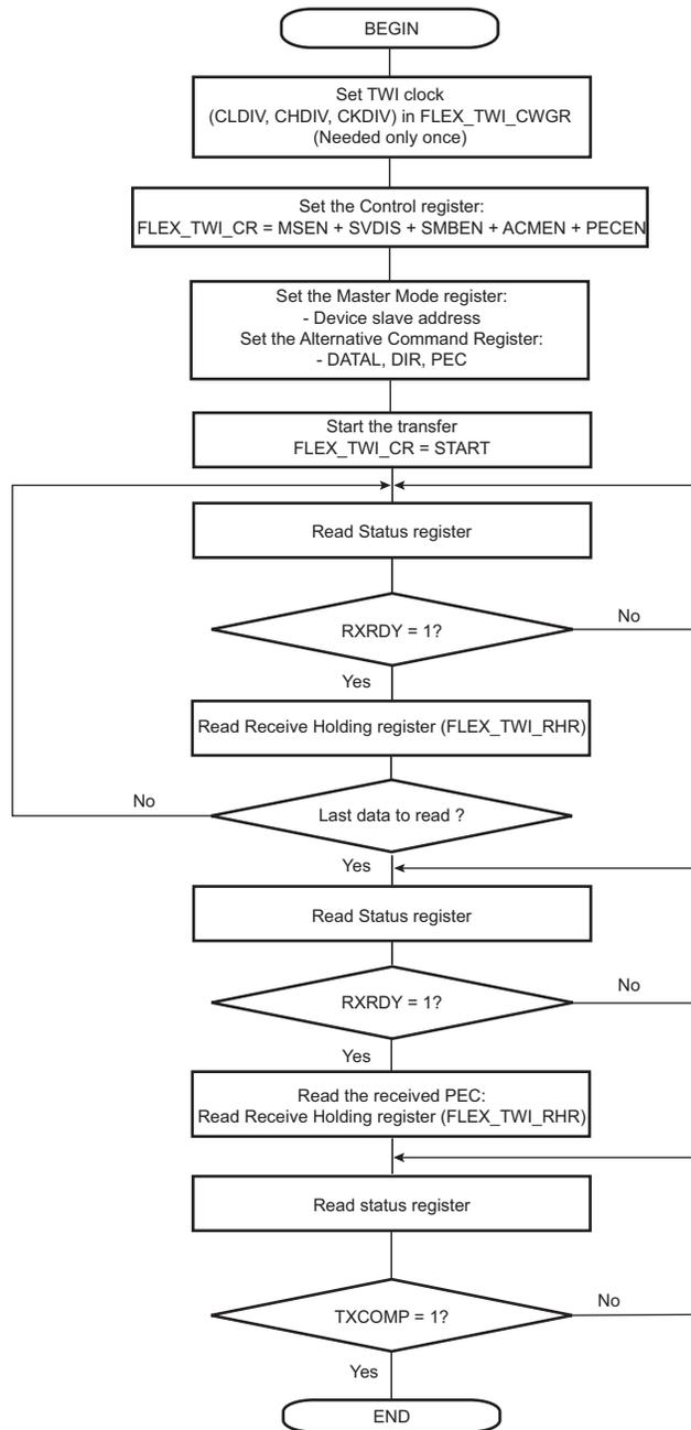
**Figure 47-107: TWI Read Operation with Multiple Data Bytes + Write Operation with Multiple Data Bytes (Sr)**
