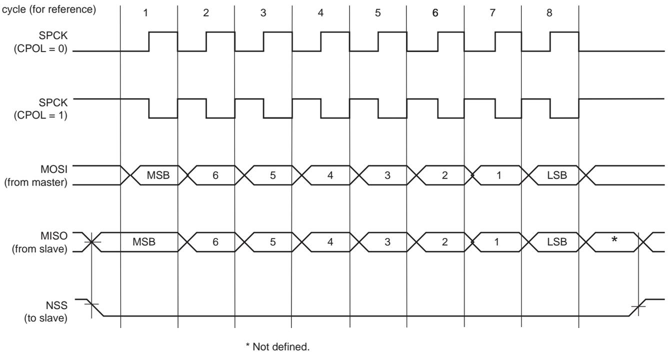
**Figure 47-66: SPI Transfer Format (NCPHA = 0, 8 bits per transfer)**
