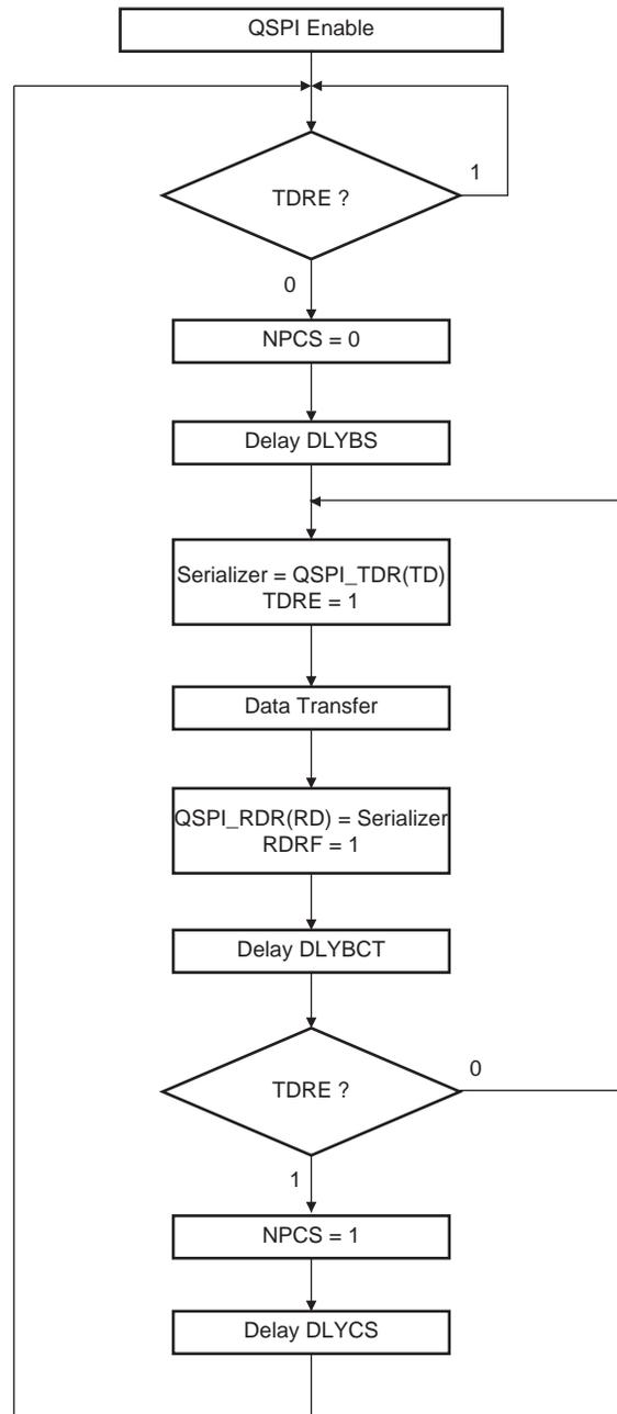
Figure 50-7 shows Transmit Data Register Empty (TDRE), Receive Data Register Full (RDRF) and Transmission Register Empty (TXEMPTY) status flags behavior within the QSPI\_SR during an 8-bit data transfer in Fixed mode, without DMA.
