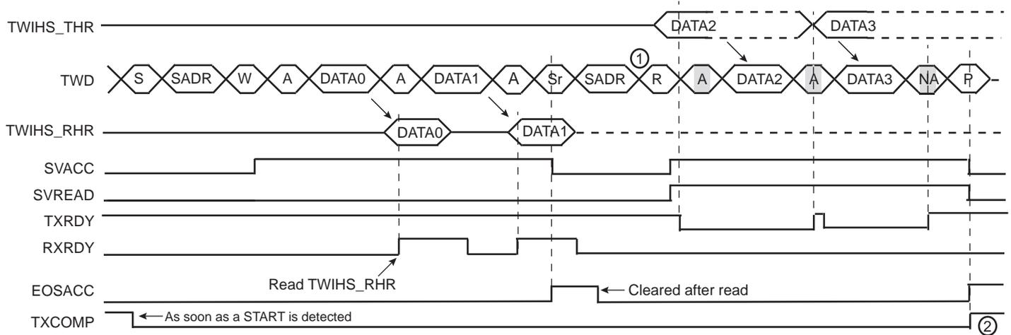
**Note 1:** In this case, if TWIHS\_THR has not been written at the end of the read command, the clock is automatically stretched before the ACK.
