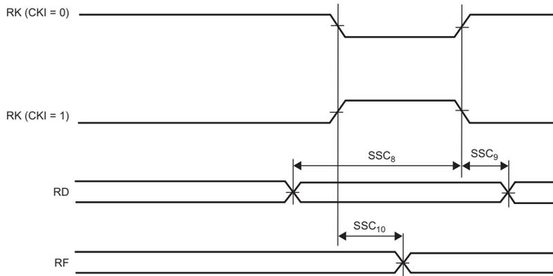
**Figure 66-36: SSC Receiver, RK and RF in Output**
