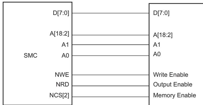
**Figure 37-5: Memory Connection for a 16-bit Data Bus**
