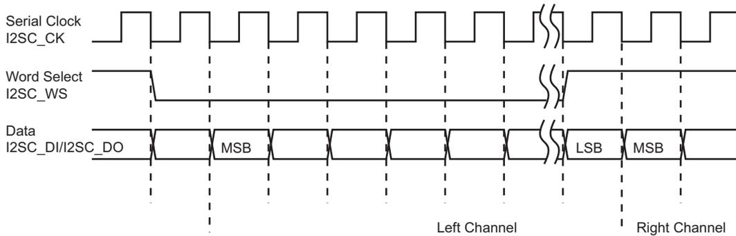
Data bits are sent on the falling edge of the serial clock and sampled on the rising edge of the serial clock. The word select line indicates the channel in transmission, a low level for the left channel and a high level for the right channel.
