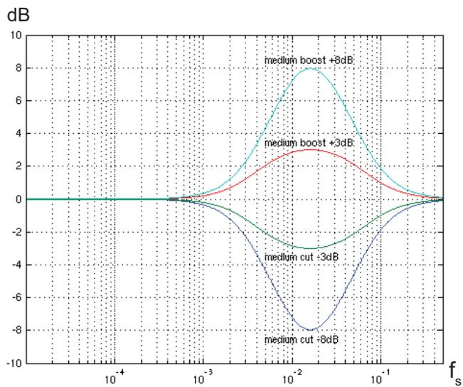
**Figure 43-7: Treble Filters Response**
