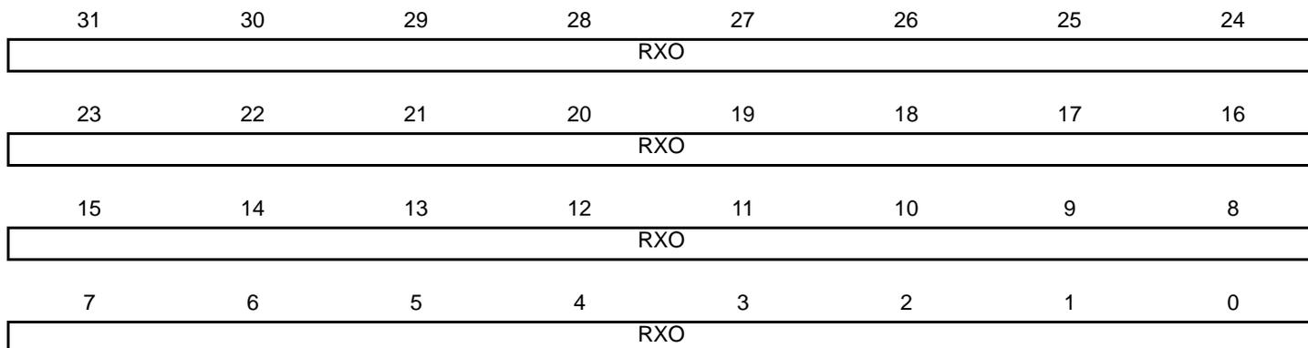
When reading the Octets Transmitted and Octets Received Registers, bits [31:0] should be read prior to bits [47:32] to ensure reliable operation.
