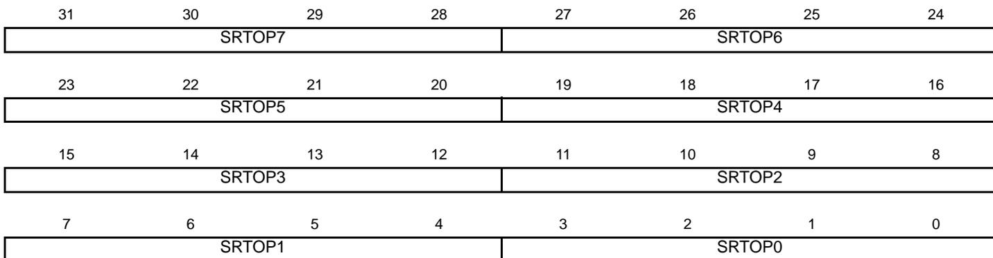
This register can only be written if the WPEN bit is cleared in the [Write Protection Mode Register](#).
