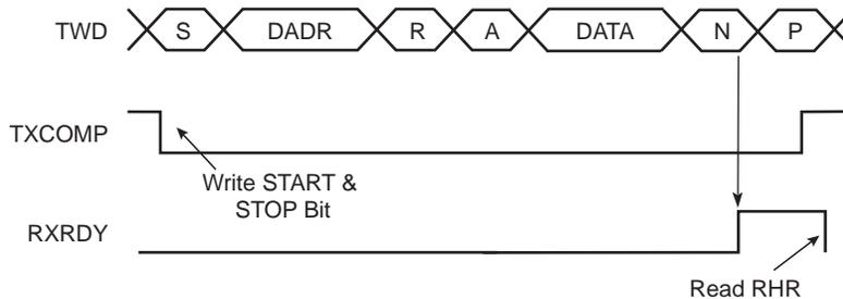
**Figure 46-8: Master Read with Multiple Data Bytes**
