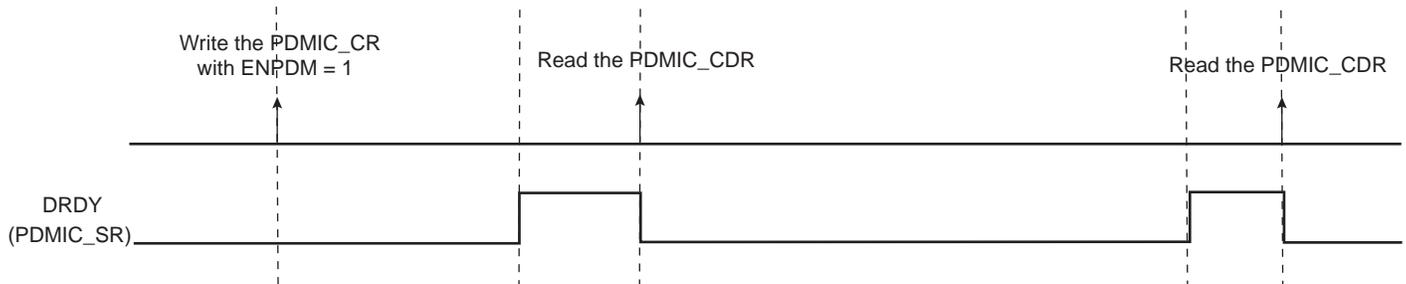
If PDMIC\_CDR is not read before further incoming data is converted, the Overrun Error (OVRE) flag is set in PDMIC\_ISR. Likewise, new data converted when DRDY is high sets the OVRE bit (Overrun Error) in PDMIC\_ISR. In case of overrun, the newly converted data is lost. The OVRE flag is automatically cleared when PDMIC\_ISR is read.
