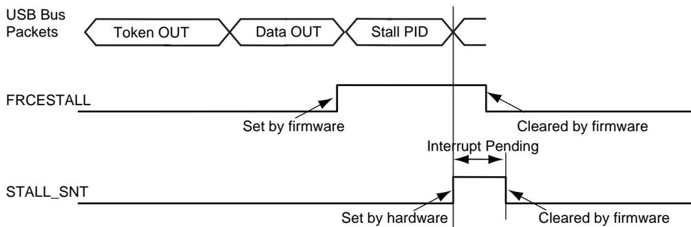
**Figure 41-18: Stall Handshake Data IN Transfer**
