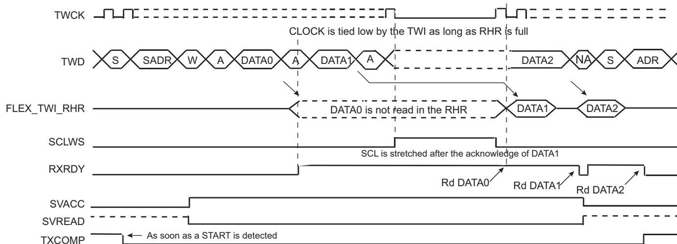
**Note 1:** At the end of the read sequence, TXCOMP is set after a STOP or after a REPEATED\_START + an address different from SADR.
