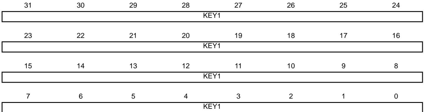
This register can only be written if the WPEN bit is cleared in the [MPDDRC Write Protection Mode Register](#).
