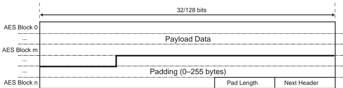
The "Pad Length" in bytes is configured in AES\_EMR.PADLEN and the "Next Header" value is configured in AES\_EMR.NHEAD. AES\_EMR.PADLEN must be configured with the length of the padding section, not including the length of the "Pad Length" and "Next Header" sections.
