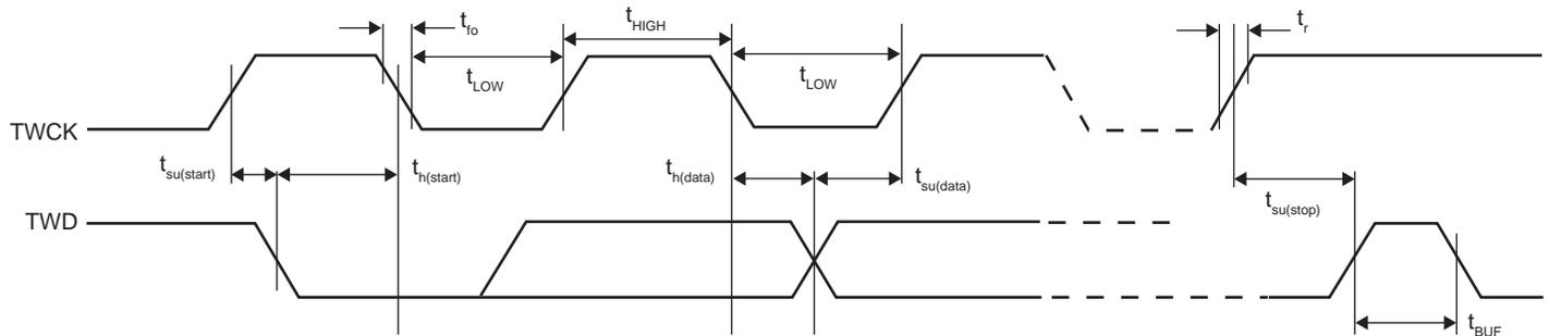
Table 66-68 describes the requirements for devices connected to the Two-wire Serial Bus.
