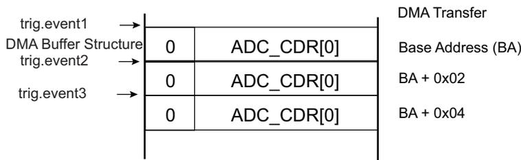
If DUALTRIG = 1 and field ADC\_TRGR.TRGMOD = 0 and none of the channels are enabled in ADC\_CHSR (ADC\_CHSR = 0), then only channel 11 is converted at a rate defined by the trigger event signal that can be configured in RTC\_MR.OUT1 (see [Figure 65-10](#)).
