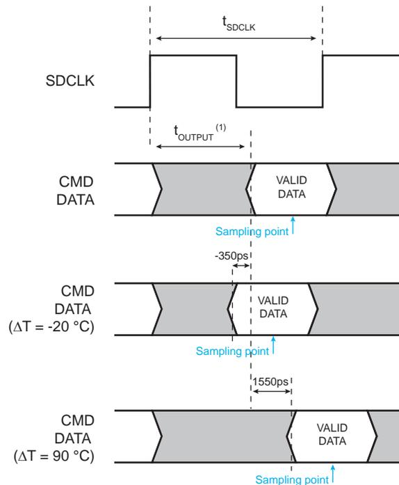
Note: 1.  $t_{OUTPUT}$  varies from 0 to  $2 \times t_{SDCLK}$
