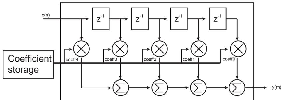
**Figure 39-8: Vertical Resampler Filter Architecture**
