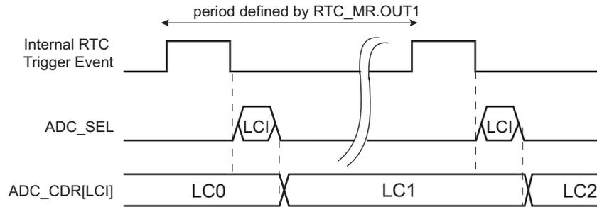
Notes: ADC\_SEL: Command to the ADC analog cell
