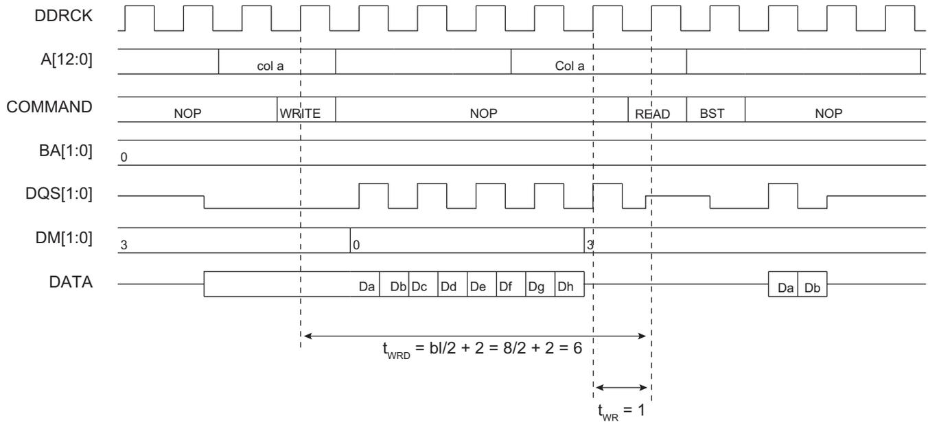
In case of a single write access, write operation should be interrupted by a read access but DM must be input 1 cycle prior to the read command to avoid writing invalid data. See [Figure 36-7](#).
