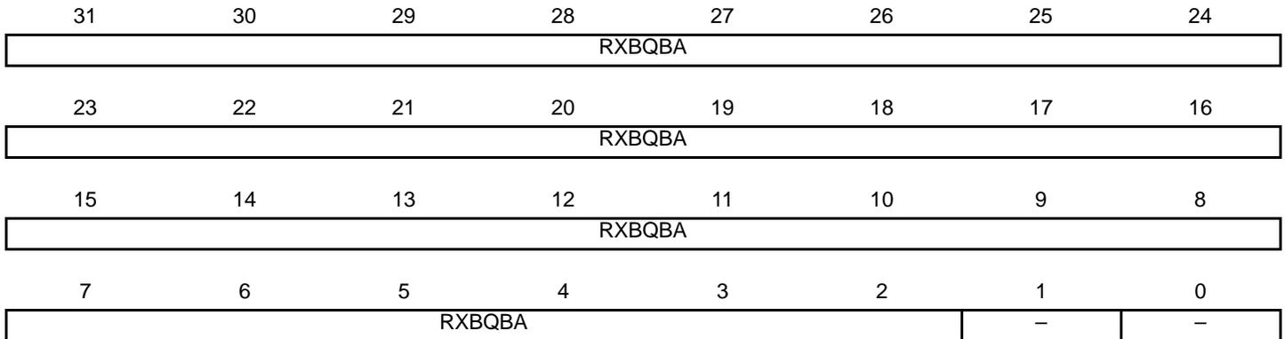
These registers hold the start address of the receive buffer queues (receive buffers descriptor lists) for the additional queues and must be initialized to the address of valid descriptors, even if the priority queues are not used.
