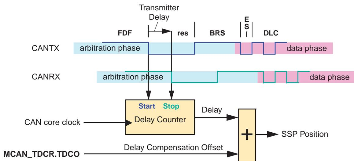
To avoid that a dominant glitch inside the received FDF bit ends the delay compensation measurement before the falling edge of the received res bit, resulting in a too early SSP position, the use of a transmitter delay compensation filter window can be enabled by programming MCAN\_TDCR.TDCF.
