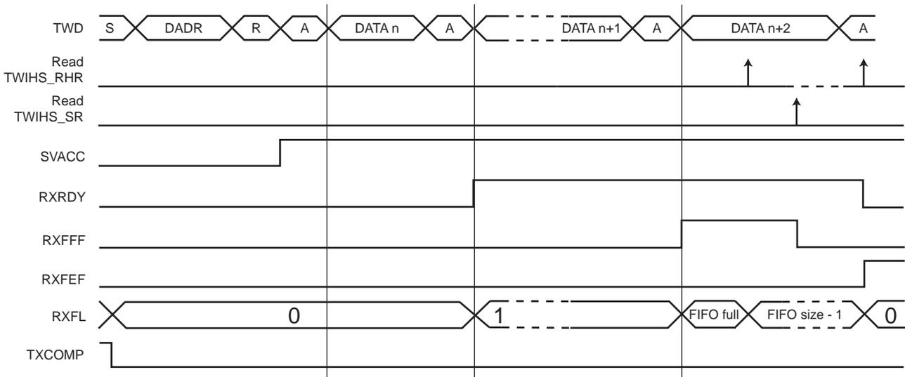
TXRDY and RXRDY behavior can be modified using the TXRDYM and RXRDYM fields in the TWIHS\_FMR. In Single Data mode, there is no need to modify the TXRDY and RXRDY behavior; however, it may be useful in Multiple Data mode.
