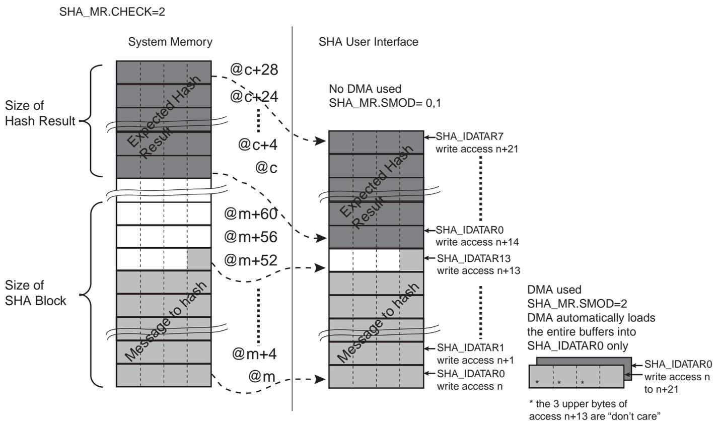
The number of 32-bit words of the hash result to check with the expected hash can be selected with SHA\_MR.CHCNT. The status of the check is available in the CHKST field in the SHA Interrupt Status register (SHA\_ISR).
