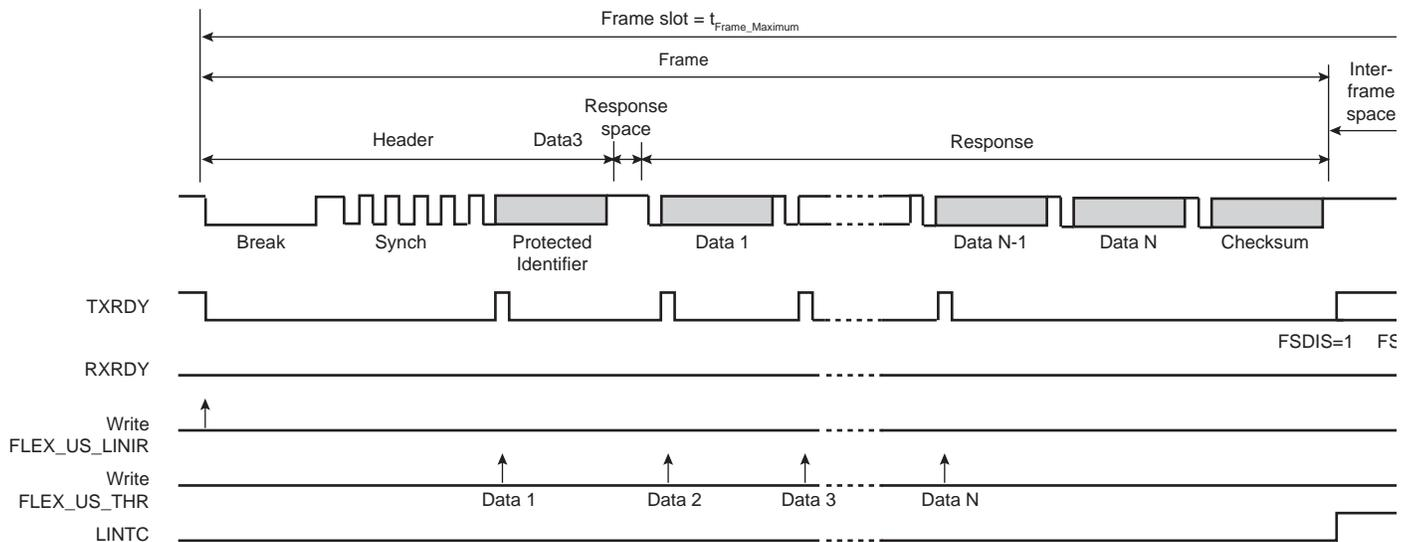
**Figure 47-48: Master Node Configuration, NACT = SUBSCRIBE**
