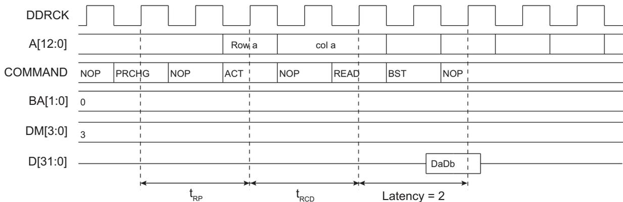
**Figure 36-10: Single Read Access, Row Closed, Latency = 3, DDR2-SDRAM Devices**
