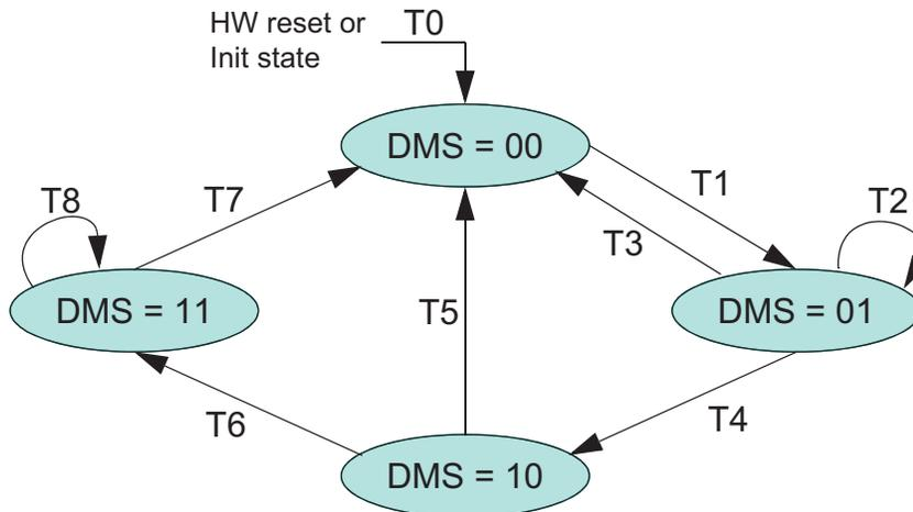
T0: reset m\_can\_dma\_req output, enable reception of debug messages A, B, and C
