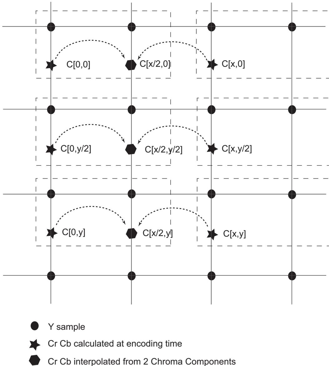
**Figure 39-3: 4:2:2 Packed Upsampling Algorithm**
