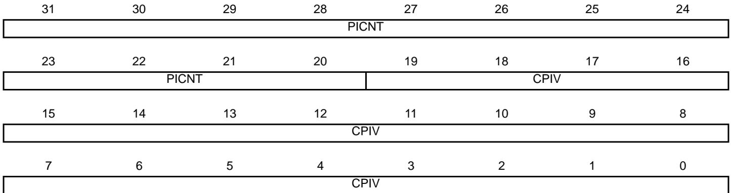
Reading this register clears PITS in PIT\_SR.
