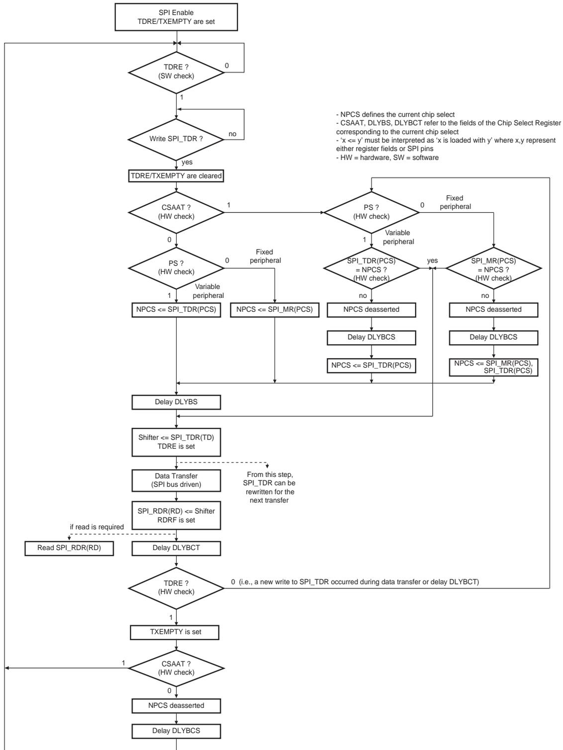
Figure 49-8 shows the behavior of Transmit Data Register Empty (TDRE), Receive Data Register (RDRF) and Transmission Register Empty (TXEMPTY) status flags within SPI\_SR during an 8-bit data transfer in Fixed mode without the DMA involved.
