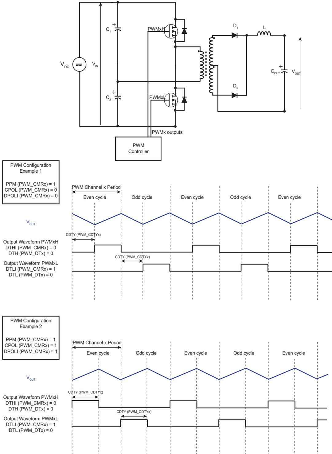
Figure 56-14: Half-Bridge Converter Application: Feedback Regulation
