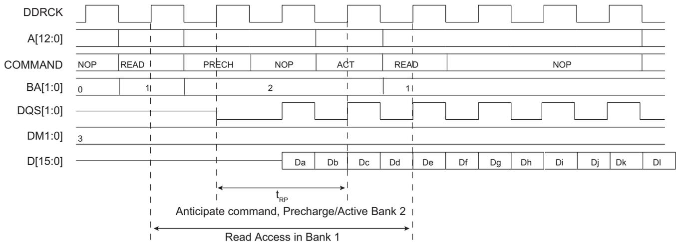
MPDDRC is a multiport controller that embeds three arbitration mechanisms based on round-robin arbitration which allows to share the external device between different masters when two or more masters try to access the DDR-SDRAM device at the same time.
