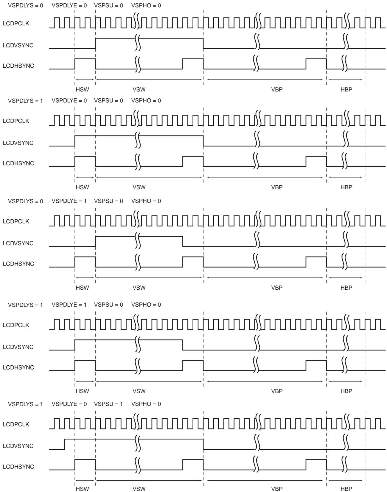
**Figure 39-16: Vertical Synchronization Timing (part 2)**
