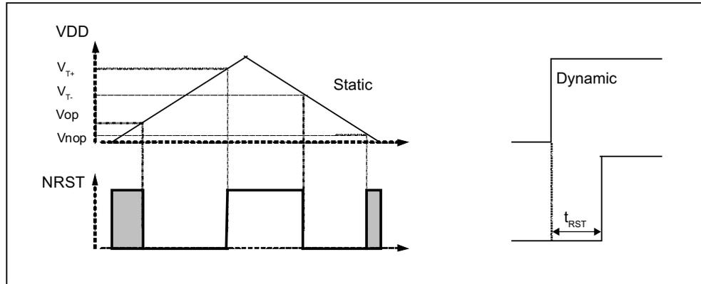
When a very slow (versus  $t_{RST}$ ) supply rising slope is applied on the POR VDD pin, the reset time becomes negligible and the reset signal is released when VDD raises higher than  $V_{T+}$ .
