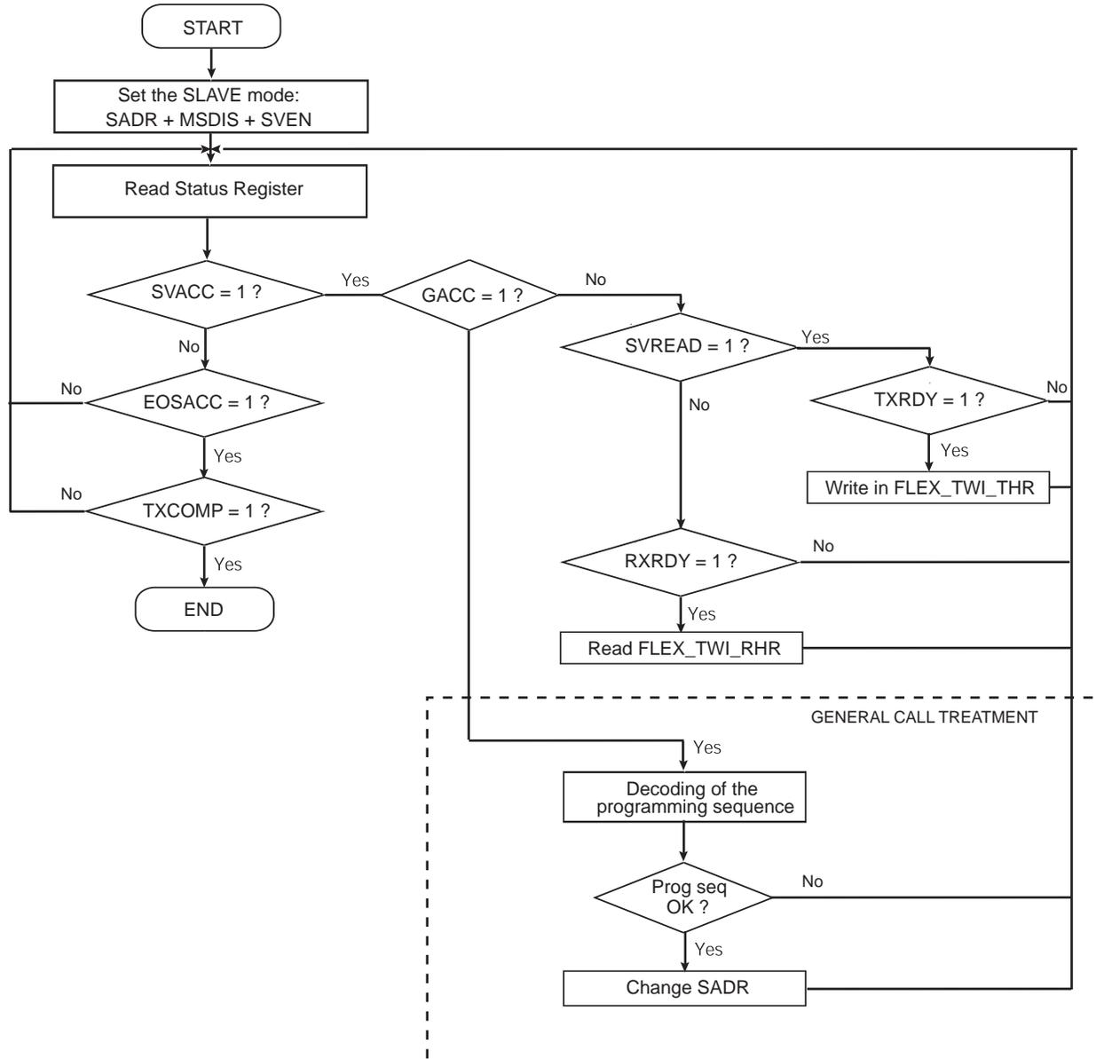
Figure 47-126: Read/Write in Slave Mode with SMBus PEC
