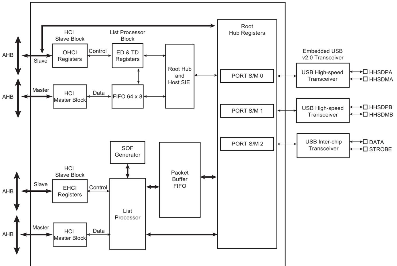
Access to the USB host operational registers is achieved through the AHB bus slave interface. The Open HCI host controller and Enhanced HCI host controller initialize master DMA transfers through the AHB bus master interface as follows:
