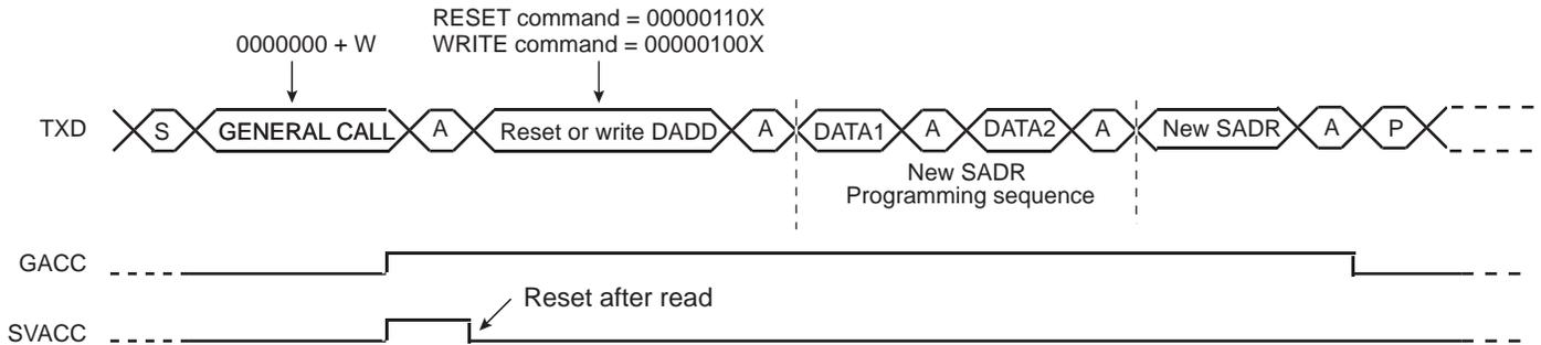
**Note:** This method allows to create a user-specific programming sequence by choosing the number of programming bytes. The programming sequence has to be provided to the master.
