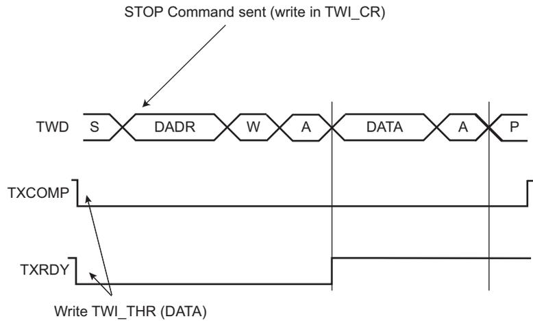
**Figure 46-5: Master Write with Multiple Data Bytes**
