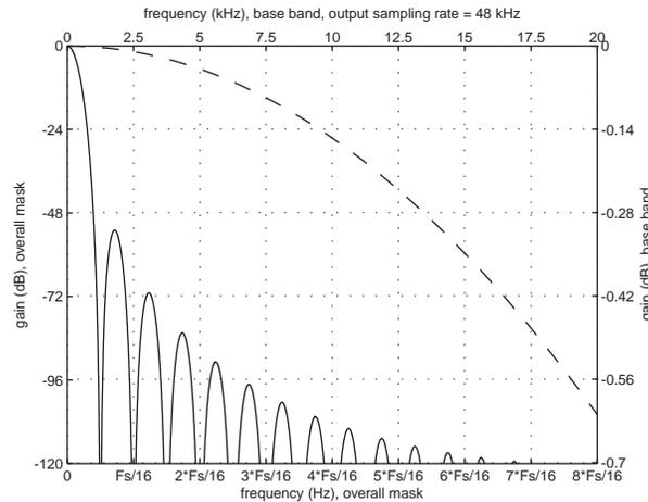
The zeros of this filter are located at multiples of  $F_s/32$ .
