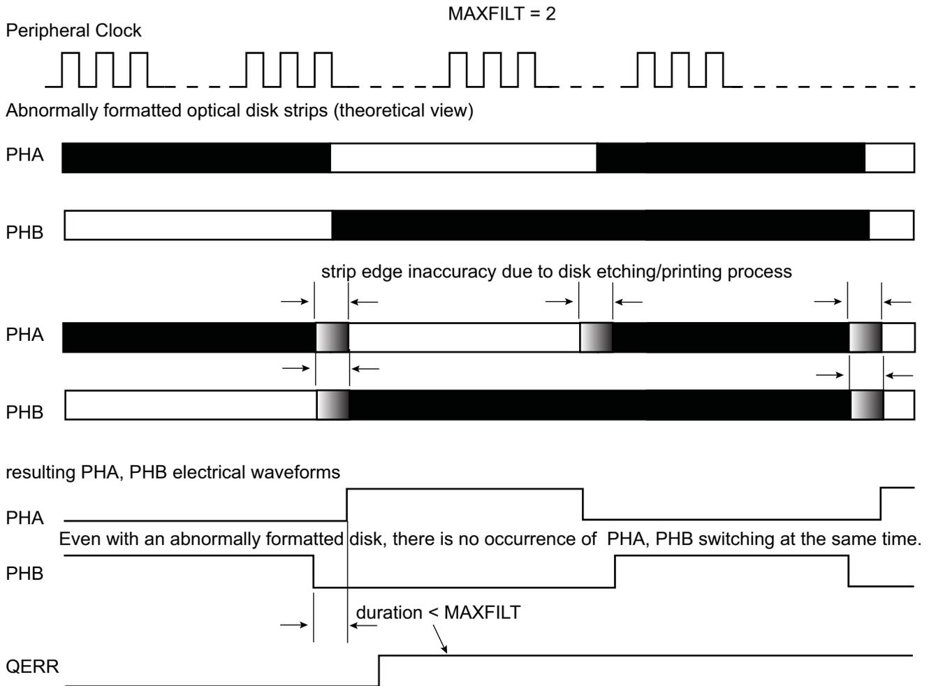
TC\_BMR.MAXFILT must be tuned according to several factors such as the peripheral clock frequency, type of rotary sensor and rotation speed to be achieved.
