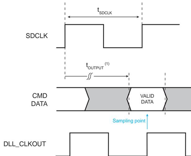
Note: 1.  $t_{OUTPUT}$  varies from 0 to  $2 \times t_{SDCLK}$
