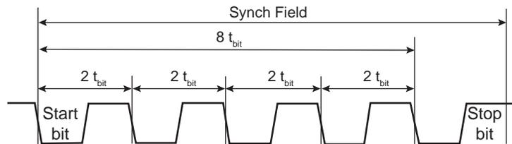
The time measurement is made by a 19-bit counter driven by the sampling clock (see [Section 47.7.1 “Baud Rate Generator”](#)).
