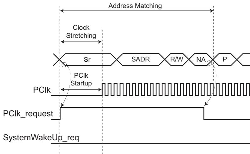
Figure 47-123: Address and Data Match (Data Matching Enabled)
