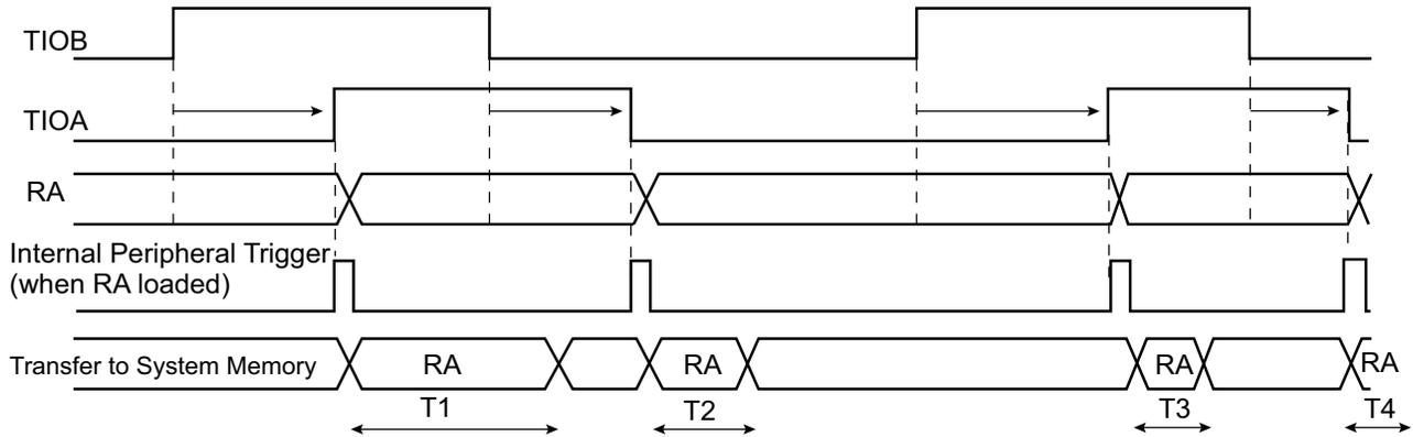
T1,T2,T3,T4 = System Bus load dependent ( $t_{\min} = 8$  Peripheral Clocks)
