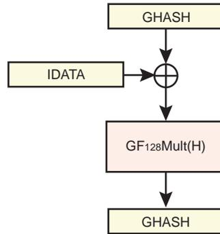
It is possible to process a message with only AAD setting the CLEN field to '0' in AES\_CLENR, this can be used for  $J_0$  generation when  $\text{len}(IV) \neq 96$  for instance.
