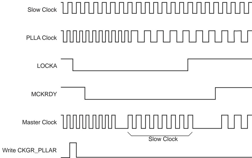
Figure 33-14: Programmable Clock Output Programming
