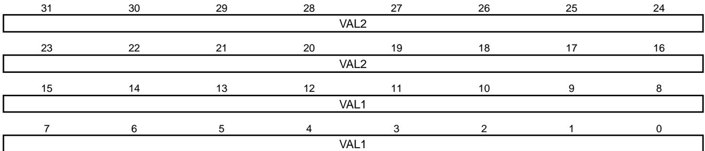
This register can only be written if the WPEN bit is cleared in the [SPI Write Protection Mode Register](#).
