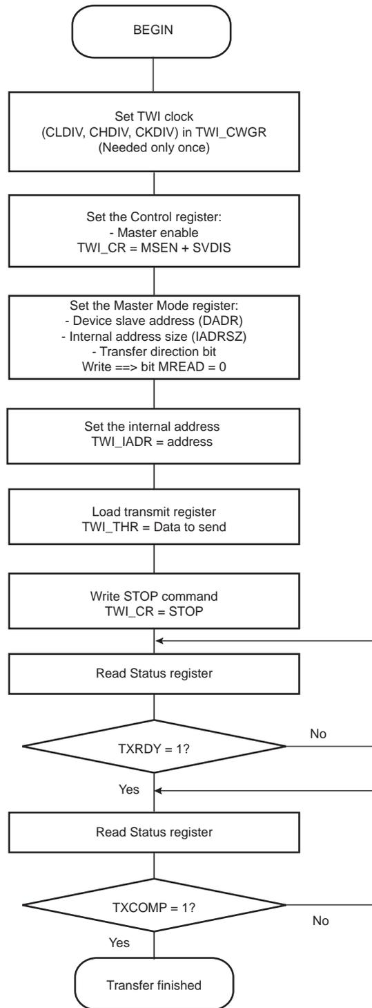
Figure 46-16: TWIHS Write Operation with Multiple Data Bytes with or without Internal Address
