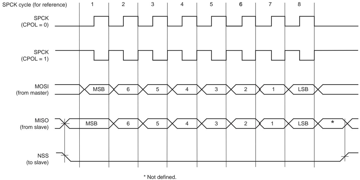
**Figure 49-4: SPI Transfer Format (NCPHA = 0, 8 bits per transfer)**
