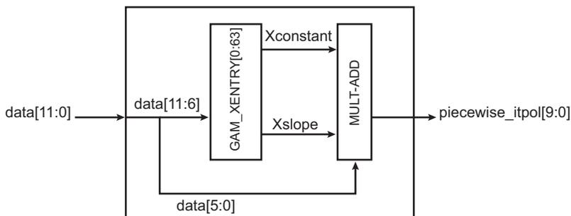
The interpolation consists of three tables that store the function values `GAM_XENTRY[0:63]` where `X` stands for `R`, `G` and `B`. The input of the table has six bits. It outputs a slope and a constant. The slope is later multiplied by the data lsb (6-bit) and added to a constant. The final value is the gamma-corrected value of the input. This module performs a 12-to-10 compression.
