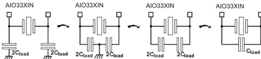
The  $C_{LOAD}$  value must be specified by the crystal manufacturer.
