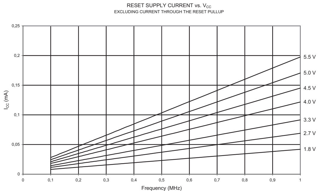
Figure 23-10. Reset Supply Current vs. V_{CC} (0.1 - 1.0 MHz, Excluding Current Through the Reset Pull-up)
