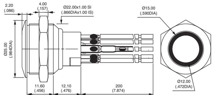
Wire colours : black: NC, orange: NO, red: LED anode (+), blue : LED cathode (-)
