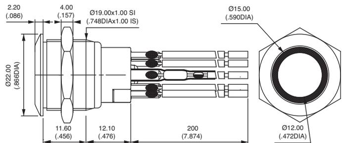
Wire colours : black: NC, orange: NO, red: LED anode (+), blue : LED cathode (-)
