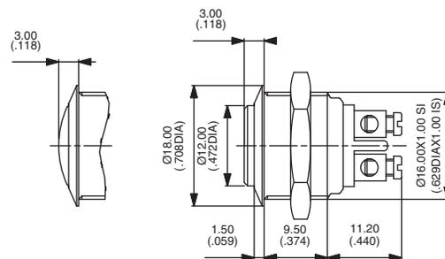
Screw terminals for wires 1,5 mm<sup>2</sup> max.
