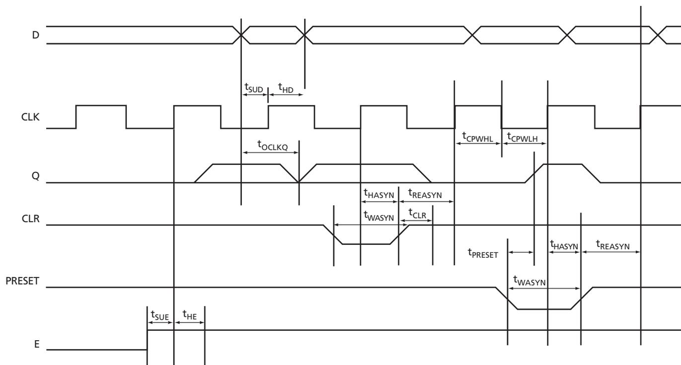
Figure 2-14 • Output Enable Register Timing Characteristics
