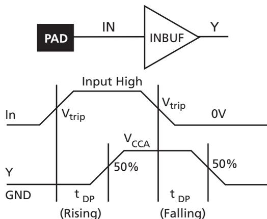
Figure 2-9 • Input Buffer Delays
