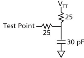
Figure 2-22 • AC Test Loads
