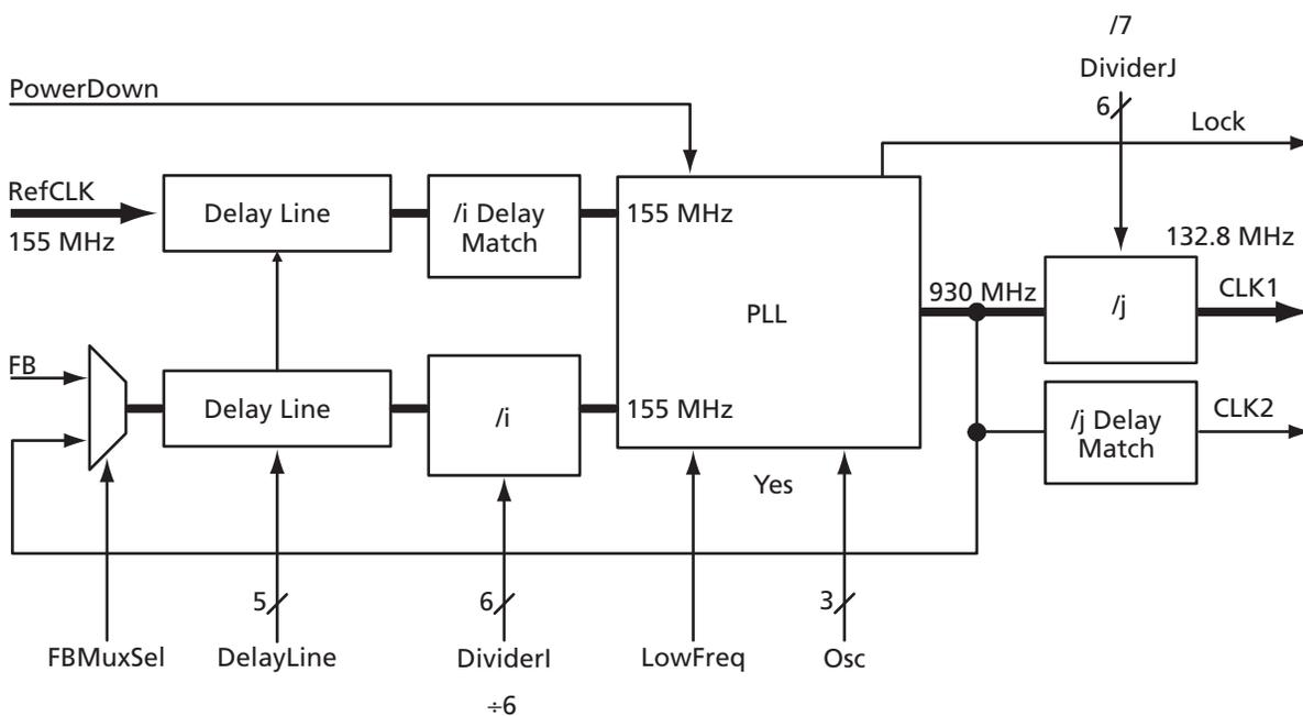
Figure 2-54 • Using the PLL 155 MHz In, 133 MHz Out
