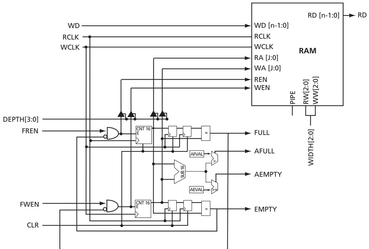
Figure 2-61 • Axcelerator RAM with Embedded FIFO Controller
