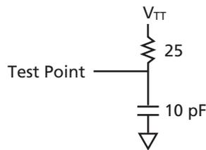
Figure 2-19 • AC Test Loads
