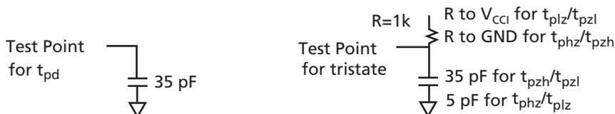
Figure 2-16 • AC Test Loads
