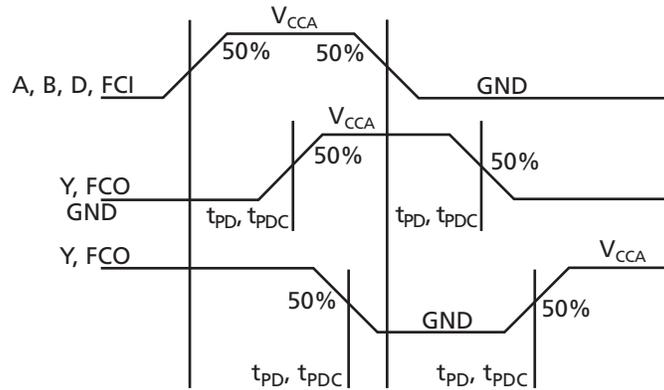
Figure 2-28 • C-Cell Timing Model and Waveforms
