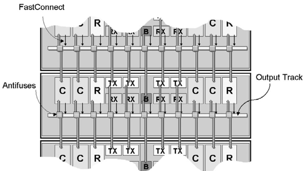
Figure 2-36 • FastConnect Routing
