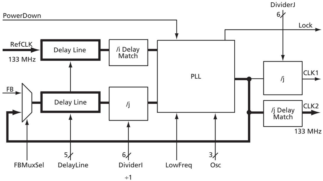
Figure 2-55 • Using the PLL Delaying the Reference Clock
