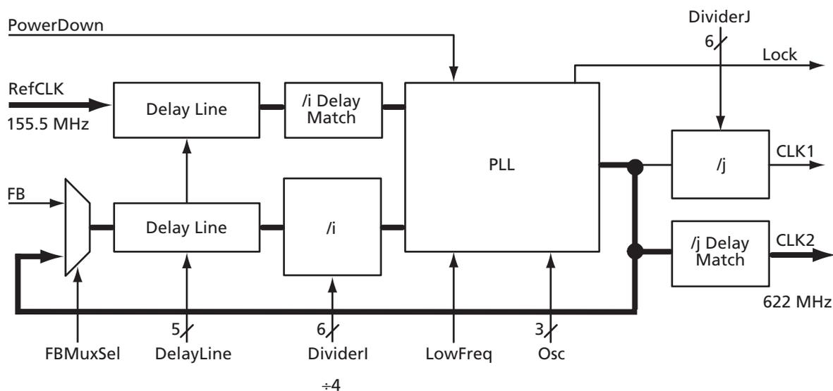
Figure 2-53 • Using the PLL 155.5 MHz In, 622 MHz Out
