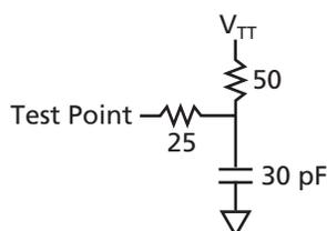
Figure 2-23 • AC Test Loads
