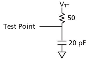
Figure 2-20 • AC Test Loads
