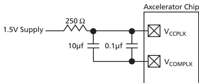
Figure 2-2 • V<sub>CCPLX</sub> and V<sub>COMPLX</sub> Power Supply Connect
