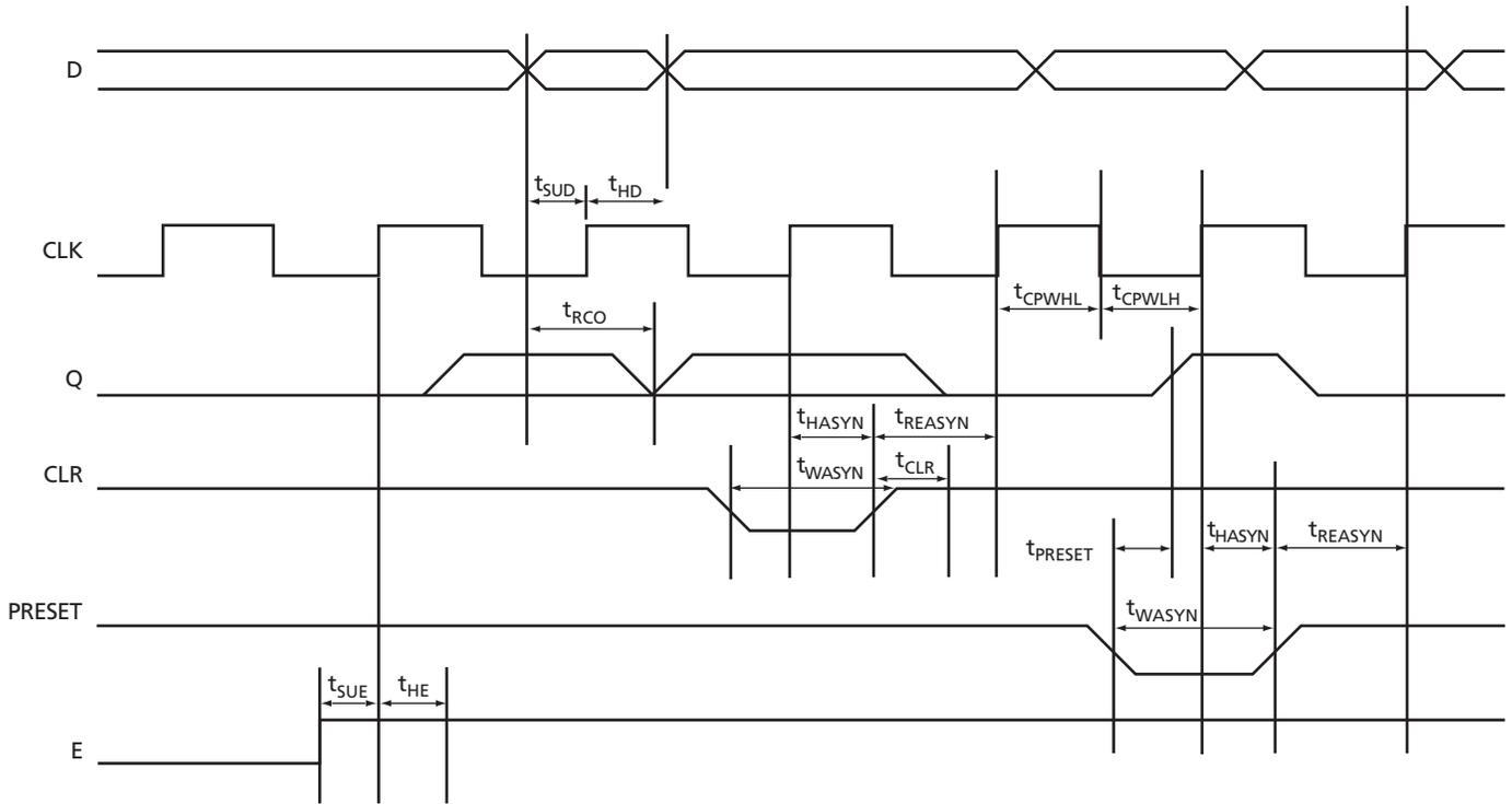
Figure 2-32 • R-Cell Delays
