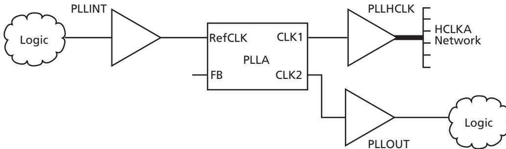
Figure 2-46 • Example of PLLINT and PLLOUT Usage
