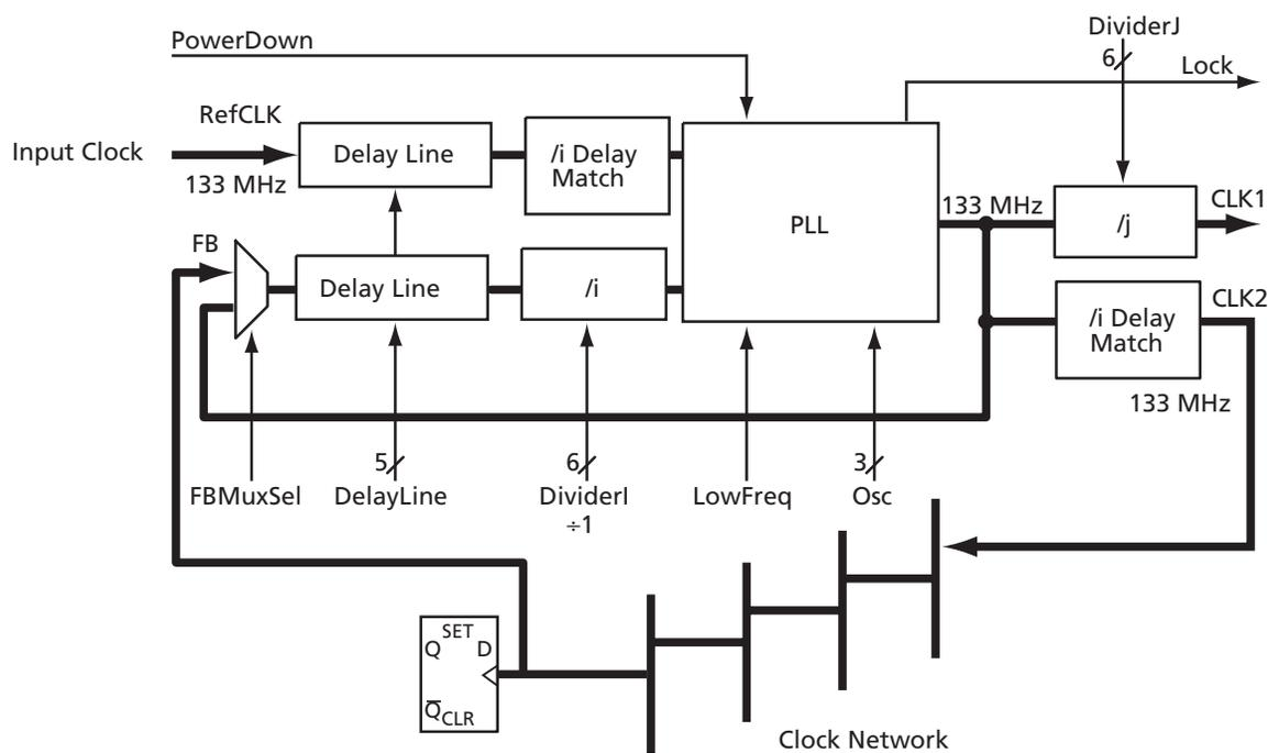
Figure 2-56 • Using the PLL for Clock Deskewing
