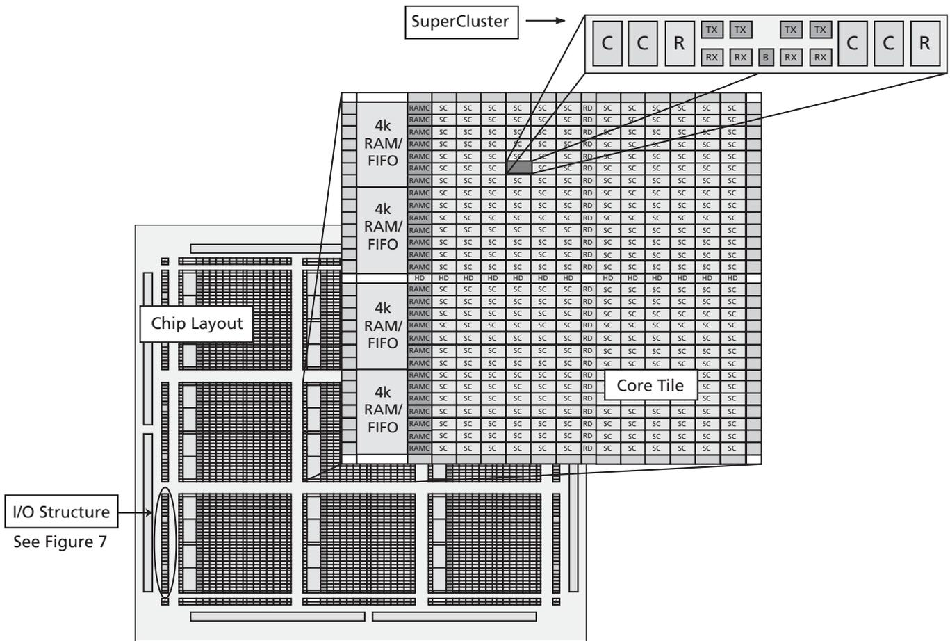
Figure 1-6 • AX Device Architecture (AX1000 shown)
