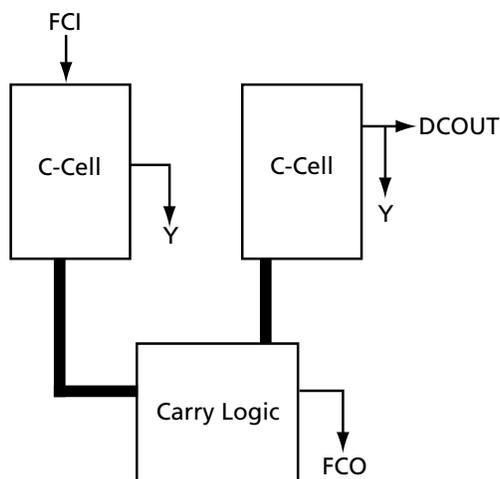
Figure 1-5 • AX 2-bit Carry Logic
