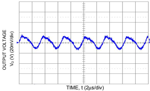
Figure 10. Typical Output Ripple and Noise
