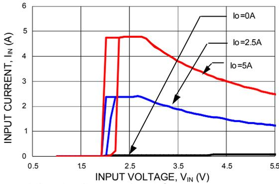
Figure 8. Input voltage vs. Input Current
