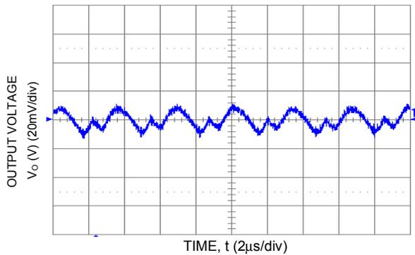
Figure 9. Typical Output Ripple and Noise
