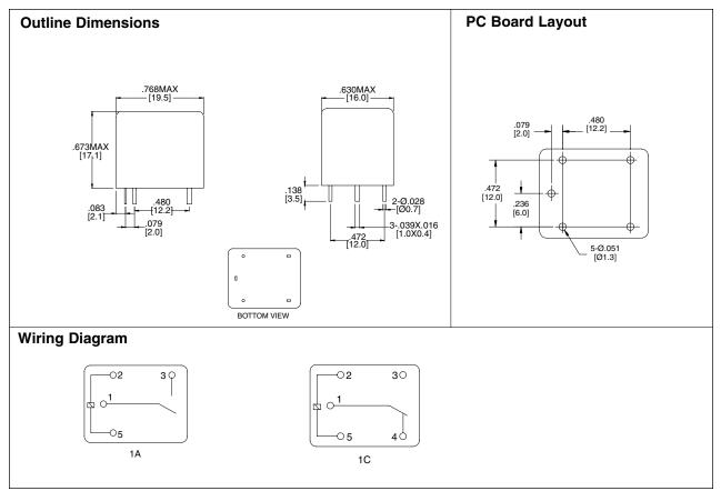
Dimensions in inches with metric equivalents in parentheses. Tolerance: ±0.010"
