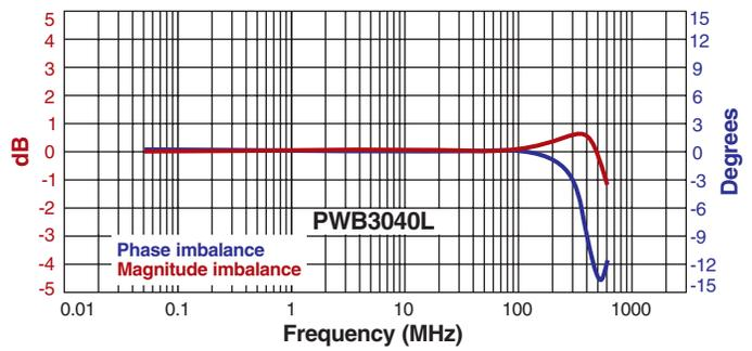
Measured on a network analyzer (re: 50 Ohms)
