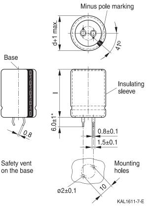
$0.8^{+0.2}_{-0.1}$ 1.5±0.2 Safety vent on the base Mounting holes ø2±0.1 ø2.5 min. KAL1612-F-E Snap-in terminals, length (6.0 ±1) mm. Snap-in capacitors are also available with 3 terminals (length (4.5 - 1) mm).
