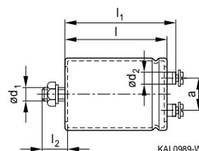
For B43330 capacitors with threaded stud and  $d \leq 76.9$  mm the base is not insulated. For details, refer to "Data Book 2007 – Aluminum Electrolytic Capacitors",
