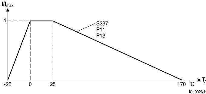
$$\text{Percent of } I_{\max} = 100 \left[ 1 - \frac{T_A - 25 \text{ }^\circ\text{C}}{T_{\max} - 25 \text{ }^\circ\text{C}} \right]$$
