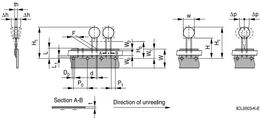
**Lead spacing  $F = 7.5 \text{ mm}$**  (taping based on IEC 60286-2)
