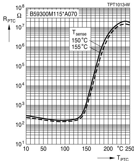
**Sensors****Motor protection, triple sensors****M1300****Characteristics (typical)**
