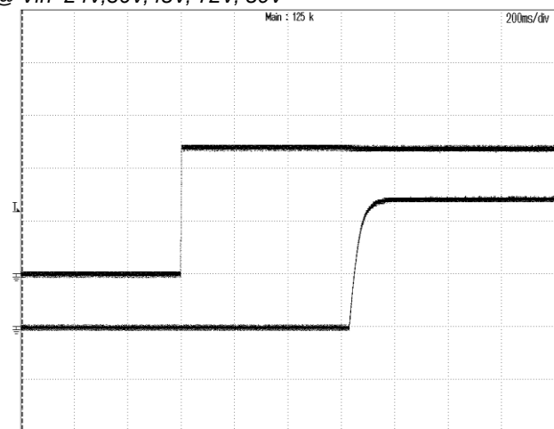
Figure 4: Vout start up with Vin on at 48Vin, 24A Iout, TOP: VIN, 20V/div, 200mS/div BOTTOM: VOUT, 5V/div, 200mS/div
