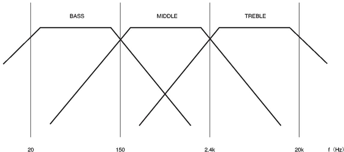
The input signal is separated into three regions : bass (20Hz to 150Hz), middle (150Hz to 2.4kHz) and treble (2.4kHz to 20kHz). These regions are then joined again with the middle and treble regions phase shifted  $-180^\circ$  and  $-360^\circ$  respectively with respect to the bass signal. This phase shift adjusts the delay time characteristic for
