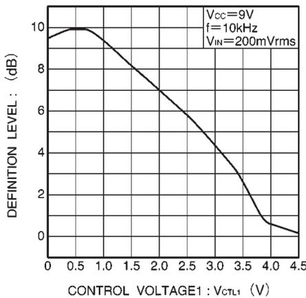
Fig. 3 Definition level vs. control voltage 1
