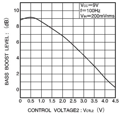
Fig. 5 Bass boost level vs. control voltage 2
