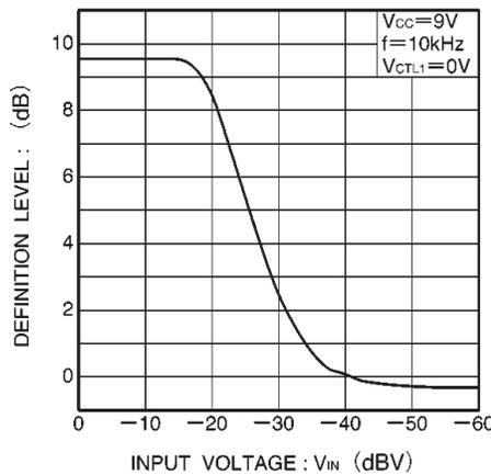
Fig. 4 Definition level vs. input voltage 1
