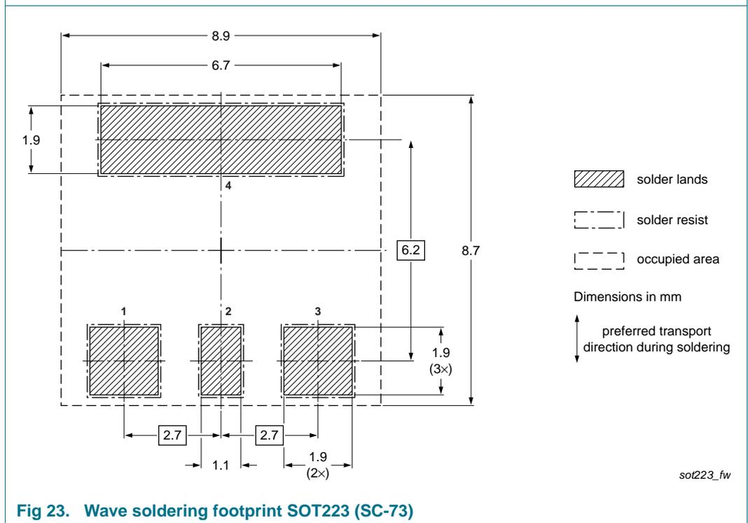
**Fig 23. Wave soldering footprint SOT223 (SC-73)**
