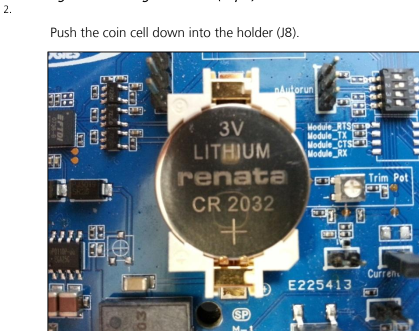
Figure 15: Inserting the coin cell (step 2)
