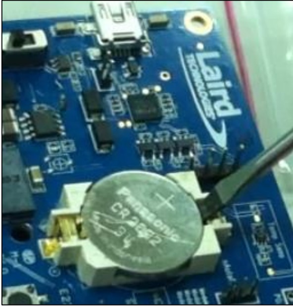
Figure 16: Removing the coin cell (step 2)
