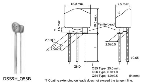
\*1 Coating extending on leads does not exceed the tangent line. Exposed electrode, if any, is covered by solder, etc.
