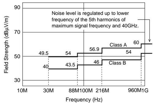
On the border frequency, lower limit should be applied.
