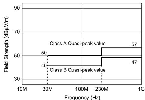
On the border frequency, lower limit should be applied.
