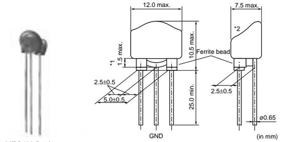
\*1 Coating extending on leads does not exceed the tangent line. Exposed electrode, if any, is covered by solder, etc.
