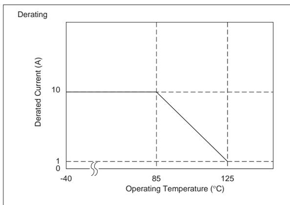
In operating temperatures exceeding +85°C, derating of current is necessary for BNX023 series. Please apply the derating curve shown in chart according to the operating temperature.
