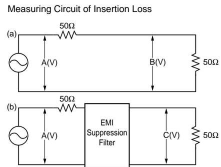
$$\text{Insertion Loss} = 20 \log \frac{B}{C} (\text{dB})$$
