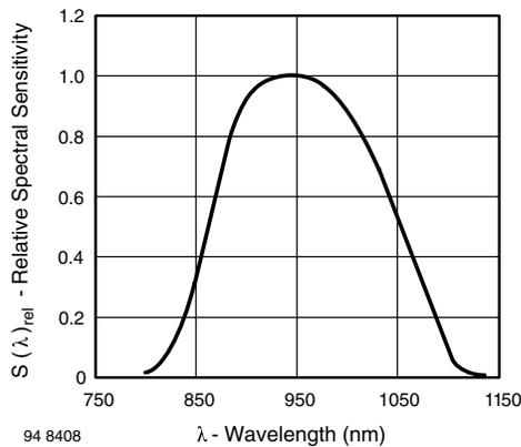
Fig. 5 - Relative Spectral Sensitivity vs. Wavelength
