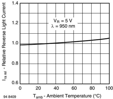
Fig. 1 - Relative Reverse Light Current vs. Ambient Temperature
