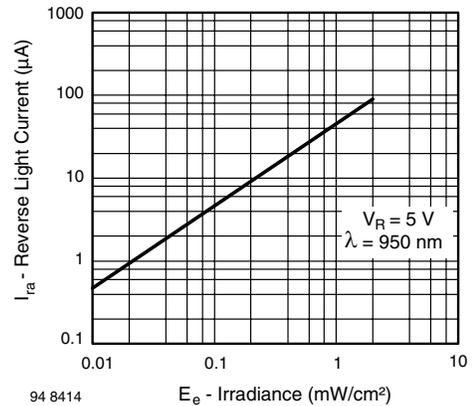
Fig. 2 - Reverse Light Current vs. Irradiance
