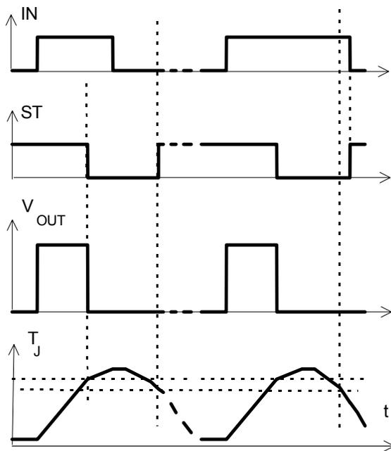
\*) ST goes high, when  $V_{IN}$ =low and  $T_j < T_{jt}$
