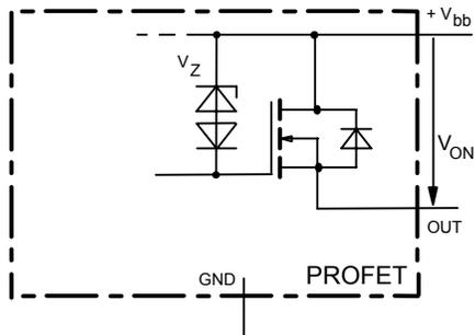
$V_{ON}$  clamped to 68 V typ.
