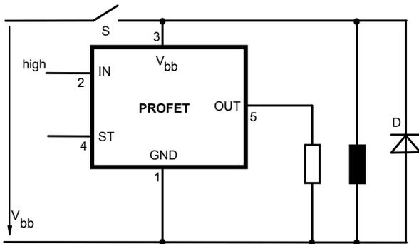
If other external inductive loads  $L$  are connected to the PROFET, additional elements like  $D$  are necessary.
