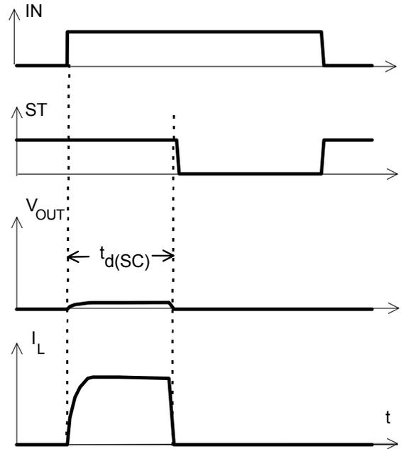
$t_{d(SC)}$  approx. --  $\mu$ s if  $V_{bb} - V_{OUT} > 8.5$  V typ.
