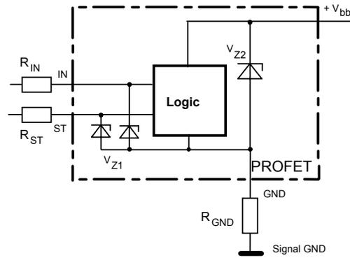
$V_{Z1} = 6.2 \text{ V typ.}, V_{Z2} = 70 \text{ V typ.}, R_{GND} = 150 \Omega, R_{IN}, R_{ST} = 15 \text{ k}\Omega$
