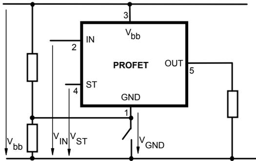
Any kind of load. If  $V_{GND} > V_{IN} - V_{IN(T+)}$  device stays off
