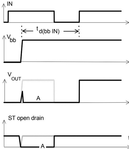
in case of too early  $V_{IN}$ =high the device may not turn on (curve A)
