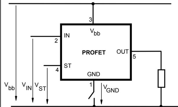
Any kind of load. In case of Input=high is  $V_{OUT} \approx V_{IN} - V_{IN(T+)}$ .
