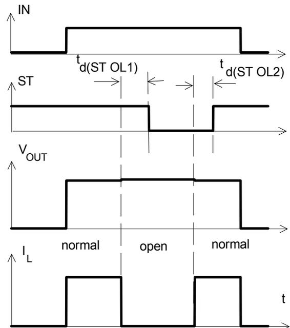
$t_{d(ST OL1)} = t_{bd} \mu$ s typ.,  $t_{d(ST OL2)} = t_{bd} \mu$ s typ
