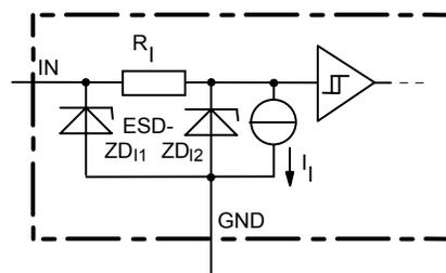
ZD11 6 V typ., ESD zener diodes are not to be used as voltage clamp at DC conditions. Operation in this mode may result in a drift of the zener voltage (increase of up to 1 V).
