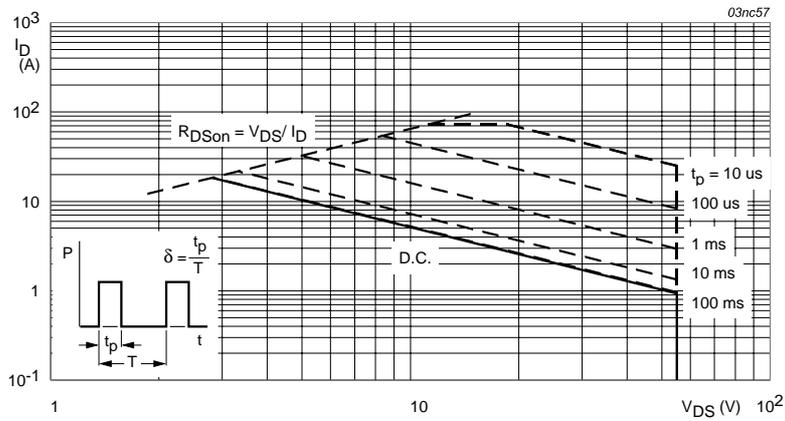
T<sub>mb</sub> = 25 °C; I<sub>DM</sub> is single pulse.
