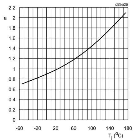
$$a = \frac{R_{DSon}}{R_{DSon(25^{\circ}C)}}$$
