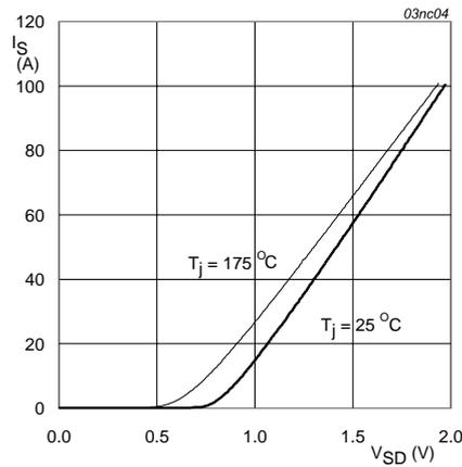
$V_{GS} = 0 \text{ V}$
