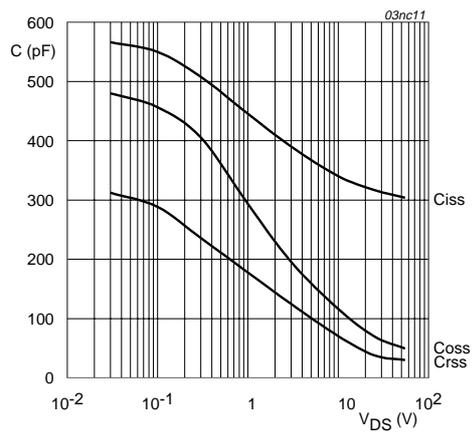
$V_{GS} = 0 \text{ V}; f = 1 \text{ MHz}$
